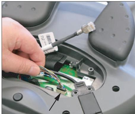
3. Press the plug connector firmly into the power supply socket.
