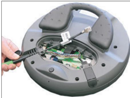
2. Insert the connecting cable in the appropriate entry (left or right).
