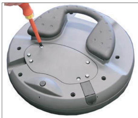
1. Open the cover by unscrewing the six PT screws (4 x 20 mm) approximately 1 cm. To do this, use a Phillips size 2 screwdriver.
