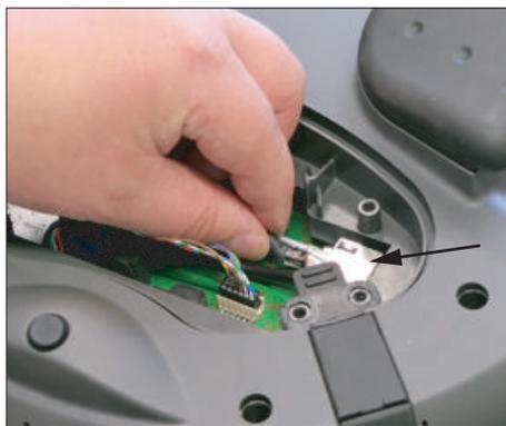
4. Connect the RJ-45 connector to the Ethernet socket.
