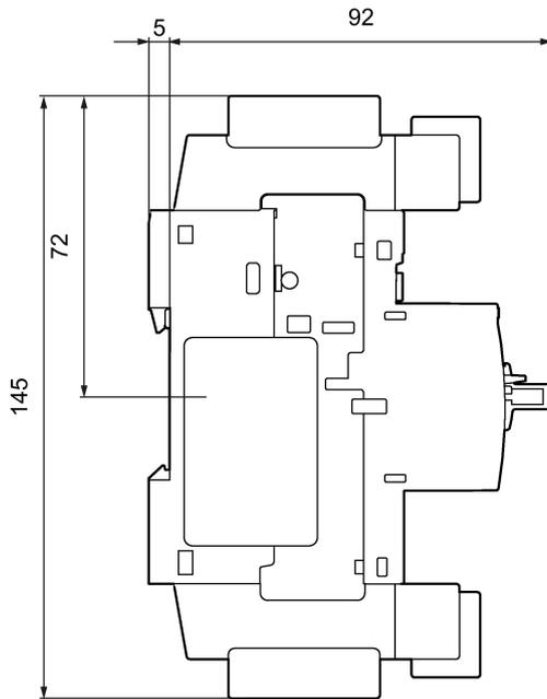
Figure C-10 Circuit breaker acc. to UL 489
