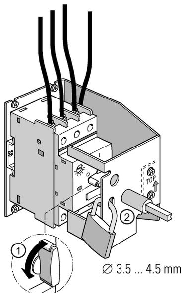
The mechanism can be locked inside the control cabinet with a padlock. The motor starter protector must be set to the O position first, before the lock is attached.
