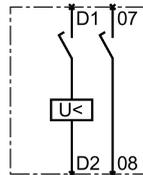
Undervoltage release with leading Shunt release
