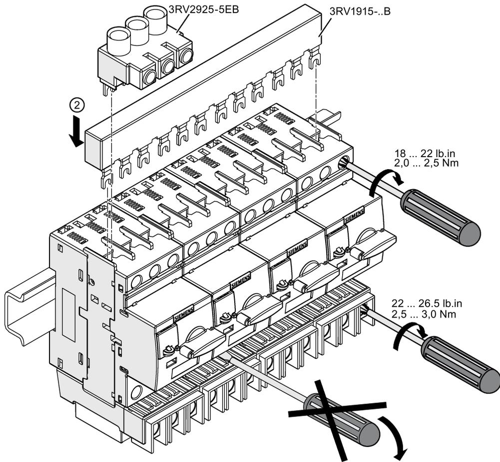
Figure 10-7 Installation with 3-phase busbars (3RV2711 / 3RV2721 / 3RV2811 / 3RV2821 size S00 / S0)
