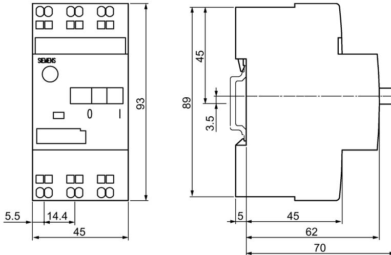
Figure C-2 Motor starter protector with spring-loaded connection system S00
