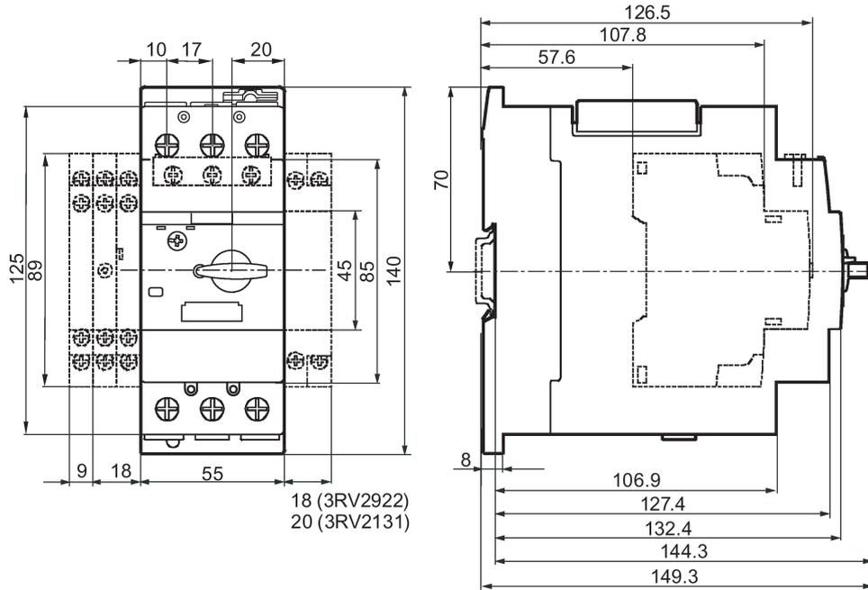
Figure C-12 3RV2.31 motor starter protector ( $\leq 45$  A)
