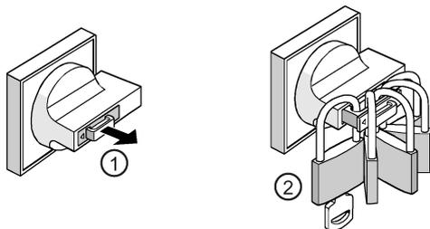
The mechanism can also be locked outside the control cabinet via the handle.
