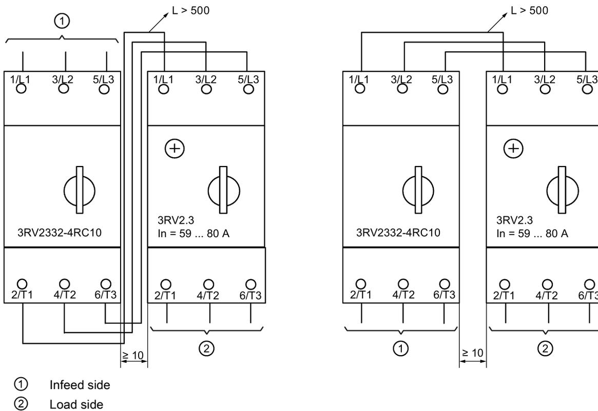
**Installation guidelines for 3RV2 motor starter protectors with limiter function (size S3)**
