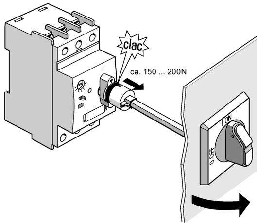
The extension shaft then needs to be re-attached to the motor starter protector and the door-coupling rotary operating mechanism as described below:
