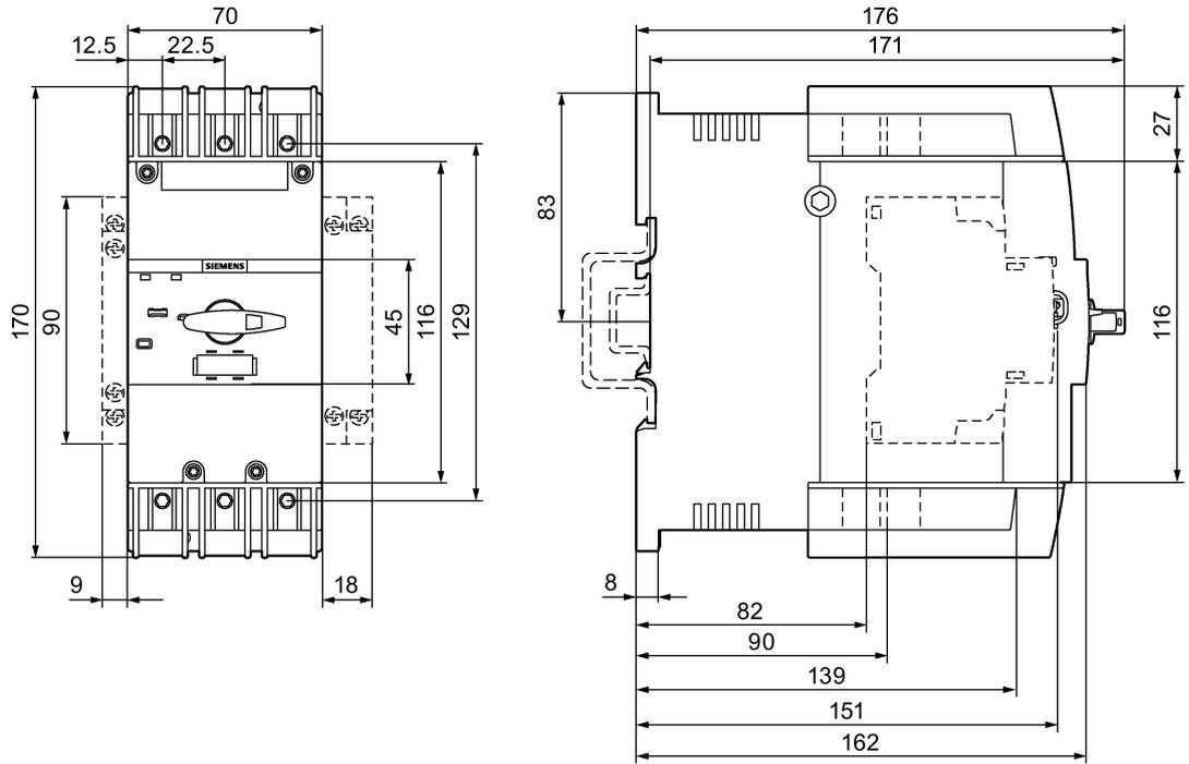
Figure C-16 Circuit breaker acc. to UL 489
