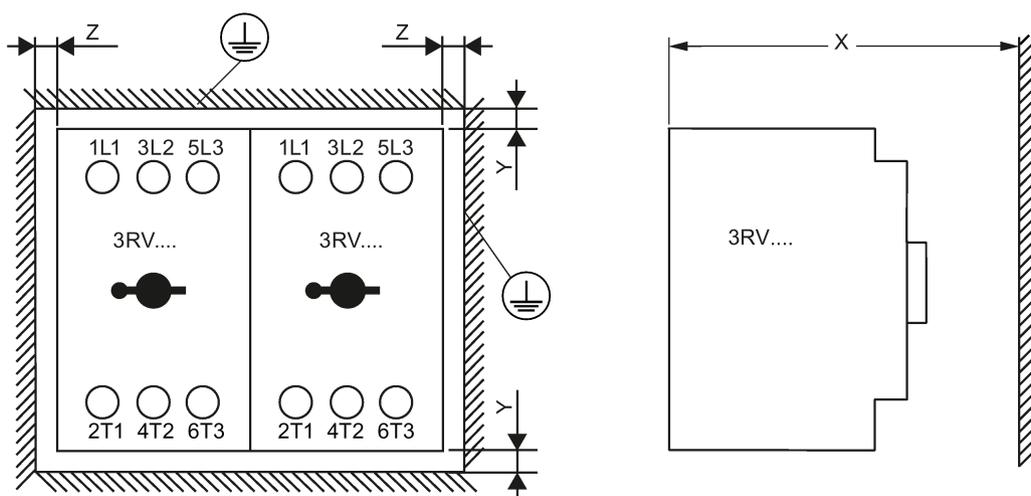
Figure 7-1 Clearances from grounded or live parts
