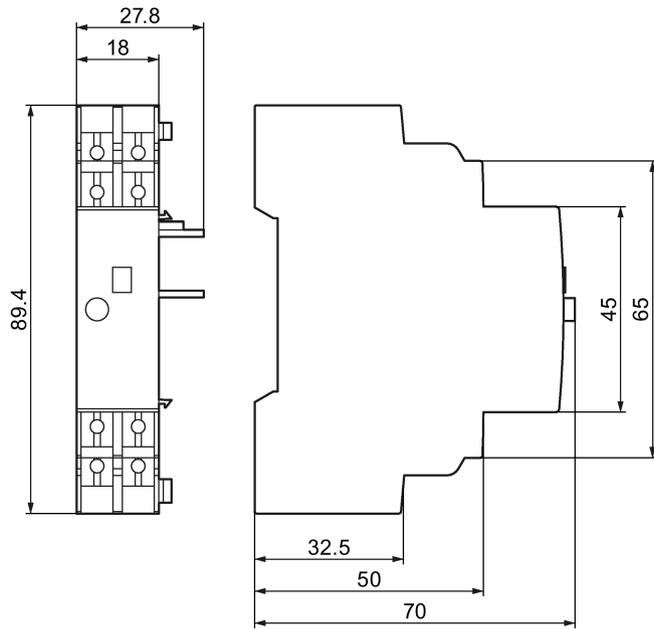
Figure C-43 3RV2921-4M signaling switch (ring cable lug connection)
