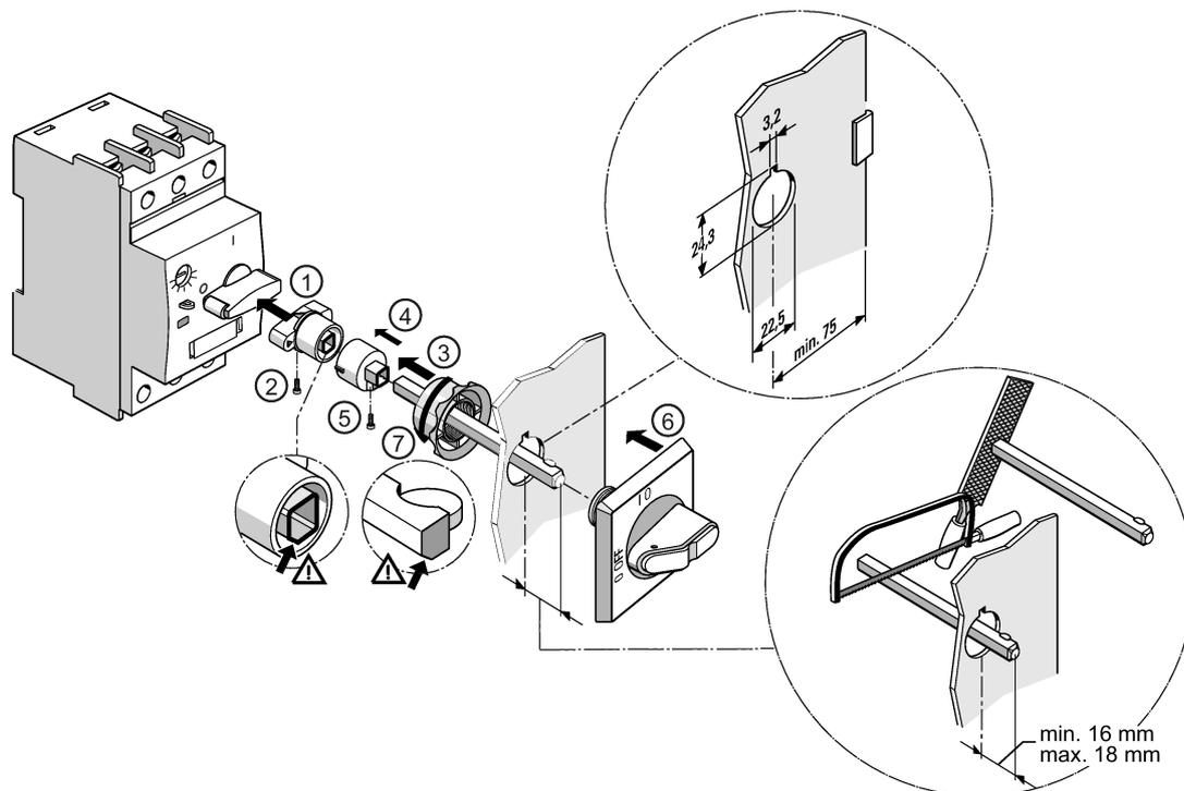
Figure 10-3 Mounting the door-coupling rotary operating mechanism
