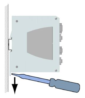
Figure 9: Removal from the DIN rail
