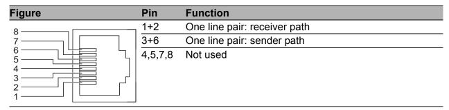
Table 2: Pin assignment of a TP/TX interface in MDI-X mode, RJ45 socket
