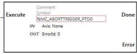
**NOTE:** When you first enter the function block, you must configure it to use the intended axis. Double-click on the function block to display the function block properties, choose the axis and click `Apply`.
