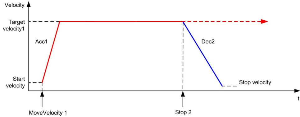
The diagram illustrates a simple profile from **Discrete** state:
