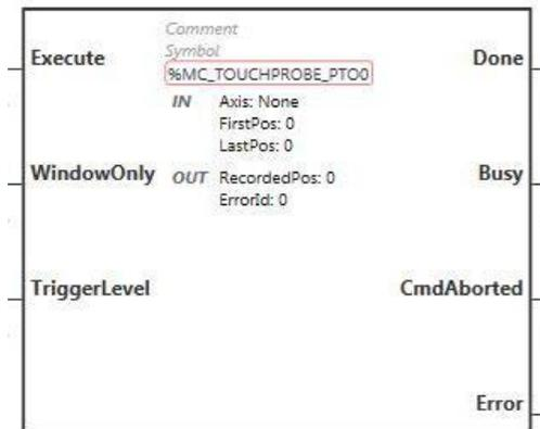
**NOTE:** When you first enter the function block, you must configure it to use the intended axis. Double-click on the function block to display the function block properties, choose the axis and click `Apply`.
