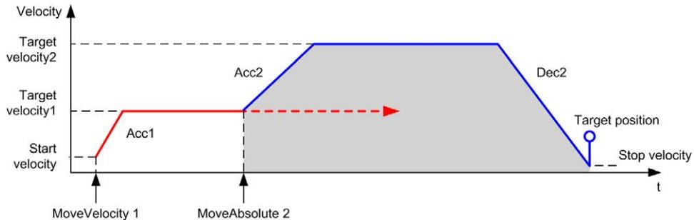
The diagram illustrates a complex profile from **Discrete** state:
