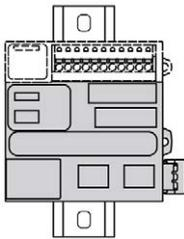
**NOTE:** Expansion modules must be mounted above the controller.
