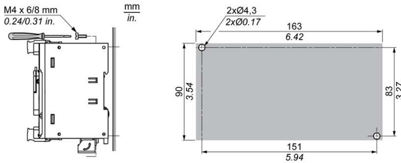
The following diagram shows the mounting hole layout for TM221M Logic Controller:
