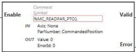
**NOTE:** When you first enter the function block, you must configure it to use the intended axis. Double-click on the function block to display the function block properties, choose the axis and click `Apply`.
