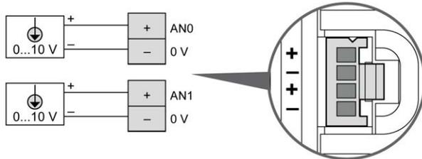
The (-) poles are connected internally.
