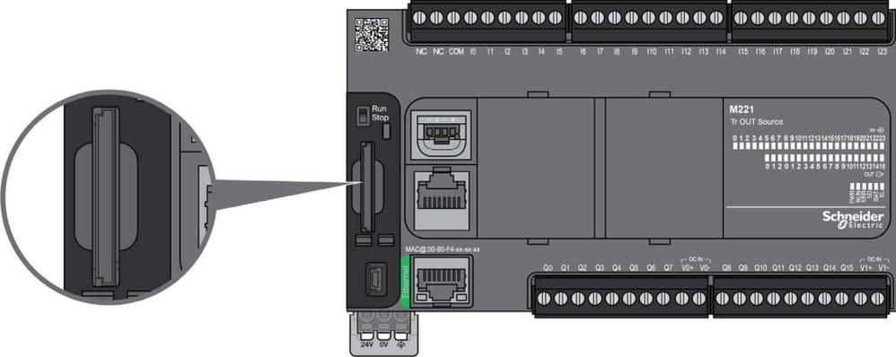
The following figure shows the SD card slot of the TM221M Logic Controller:
