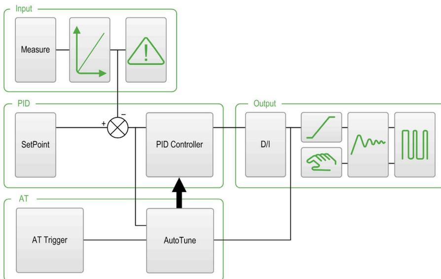
The graphical assistant helps you to visualize how the PID function is built. This is a dynamic graphic that is updated according to the configuration.
