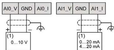
(1): Current/Voltage analog output device
