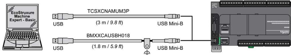
The following illustration shows the USB connection to a PC on a TM221M Logic Controller:
