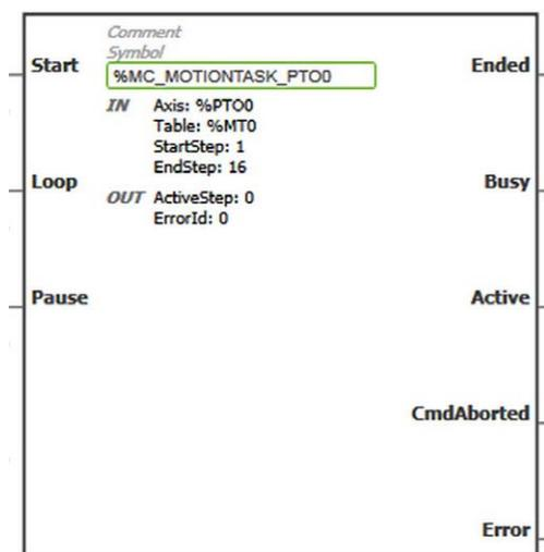
**NOTE:** When you first enter the function block, you must configure it to use the intended axis and motion task table. Double-click the function block to display the function block properties, choose the axis and table, then click `Apply`.
