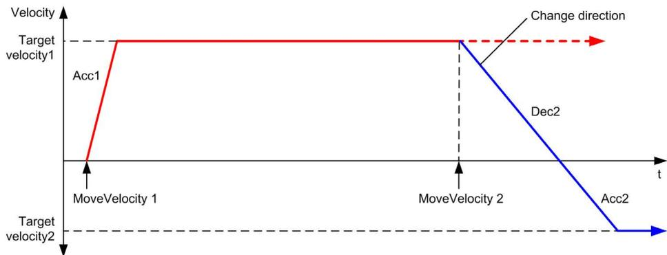
The diagram illustrates a complex profile from **Discrete** state:
