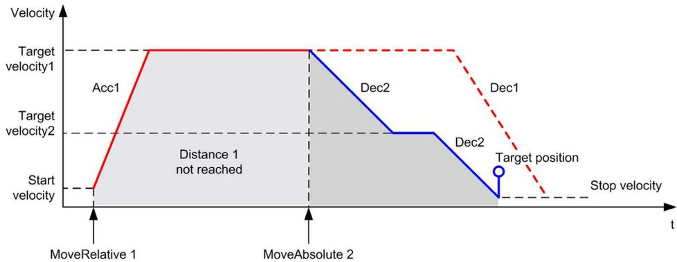
The diagram illustrates a complex profile from **Discrete** state with change of direction:
