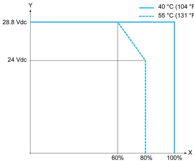
**X** Output simultaneous ON ratio
