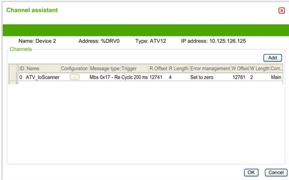
Preconfigured channels are displayed with a lock symbol
