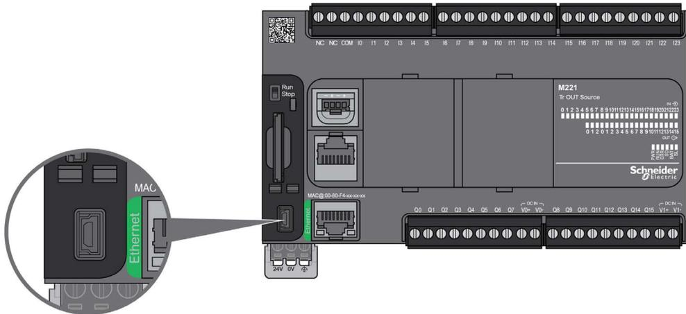
The following figure shows the location of the USB Mini-B programming port on the TM221M Logic Controller:
