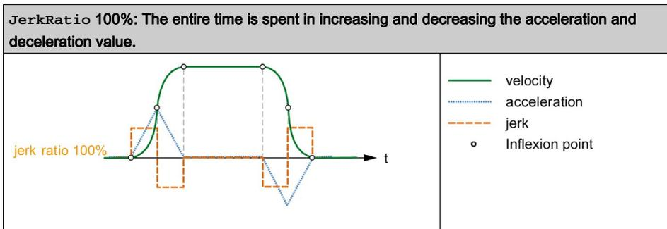
**NOTE:** The `JerkRatio` parameter value is common for acceleration and deceleration so that concave time and convex time are equal.
