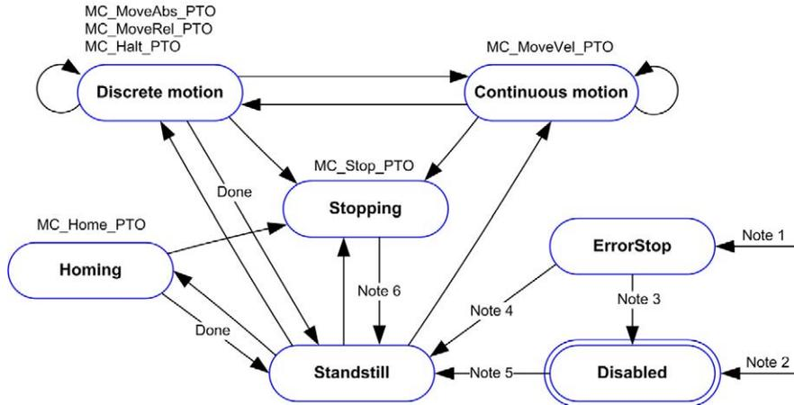
**Note 1** From any state, when an error is detected.
