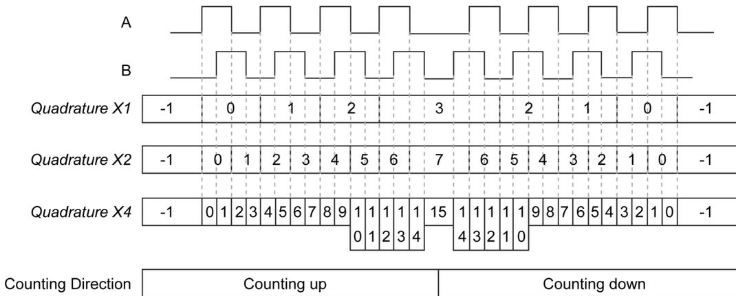
**Quadrature X1** When channel A leads channel B, the counter increments on the rising edge of channel A. When channel B leads channel A, the counter decrements on the falling edge of channel A.
