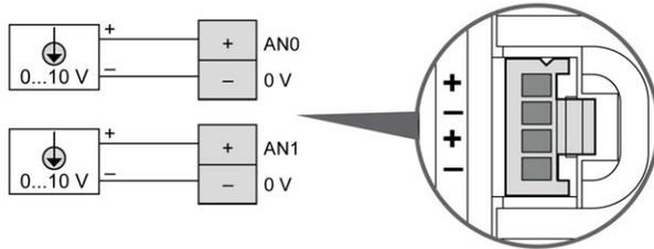
The (-) poles are connected internally.
