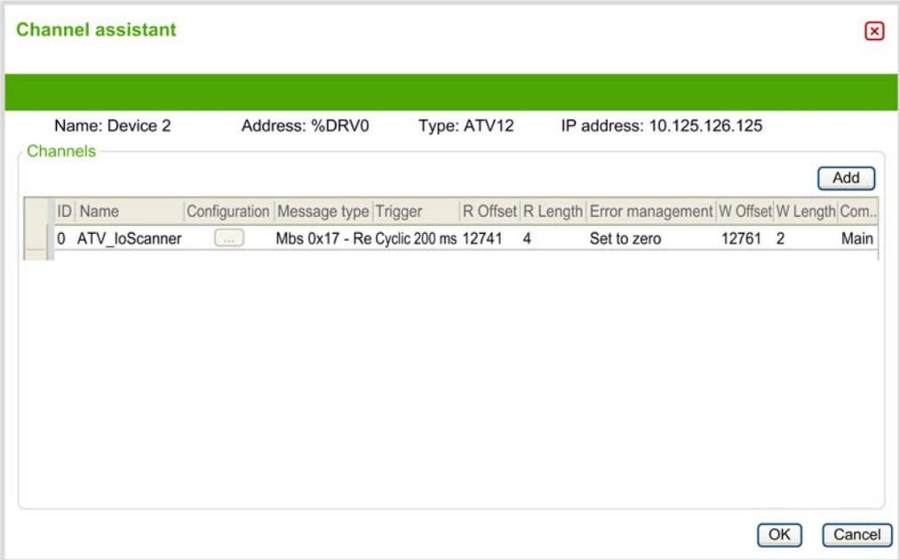
Preconfigured channels are displayed with a lock symbol
