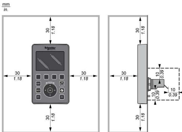
**NOTE:** Keep adequate spacing for proper ventilation and to maintain the operating temperature specified in the Environmental Characteristics ([see page 16](#)).
