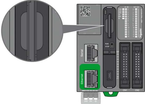
It is possible to set the Write-Control Tab to prevent write operations to the SD card. Push the tab up, as shown in the example on the right-hand side, to release the lock and enable writing to the SD card. Before using an SD card, read the manufacturer's instructions.
