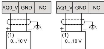
(1): Voltage analog input device
