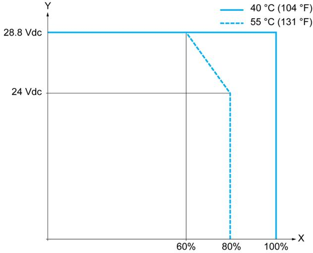
**X** Output simultaneous ON ratio
