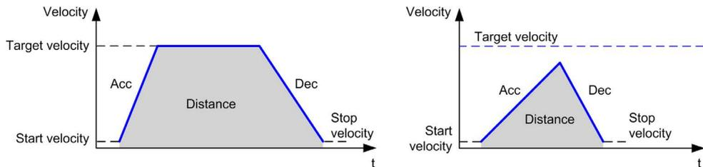
The diagram illustrates a complex profile from **Continuous** state:
