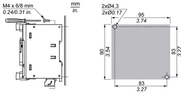
The following diagram shows the mounting hole layout for TM221C Logic Controller with 24 I/O channels:
