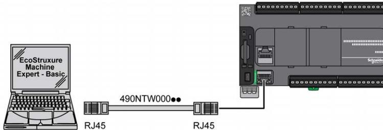
The following illustration shows the Ethernet connection to a PC on a TM221M Logic Controller:
