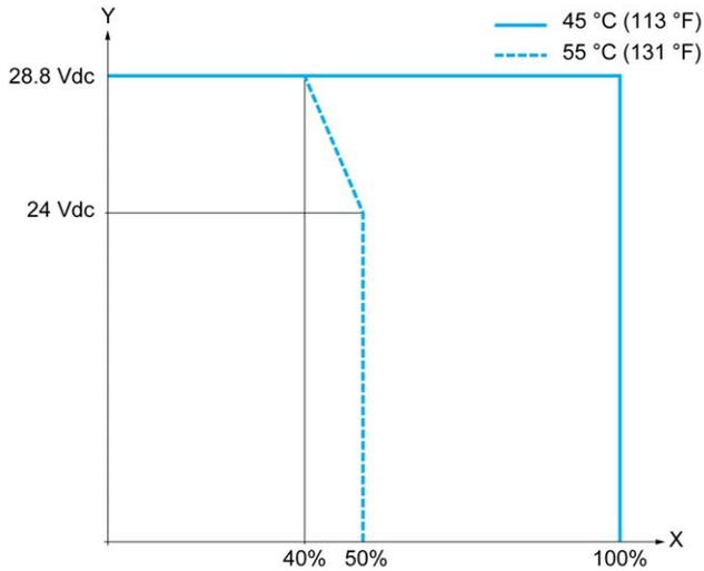
**X** Input simultaneous ON ratio
