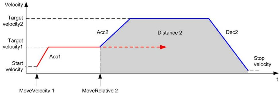
The diagram illustrates a complex profile from **Continuous** state with change of direction:
