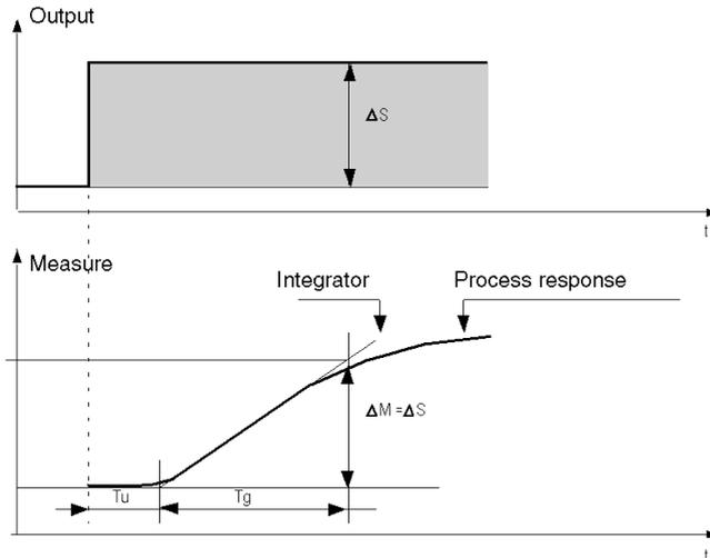
The intersection point on the right hand side, which is representative of the integrator with the time axes, determines the time  $T_u$ . Next, the  $T_g$  time is defined as the time necessary for the controlled variable (measurement) to have the same variation size (% of the scale) as the regulator output.
