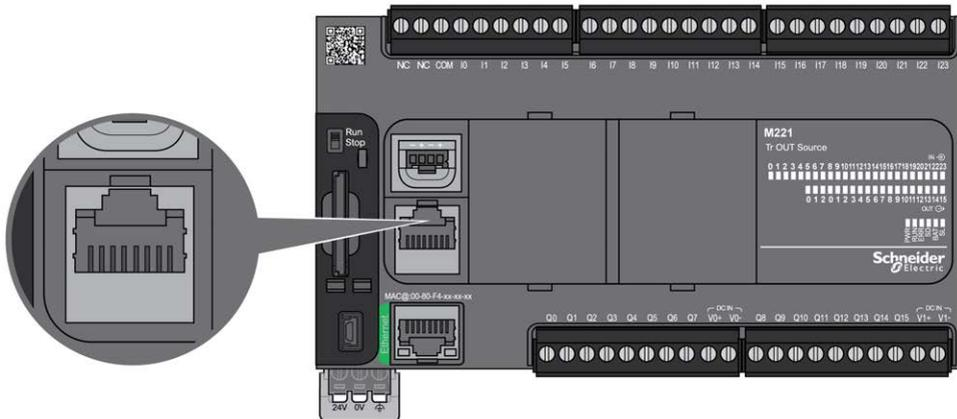
The following figure shows the location of the serial line 1 port on the TM221M Logic Controller:
