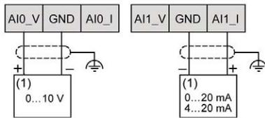
(1): Current/Voltage analog output device
