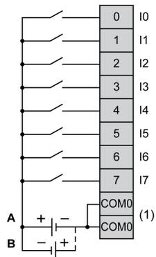
(1) The COM0 terminals are connected internally.
