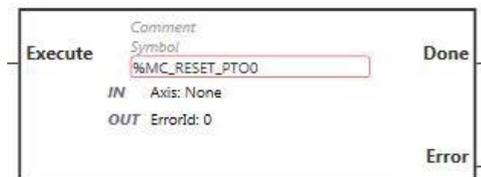
**NOTE:** When you first enter the function block, you must configure it to use the intended axis. Double-click on the function block to display the function block properties, choose the axis and click `Apply`.
