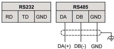
**NOTE:** Only 1 serial line (RS232 or RS485) can be connected to the cartridge.
