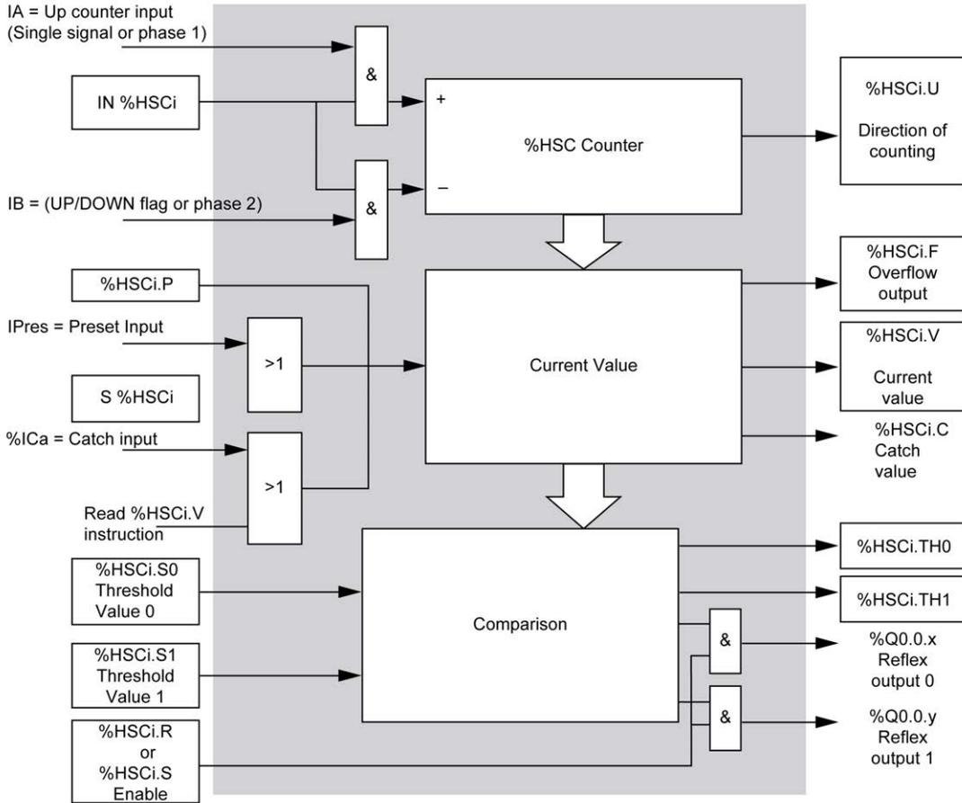
**NOTE:** Reflex outputs are managed independently from the controller cycle time.
