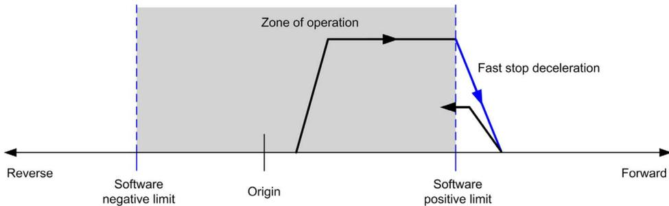
**NOTE:** In previous diagram, the axis move back in the limits is the result of the execution of `MC_Reset_PTO` (it is not performed automatically).
