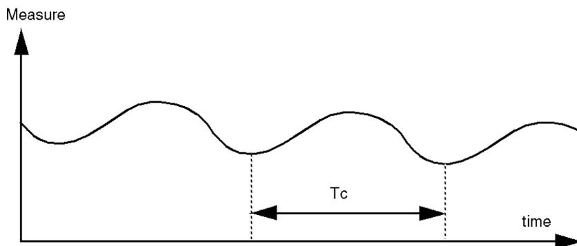
Depending on the corrector type used (PID or PI), the adjustment of the coefficients is executed with the following values:
