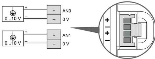
The (-) poles are connected internally.
