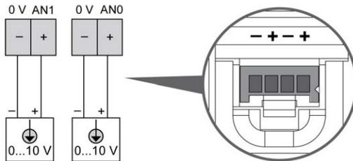
The (-) poles are connected internally.
