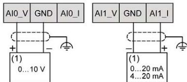
(1): Current/Voltage analog output device
