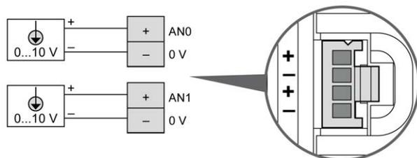
The (-) poles are connected internally.
