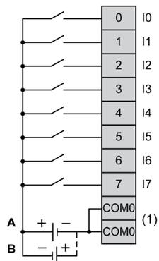
(1) The COM0 terminals are connected internally.
