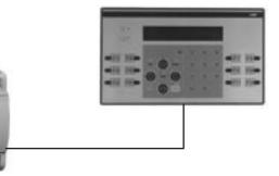
A display is continuously available to the operator, providing information on the production process. In real time, the user can intervene as soon as an anomaly appears.The operator terminal, connected to the TSX Nano terminal port can:
