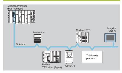
The Fipio fieldbus is a standard means of communication between different control system components. It enables 127 devices to be connected at the connection point integrated in the processor.
