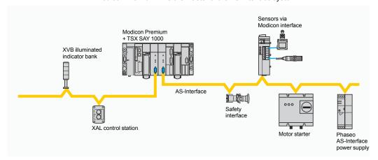
The AS-Interface cabling system consists of a master station (Modicon Premium PLC) and slave stations. The master supporting the AS-Interface profile interrogates the devices connected on the AS-Interface line one by one and stores the information (sensor/actuator status, device operating status) in the PLC memory. Communication on the AS-Interface line is managed totally transparently in relation to the PLC application program.
