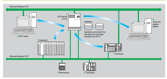
The OFS server 1 is at the centre of the data exchanges. It ensures that variables exchanged between the OPC client 2 and the PLC 3 are consistent, in one of three ways using a symbol (or variables) database:
