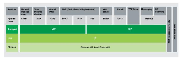
In addition to universal Ethernet services (HTTP, BOOTP/DHCP, FTP, etc.), the Transparent Ready device communication services designed for use in automation applications include:
