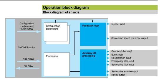
Axis control modules are set up using Unity Pro or PL7 Junior/Pro software. TSX CAY 22/42/33 modules require the use of Premium TSX P57 ●●3M/4M processors.
