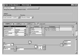
Configuring process control channels
