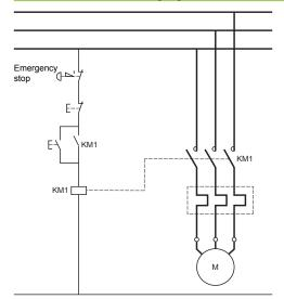
The control signal from the protection device (emergency stop pushbutton illustrated to the left) acts directly on the power contactor of the machine.
