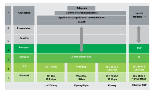
■ The physical layer enables the physical transmission of data signals between 2 systems via a medium.
