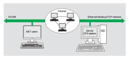
The .NET Microsoft compatibility of the OFS server has been developed to allow an OPC .NET client to access OFS server items on an Intranet network via the OPC .NET API interface.
