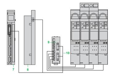
The motor starter is connected to an APP 1C● 7 module using an adaptor plate APP 2CX 8 and a cable APP 2AH40H060 10.
