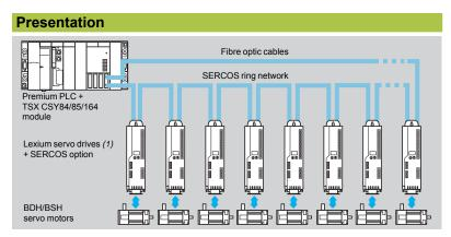
SERCOS (SERial COmmunication System) is a communication standard which defines the digital link (medium and exchange protocol) between the motion control module and servo drives. This standard is defined in European standard IEC/EN 61491
