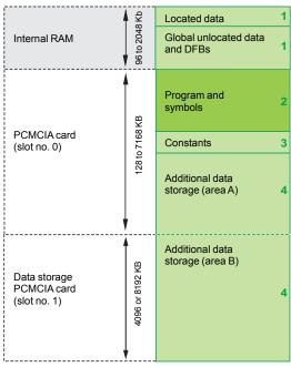
Processor with mixed type memory card in slot no. 0 and data storage type memory card in slot no. 1 (1)
