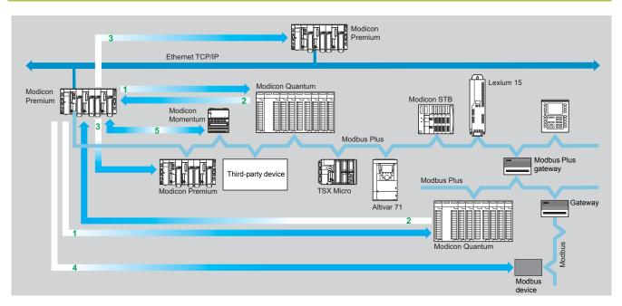
The Modbus Plus network is a high-performance industrial local network suitable for the requirements of Client/Server type extended architectures, combining high speed (1 Mbps), simple low-cost transmission media and numerous message handling services.
