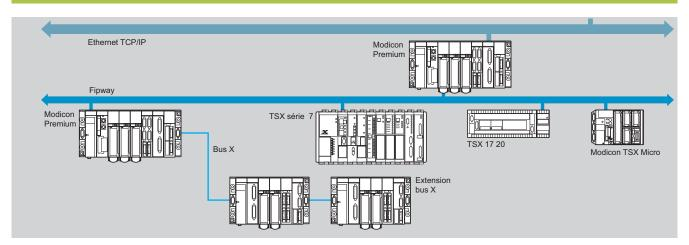
The Fipway network is an open industrial local area network for communication between the various Modicon TSX Micro, Modicon Premium and TSX Series 7 PLCs using the X-Way services. It conforms to the FIP standard with access via a bus arbitrator.
