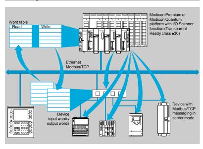
The I/O Scanning Service is used to manage the exchange of remote I/O states on the Ethernet network after simple configuration, with no need for any special programming.
