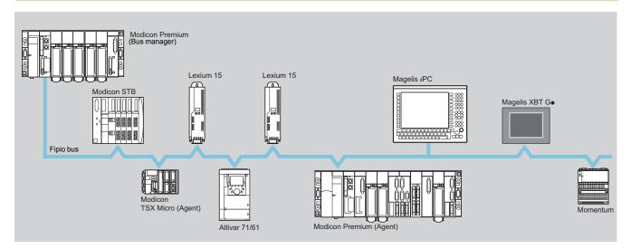
Modicon TSX Micro (TSX 37 21/22) or Modicon Premium PLCs, fitted with a PCMCIA **TSX FPP 10** card on their integrated communication channel, are agents on the Fipio bus. (With Fipio bus manager, see page 5/103).
