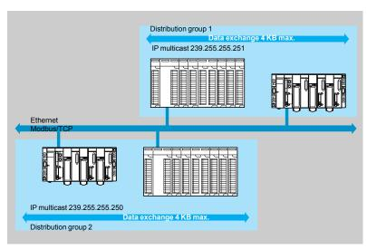
The Global Data service performs data exchanges in real time between stations belonging to the same distribution group. It is used to synchronize remote applications, or to share a common database between a number of distributed applications.
