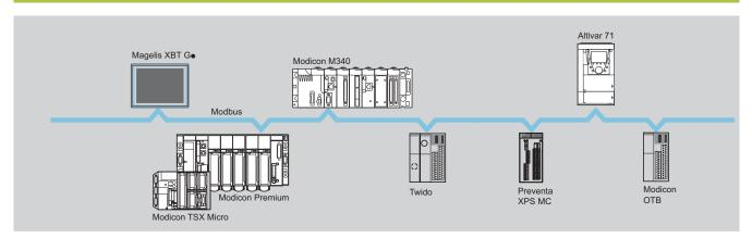
The Modbus serial link is used for master/slave architectures (it is necessary, however, to check that the Modbus services used by the application have been implemented on all devices concerned).
