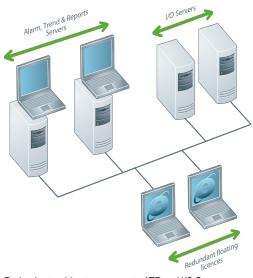
Redundant architecture, separate ATR and I/O Servers, with 2 Server Control Clients and 2 Web View Only Clients
