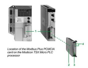
Modicon TSX Micro/Premium PLCs are connected to the Modbus Plus network via the **TSX MBP 100** type III PCMCIA card. This card is installed in the reserved slot on the processors:
