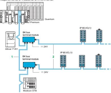
The topology of the INTERBUS bus is designed as a ring system with master/slave central access procedure.
