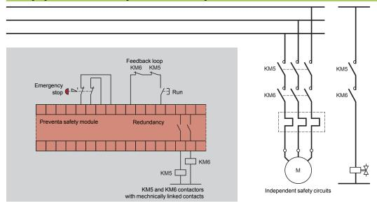
Preventa safety modules provide a reliable interposing relay function by eliminating the risks of:
