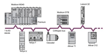
The CANopen bus is a multi-master bus providing reliable, deterministic access to real-time data in control system devices. The CSMA/CA protocol is based on broadcast exchanges, sent cyclically or on an event, ensuring optimum use of the bandwidth. A message handling channel can also be used to set the parameters of slave devices.
