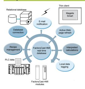
FactoryCast HMI Web services are integrated in the Web server modules embedded in the Modicon Premium and Modicon Quantum automation platforms.
