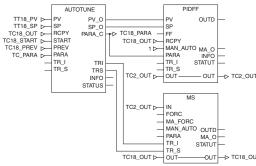
Example: PID controller with MS manual control
