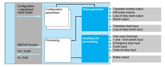
Stepper motor control modules are set up using Unity Pro or PL7 Junior/Pro software.
