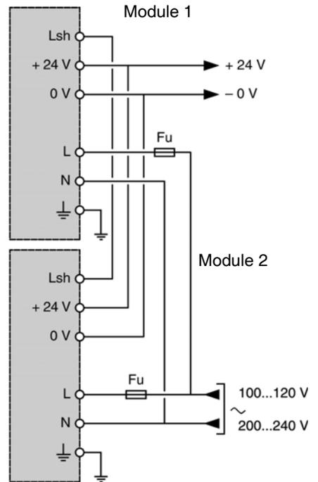
**Connection rules** **Primary:** observe the rules concerning phase and neutral when wiring.
