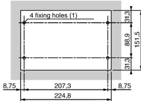
(1) The diameter of the fixing holes must be sufficient to take M6 screws.
