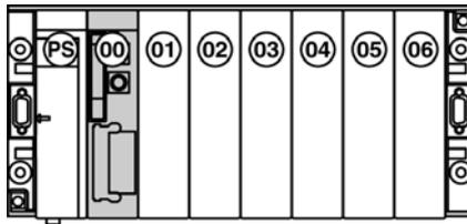
**Rack with double format power supply module:** TSX PSY 3610/5500/5520/8500.
