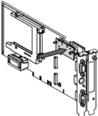
A technical drawing of the same processor card. A daughterboard is being inserted into the slot where the terminator was removed. The daughterboard is a smaller component that fits into the larger slot on the right side of the card.             |
