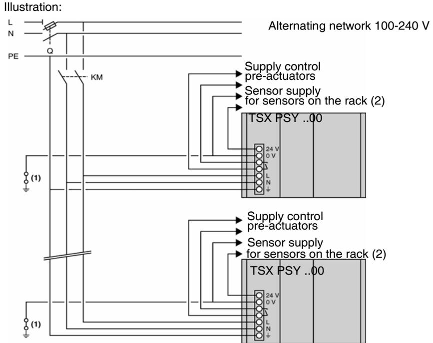
**Note:** if there are several PLC stations supplied by the same network, the principles of connection are identical.
