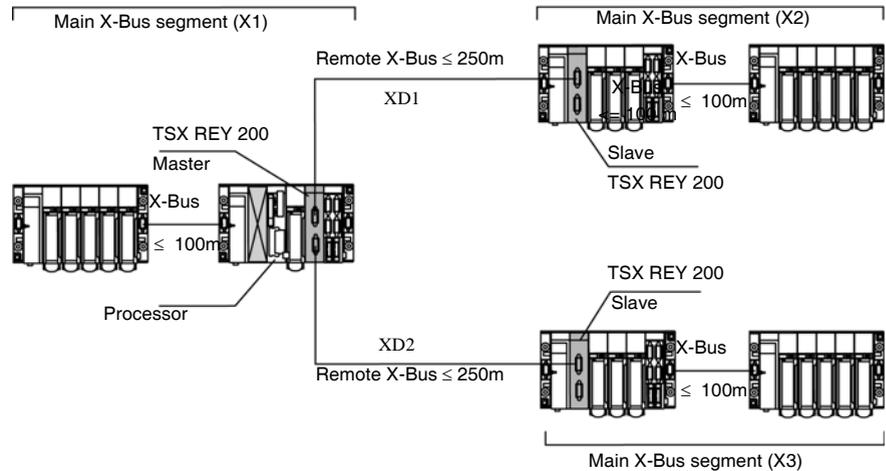
Taking this into account, the maximum distance possible between the processor and the remote modules is 350 meters.
