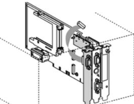
A technical drawing showing the processor card and daughterboard installed in a slot. A shield is being attached to the left side of the card. Dotted lines indicate the shield's position relative to the card and the adjacent slot to its left. |
