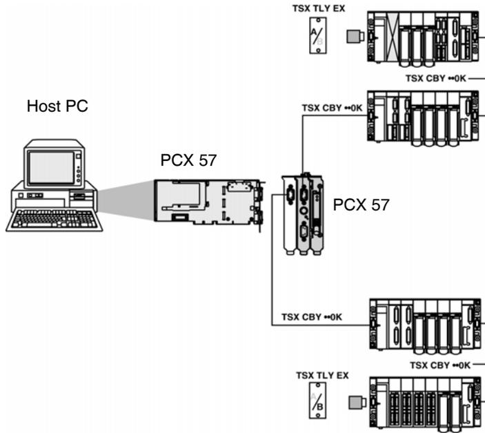
**Note:** in this example, as the PCX 57 processor is no longer integrated at the start of the line, the **TSX TLY EX A/** and **/B** line terminators must be installed on each of the racks situated at the end of the lines.
