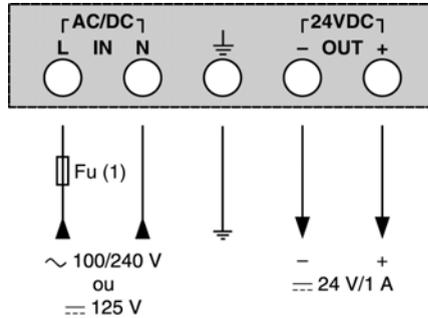
(1) External protection fuse on phase: 1A time delay 250V if single supply block.
