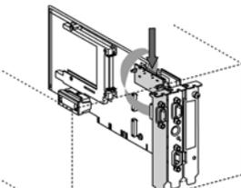
A technical drawing showing the processor card and daughterboard installed in a slot. A cable is being connected to a connector on the daughterboard. Dotted lines indicate the cable's path and connection point.                                |
