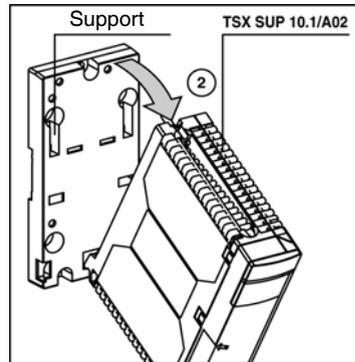
**Mounting on an AM1-ED\*\*\* mounting rail**
