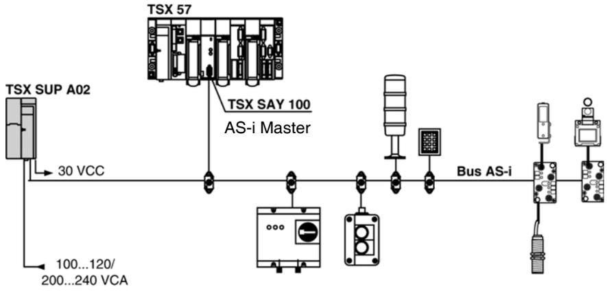
**Connection rules** **Primary:** observe the rules concerning phase and neutral when wiring.
