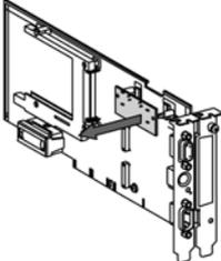
A technical drawing of a processor card. A metal bracket, which is the terminator, is shown being removed from a slot on the right side of the card. The card is oriented vertically with the connector edge at the bottom.                          |
