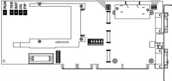
Position of the RACK ADD micro-switches in relation to the rack address:
