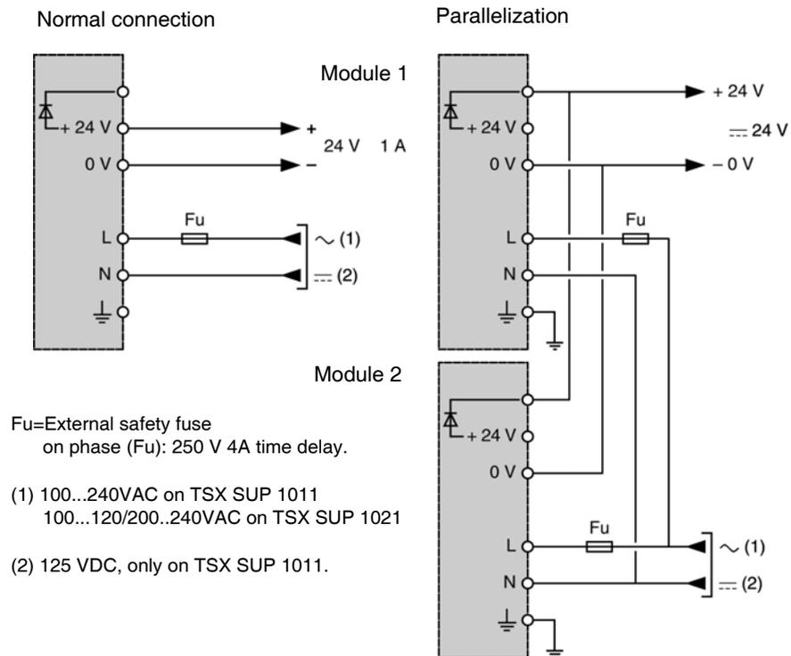
**Connection rules** **Primary:** if the module is supplied with a 100/240V AC power supply, it is necessary to observe wiring requirements for the phase and neutral when connecting the module. However, if the module is powered by a 125 VDC supply, it is not necessary to respect the polarities.
