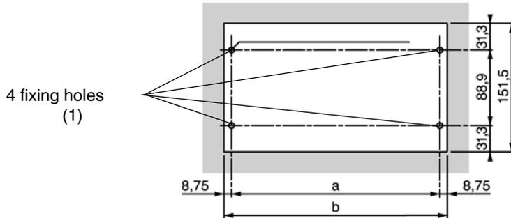
(1) the diameter of the fixing holes must be sufficient to take M6 screws.
