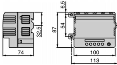
The TBX SUP 10 supply block must be mounted in an upright position to allow for the best possible natural air convection within the block.
