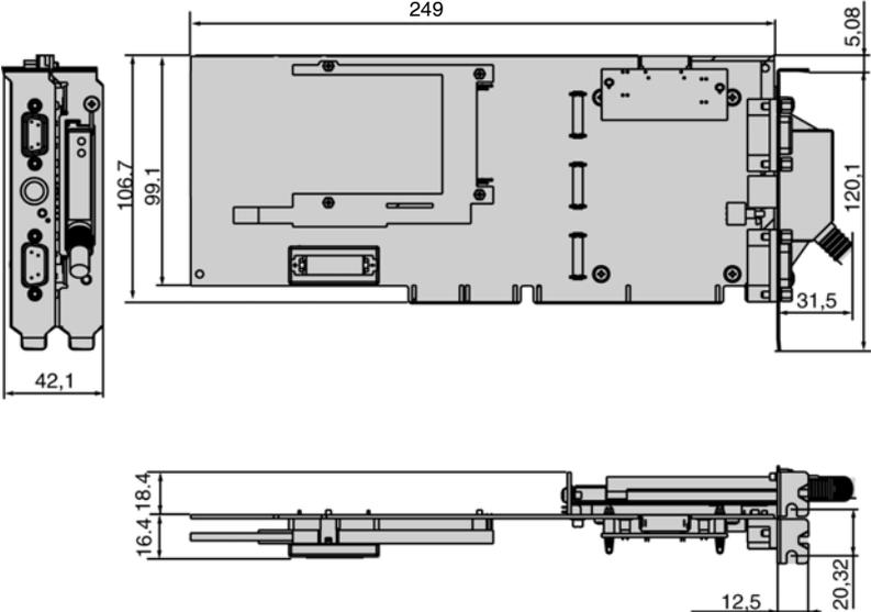
**Note:** a PCX 57 processor uses two slots on the PC ISA bus. These slots must be adjacent and 20.32mm apart.
