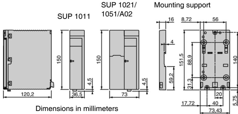
TSX SUP 1011/1021/1051/A02 power supply modules can be mounted in different ways:
