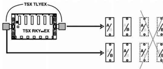
**Note:** When a single extendable rack is used, a line terminator must always be mounted on each of the rack's 9-pin SUB D connectors.
