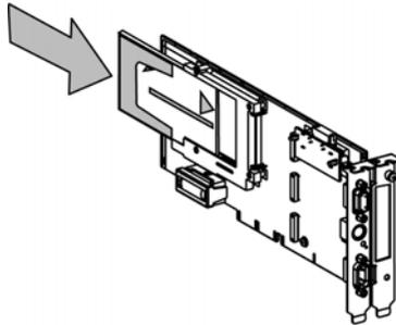
**Note:** if the program in the PCMCIA memory cartridge contains the **RUN AUTO** option, the processor will automatically restart in RUN mode after the cartridge is inserted and the PC is turned on.
