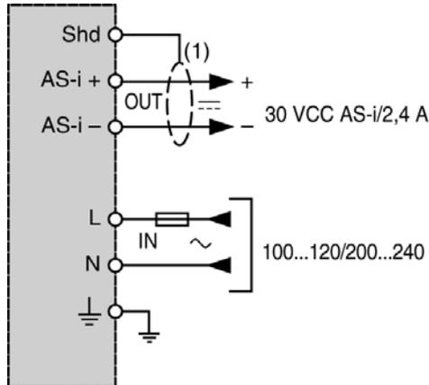
(1) Shielded AS-i cable screen if environment is disturbed.
