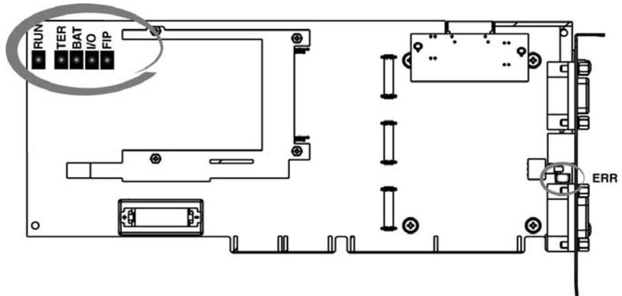
Due to the small amount of space available on the shield, only the ERR LED is visible when the PC housing the processor is closed.
