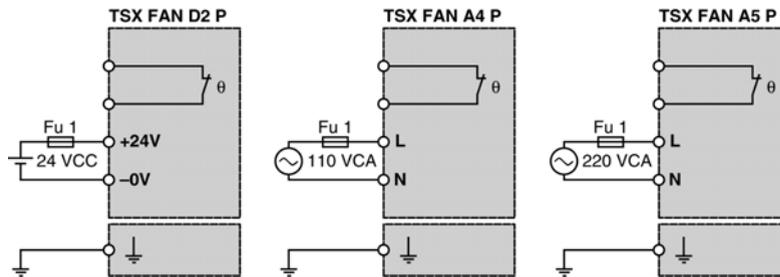
**Note:** If several ventilation modules of the same type are used, a common power supply should be used for all ventilation modules.
