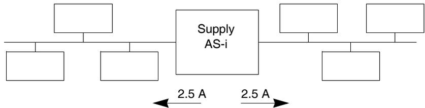
If there is no slave which consumes large amounts of power, it would be better to place the supply module in the middle of the installation. Conversely, if the installation has one or several large power consumers, it would be wise to place the supply module close to them.
