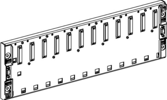
A perspective view of a TSX RKY 12EX rack. It is a long, thin metal frame with twelve vertical slots for modules. The front edge has twelve small rectangular cutouts. The top edge has a series of mounting holes and a locking mechanism on the right side. |
