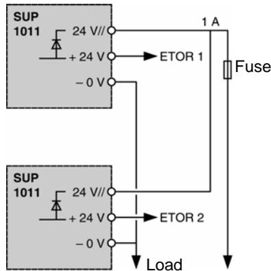
Discrete inputs 1 and 2 on the PLC indicate the failure of one or other of the power supplies.
