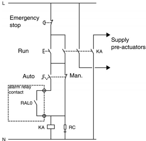
KA: contact controlled by alarm relay from supply module in AUTO run mode.
