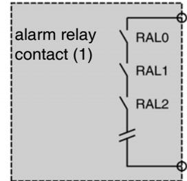
(1) When the PLC station is composed of several racks: set all the "alarm relay" contacts in series (RAL0, RAL1, RAL2, etc.).
