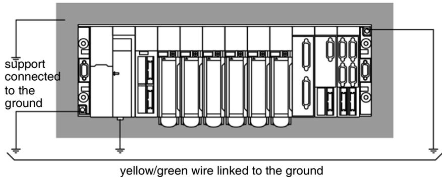
**Note:** The PLC's internal 0V is linked to the ground connection. The ground connection itself being linked to ground.
