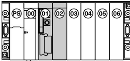
**Note:** the rack on which the processor is installed always has address 0.
