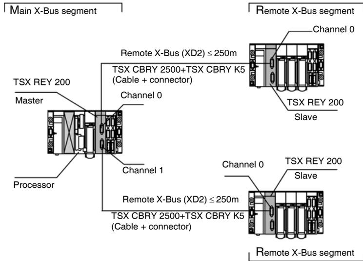
**Note:** Each X-Bus segment must have a A/ and B/ line terminator (See *Line terminator TSX TLYEX, p. 105*) at each end.
