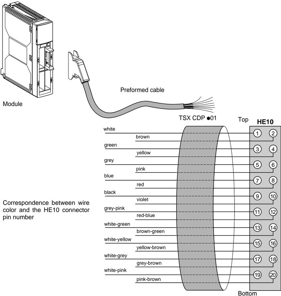
**Preformed stranded sheathed connection cable 28 gauge (0.08 mm<sup>2</sup>)**
