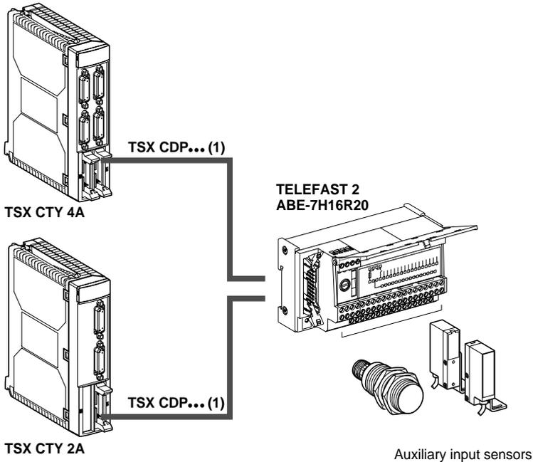
(1) TSX CDP ●●2 pre-formed cable or TSX CDP ●●3 cable (see part B - section 5.1-2 for characteristics).
