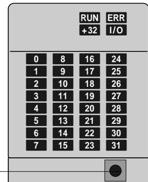
Switch for displaying channels higher than 31
