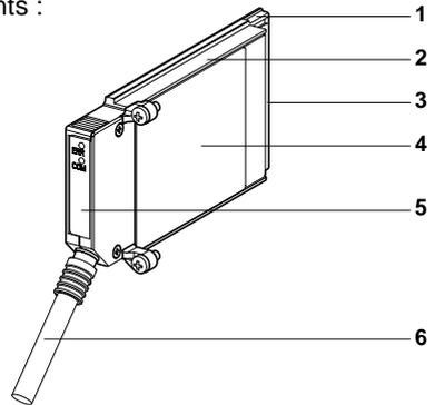
The removable cover (5) displays the operating status of the card in its environment. The function of the two indicator lamps is printed on the front of the removable cover.
