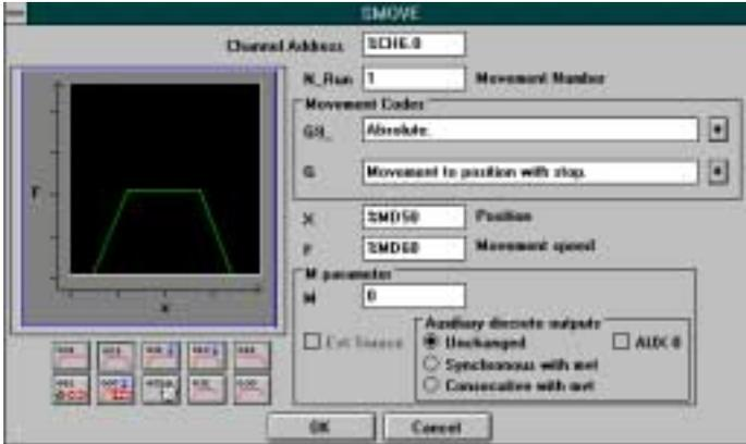
Screens for adjusting the axis parameters and setting up movements can also be accessed via PL7 Junior.
