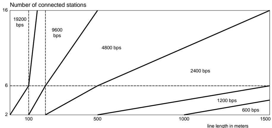
The performance of a multidrop link is much improved when a large number of stations are connected. The load on the line is greater, which improves the quality of the transmitted signal.
