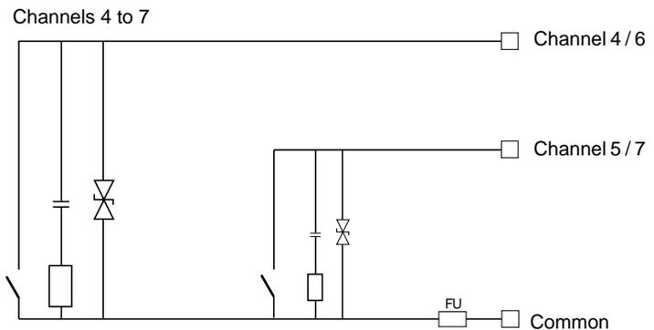
FU = 6.3 A - interchangeable fast blow fuse. 1 fuse per common.
