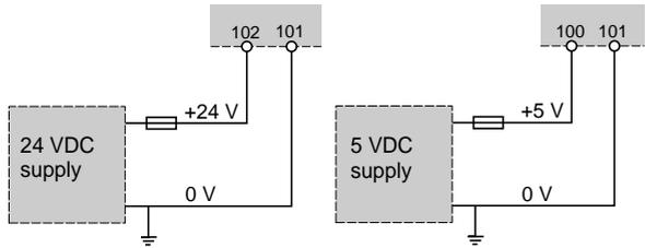
**Important :** the maximum length of the wires between the supply outputs and the Telefast connecting pins must be less than 0.5m.
