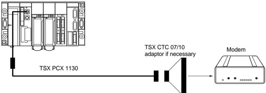
**Example 1 :** for a terminal port in UNI-TELWAY master mode connected to a modem/telephone network in response mode, numbers 1 to 6 of the above characteristics are required.
