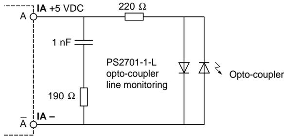
Inputs IA, IB and IZ used in RSS 422 are totally compatible with incremental encoder line drivers with RS 422 outputs and also with encoders with pushpull complementary outputs with a 5 V power supply. Line monitoring is performed on each output.
