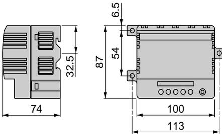
The TBX SUP 10 power supply block should be mounted vertically to ensure optimal air flow within the block.
