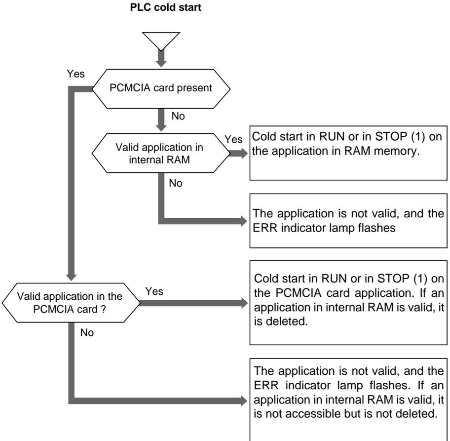
(1) Starting in RUN or in STOP is defined during configuration
