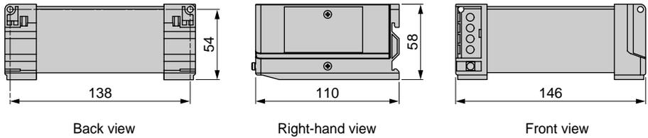
• Fan module + rack (measurements in millimeters)
