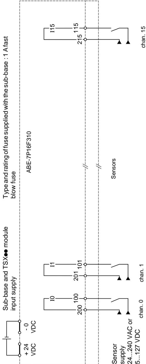
Provide one protection fuse per group of sensors if they are supplied with the same voltage
