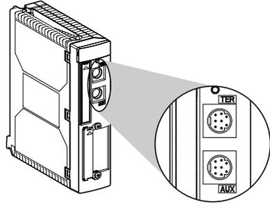
Note : the user-defined communication protocol is identical for both ports.
