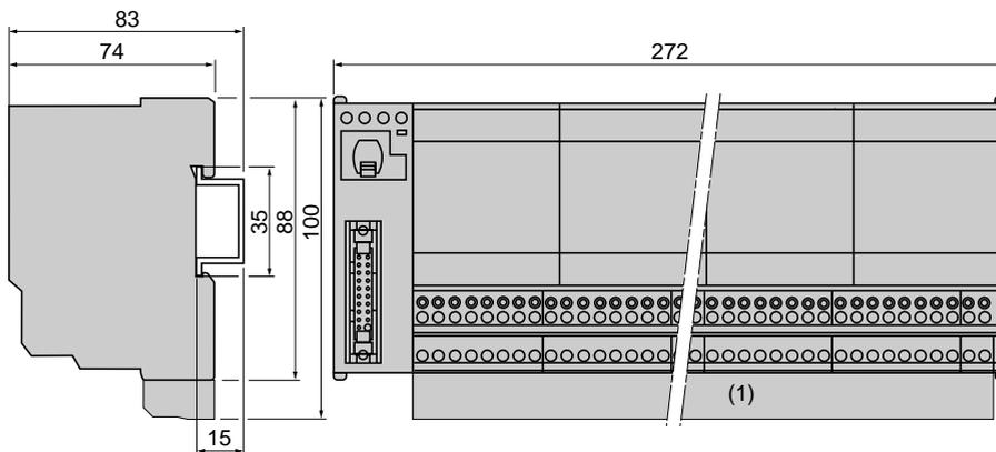
Reference with dimensions of 272x88 mm (product pictured with removable relays and screws not mounted)
