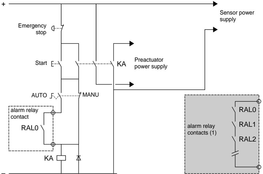
KA : contactor interlocked with the alarm relay of the power supply in AUTO operation.
