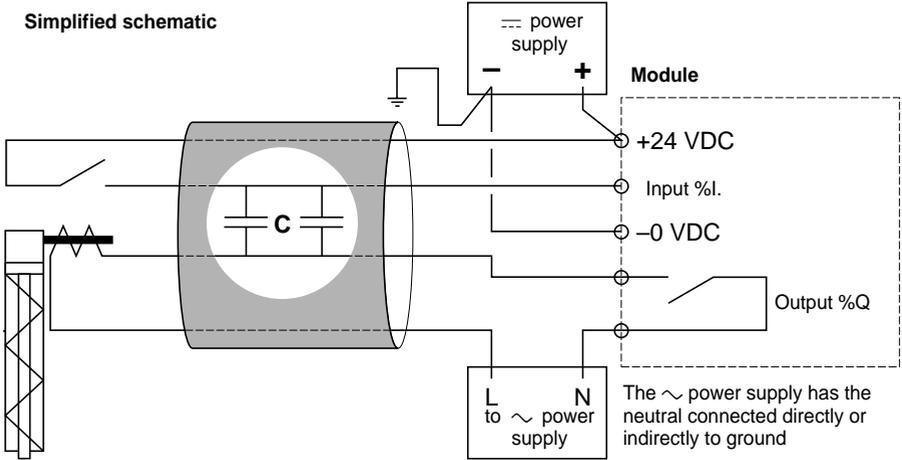
When the contact at the input is open, AC crossing the parasitic capacitance of the cable may generate a current in the input which may cause it to change to state 1.
