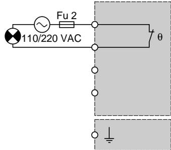
Note : when using several fan modules, the probe contacts will be placed in series.
