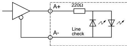
5V supply, totem pole outputs. Differential line check on each input.
