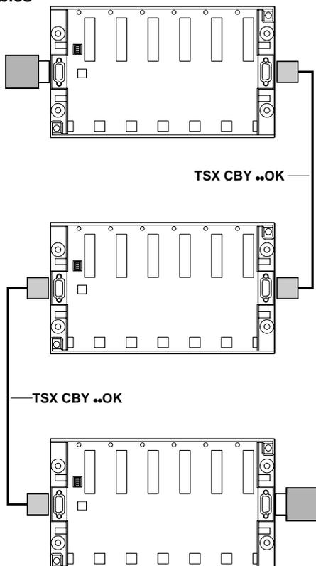
**⚠** The total length of all the cables used in a PLC station is limited to 50 meters.
