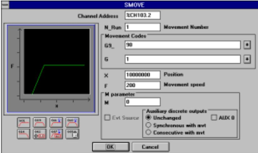
Screens for adjusting the axis parameters and setting up movements can be accessed via the PL7 Junior software.
