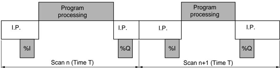
**I.P.** (internal processing) : the system implicitly monitors the PLC (managing the system bits and words, updating the realtime clock current values, updating the status indicator lamps, detecting changes to RUN/STOP, etc) and processing requests originating from the programming terminal or the communication system,
