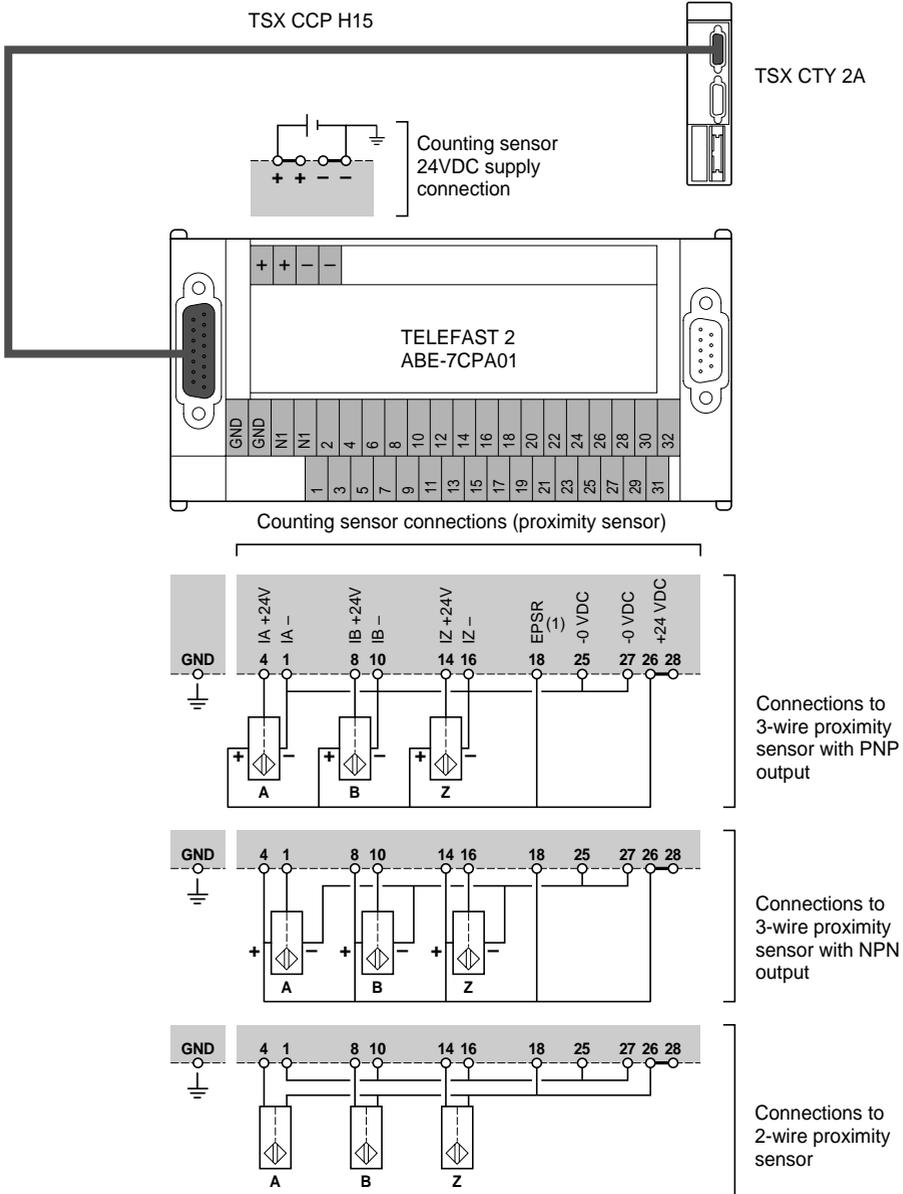
(1) When the counting sensors are proximity sensors, the EPSR input (encoder power supply return) must respect polarity :
