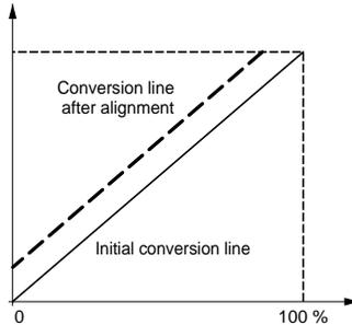
For example, suppose that a pressure sensor, linked to a conditioning unit (1mV/mB), indicates 3200 mB, while the actual pressure is 3210 mB. The value measured by the module in standard scale will be 3200 (3.20 V). The user can align the measurement to the value 3210 (required value). After this alignment procedure, the measurement channel will apply a systematic offset of +10 to any new measurement.
