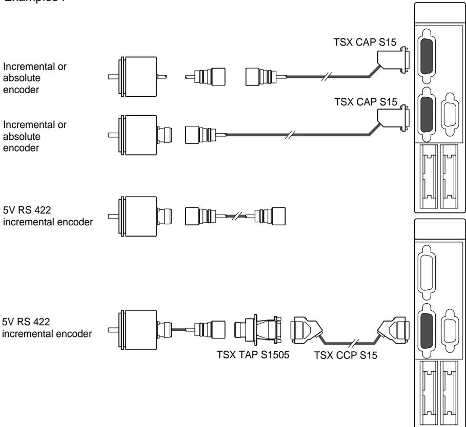
These accessories provide good signal and shielding continuity in adverse conditions. The encoder connection cables are generally offered by the encoder suppliers.
