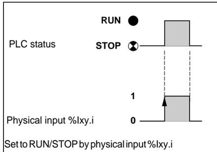
Setting the PLC to STOP using this physical input has priority over setting it to RUN from a terminal or network.
