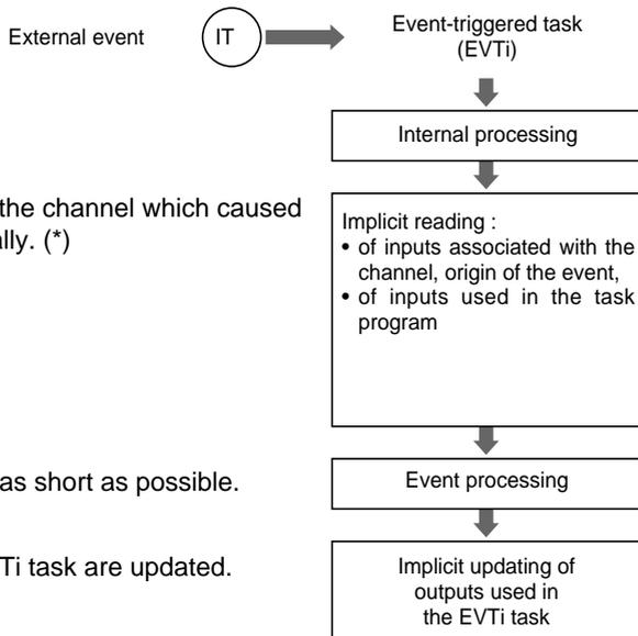
All the inputs associated with the channel which caused the event are read automatically. (\*)
