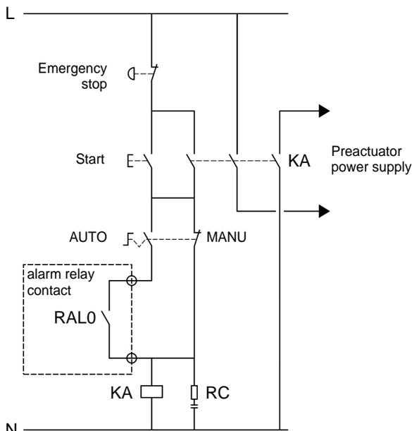
KA : contactor interlocked with the alarm relay of the power supply in AUTO operation.
