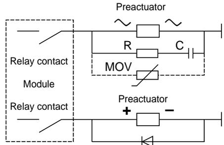
**Note :** A relay output, used on an AC load, must not then be used on a DC load and vice versa.
