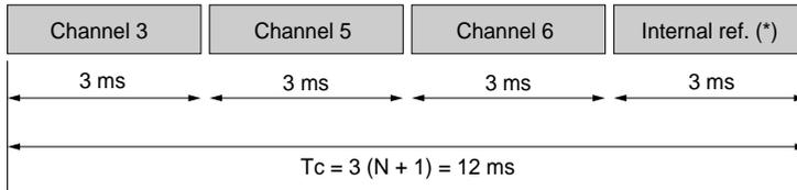
(\*) corresponds to the acquisition of voltage references integrated in the module, to enable its periodic autocalibration.
