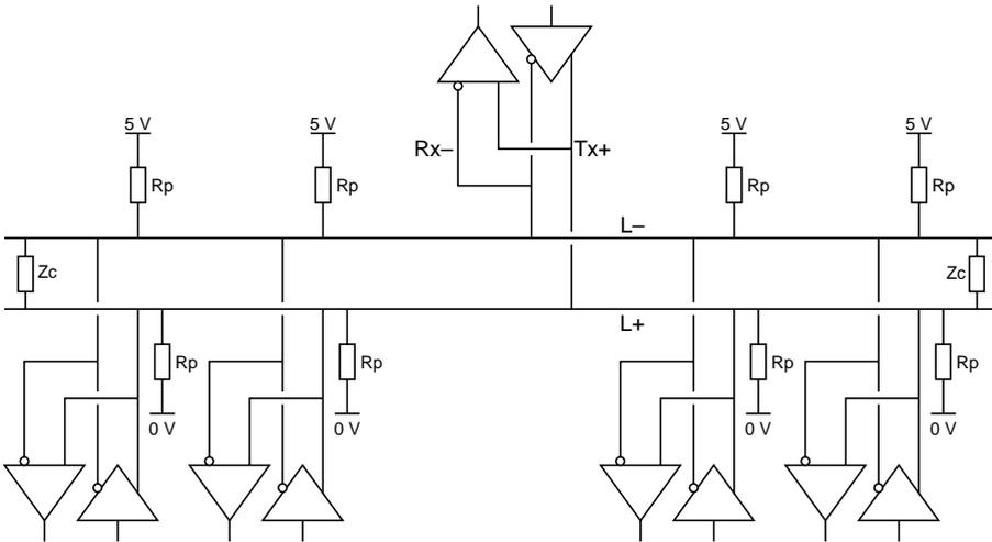
The above diagram shows the general architecture of a UNI-TELWAY network.
