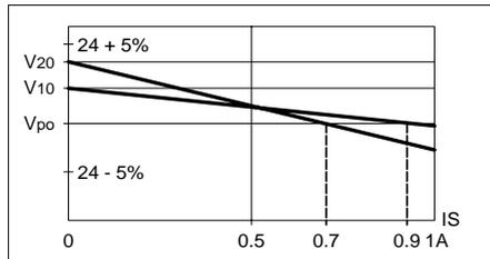
Parallel operation "with power optimization" is active when the **NOR/LSH** switch at the rear of the module is in the LSH position. The orange LED on the front of the module is lit when the mode is operational.
