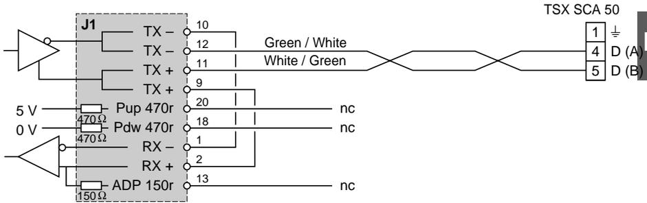
Connection of SCA 50 with line terminator
