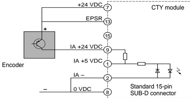
**Schematic for channel connection**
