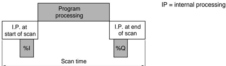
$$\text{MAST scan time} = \text{Program processing time (Ttp)} + \text{Internal processing time at start and end of scan (Tti)}$$
