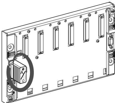
TSX TLY line terminators are sold in lots of 2 and marked A and B. Each end of the bus must, without fail, have an A line terminator or a B line terminator (see diagrams below).
