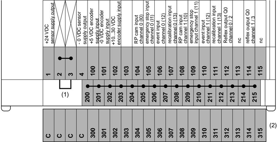
(1) On the ABE-7H16R20 sub-base, the position of the jumper defines the polarity of all 2•• terminals :
