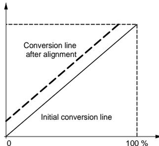
For example, suppose that a Pt100 probe, plunged into melting ice (probe adjustment procedure) displays 10 °C after measurement (and not 0 °C). The user can align the measurement to the value 0 (required value). After this alignment procedure, the measurement channel will apply a systematic offset of -10 to any new measurement.
