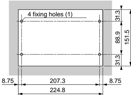
(1) The diameter of the fixing holes must be large enough to take M6 screws.
