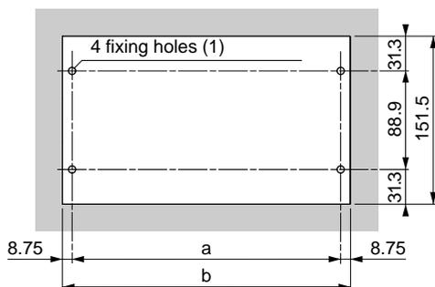
(1) The fixing hole diameter must be large enough for M6 screws.
