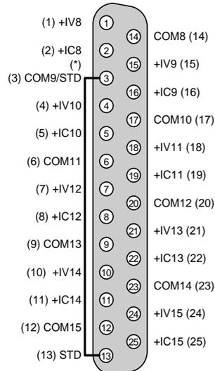
+IVx : +ve voltage input of channel x
