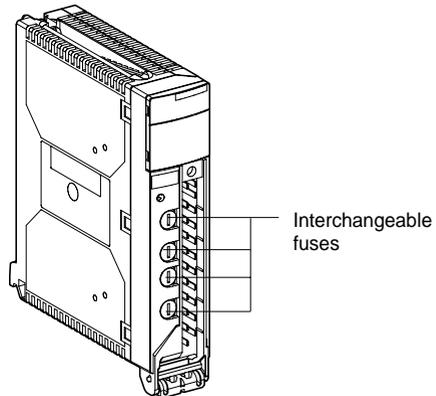
The fuses can be accessed once the terminal block has been removed.
