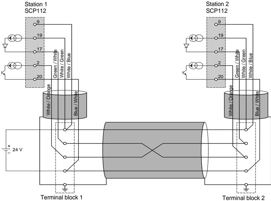
**Important :** the cable shielding must be connected as closely as possible to the terminal blocks.
