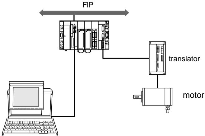
The CFY 11/21 stepper motor axis control range for TSX model 57 PLCs is designed to meet the requirements of machine manufacturers.
