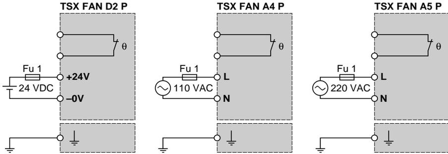
Note : when using several fan modules of the same type, use one common power supply for all the fan modules.
