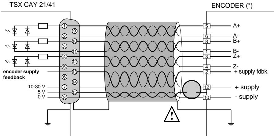
(\*) standard pin-out of an encoder with a 12-pin DIN connector.
