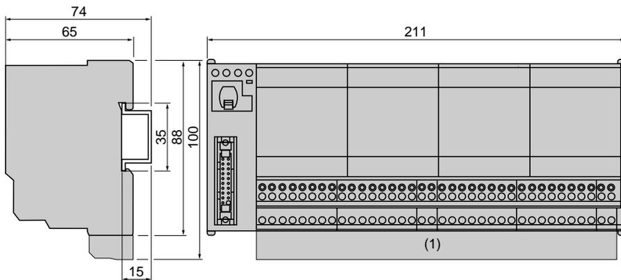
Reference with dimensions of 211x88 mm (product pictured with removable relays and screws not mounted)
