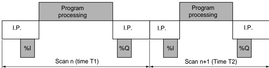
**I.P.** (internal processing) : the system implicitly monitors the PLC (managing the system bits and words, updating the realtime clock current values, updating the status indicator lamps, detecting changes to RUN/STOP, etc) and processing requests originating from the programming terminal or the communication system,
