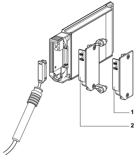
Connection to the network is obtained by connecting the cable to the front of the card. A module locating device prevents incorrect mounting. The product reference label informs the user of the type of physical layer supported by the card.
