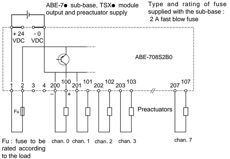
6.5-15 Solid state or electromechanical relay output sub-bases, relay 10mm wide
