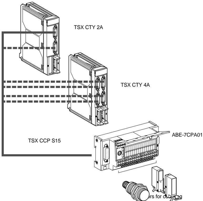
A 9-pin SUB-D connector is used to transfer information to an Altivar drive when using this sub-base with analog I/O.
