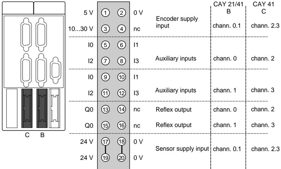
Channels 2 and 3 are assigned to the TSX CAY 41 module
