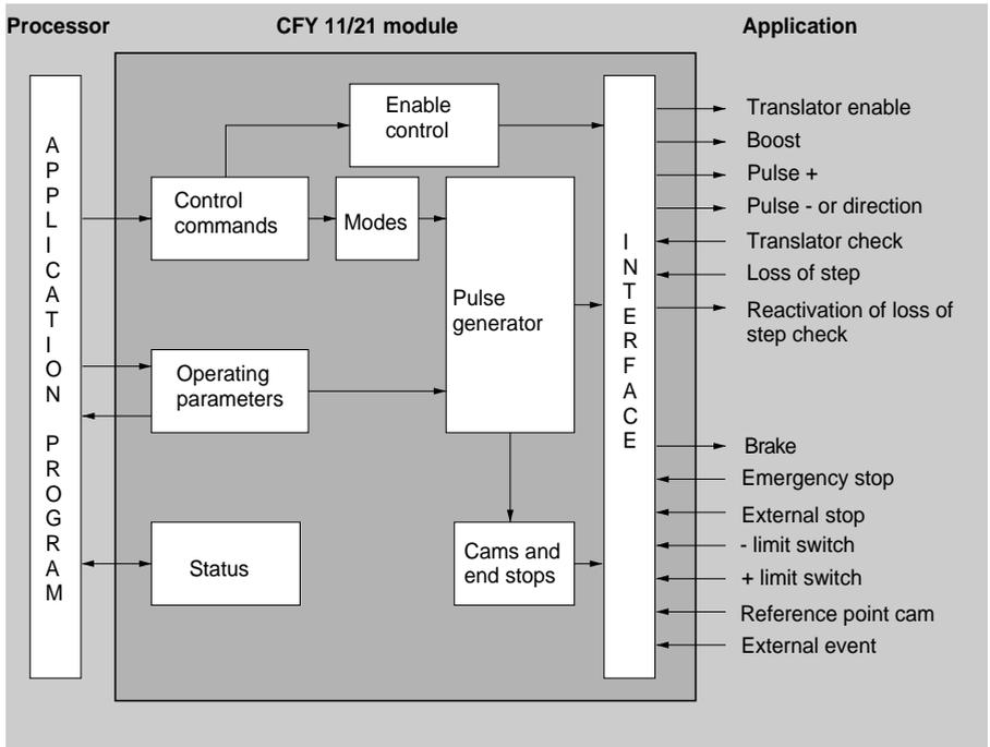
CFY 11/21 stepper motor axis control modules provide for each axis :
