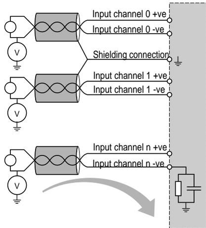
For safety reasons, the modules are fitted with an RC network ( $>30\text{ M}\Omega$ ,  $4.7\text{ nF}$ ), which grounds the reference voltage of the channels.
