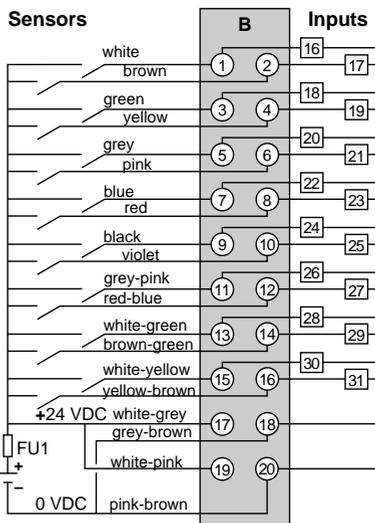
TSX DEY 64D2K module connections
