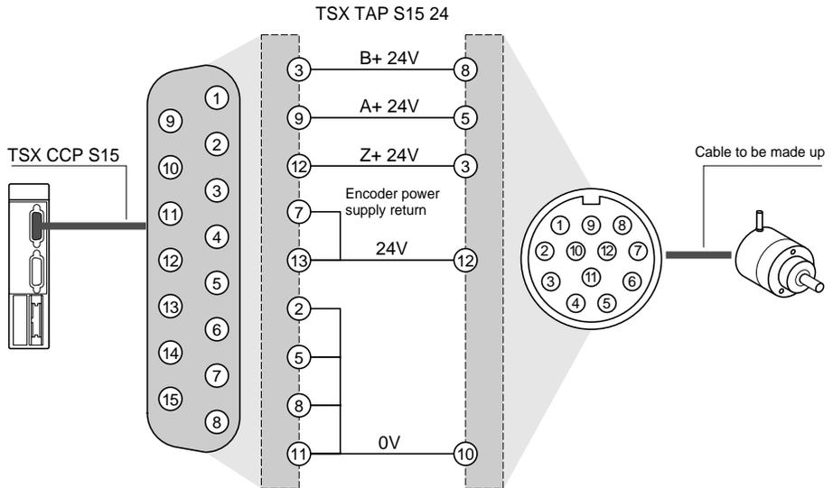
This type of connection is compatible with encoders with a 24V supply :
