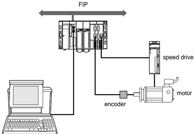
The servo-loop positioning axis control range for TSX model 57 PLCs is designed to meet the requirements of machine manufacturers. It is designed for machines which require high-performance motion control together with simultaneous sequential control via a PLC. The range is used to control movements on a restricted independent axis or on an infinite linear axis.
