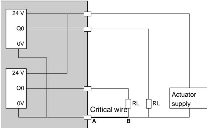
If there is a break in the supply cable segment between A and B, there is a risk of the RL actuators remaining energized. If possible, double the 0V supply connections for the module(s).
