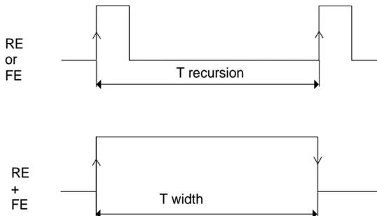
$$T \text{ recursion or } T \text{ width} > 0.25 \text{ ms} + 0.25 \times \text{module event number}$$
