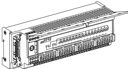
• **Connection interface and solid state output adaptor sub-bases, 8 and 16 channels :**
