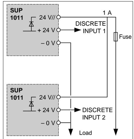
For power supplies operating in parallel, it is recommended to use the "power optimization mode" to ensure optimum lifetime of the 2 modules. Otherwise, the power supply with the higher output voltage will try to supply the maximum current with the other having practically no-load. The lifetime of the first supply will decrease more rapidly than that of the second supply.
