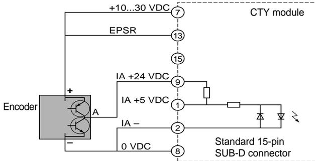
**Schematic for channel connection**
