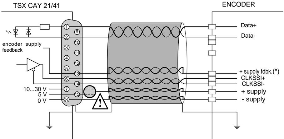
⚠ The encoder supply must be connected to pin number 15 or 7 of the Sub-D connector depending on the encoder supply voltage.
