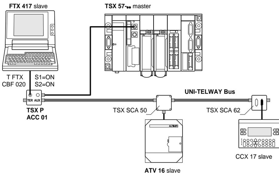
The connected devices communicate with the PLC using UNI-TE protocol.
