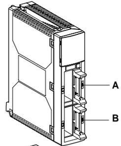
The TSX DEY 64D2K module is fitted with 4 HE10 male connectors :
