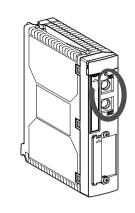
The default communication mode for the TER and AUX connectors is UNI-TELWAY master at 19200 bauds and, by configuration, UNI-TELWAY slave mode or ASCII character mode.
