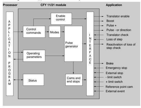
CFY 11/21 stepper motor axis control modules provide for each axis :
