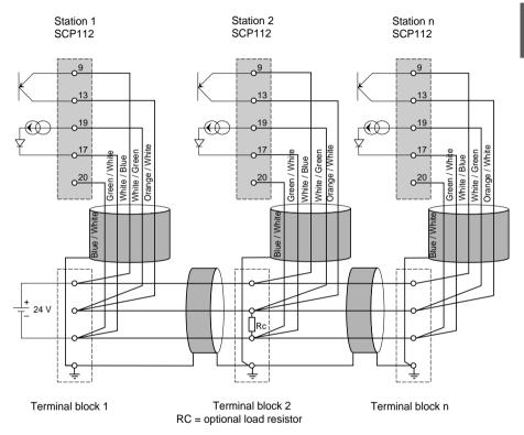
**Important**: the cable shielding must be connected as closely as possible to the terminal blocks.
