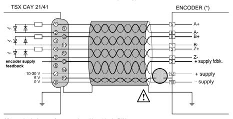
(\*) standard pin-out of an encoder with a 12-pin DIN connector.
