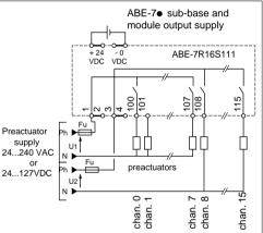
Type and rating of fuse supplied with the sub-base : 1 A fast blow fuse.
