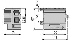
The TBX SUP 10 power supply block should be mounted vertically to ensure optimal air flow within the block.
