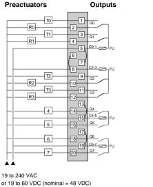
= strap 24 V must be connected when using 24 V AC or DC.
