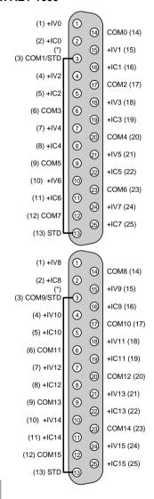
+IVx : +ve voltage input of channel x +ICx : +ve current input of channel x
