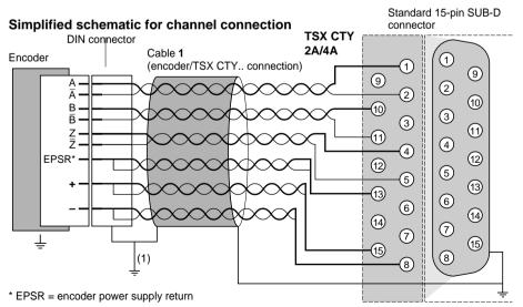
(1) This link should be made directly if the encoder is isolated from ground
