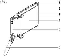
The removable cover (5) displays the operating status of the card in its environment. The function of the two indicator lamps is printed on the front of the removable cover.
