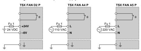
Note: when using several fan modules of the same type, use one common power supply for all the fan modules.
