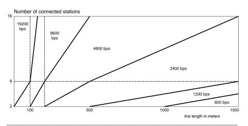
The performance of a multidrop link is much improved when a large number of stations are connected. The load on the line is greater, which improves the quality of the transmitted signal.
