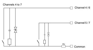
FU = 6.3 A - interchangeable fast blow fuse. 1 fuse per common.
