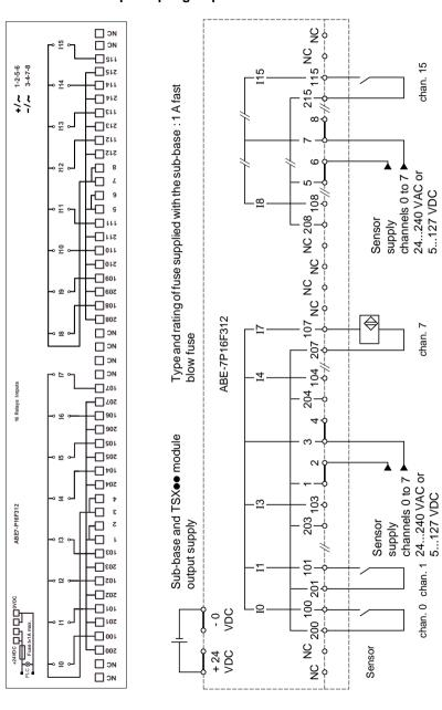
Provide a protection fuse for the sensor supply
