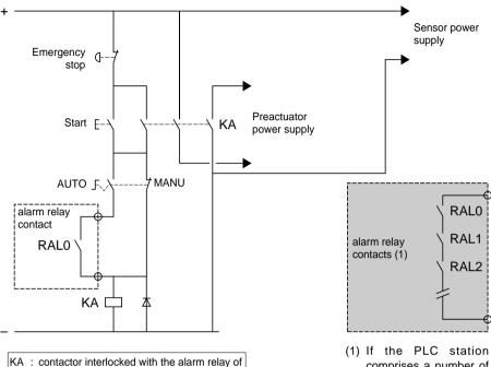
KA: contactor interlocked with the alarm relay of the power supply in AUTO operation.
