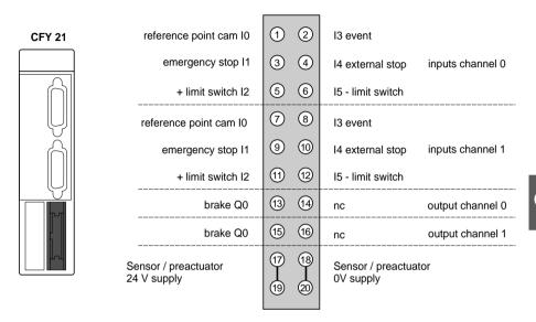
The 0V connection for the sensors / preactuators should be connected within the module to machine ground by an R/C circuit with value :  $R = 10M\Omega / C = 4.7nF$ .
