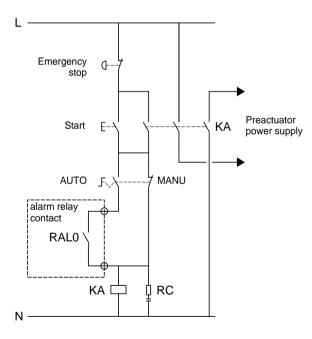
KA: contactor interlocked with the alarm relay of the power supply in AUTO operation.
