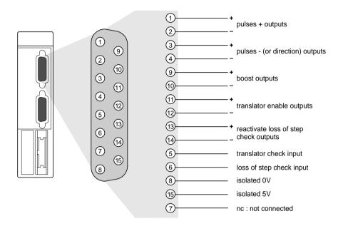
Each module output transmits an RS 485-type signal, and for each output there is thus a direct (+) signal and its complement (-). The inputs are TTL-compatible current sinking inputs. The 5V isolated supply is only available (if necessary) for the translator I/O interface. The 0V supply is common to both inputs and outputs. The 5V supply may only be used for translators with open collector outputs and TTL-type inputs (the 5V isolated supply is not supplied by the translator).
