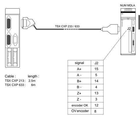
Note: in this case no encoder supply is necessary.
