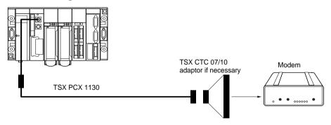
**Example 1**: for a terminal port in UNI-TELWAY master mode connected to a modem/ telephone network in response mode, numbers 1 to 6 of the above characteristics are required.
