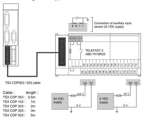
**Important**: the maximum length of the wires between the supply outputs and the Telefast connecting pins must be less than 0.5m.
