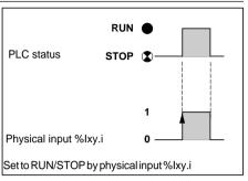
Setting the PLC to STOP using this physical input has priority over setting it to RUN from a terminal or network.
