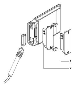
Connection to the network is obtained by connecting the cable to the front of the card. A module locating device prevents incorrect mounting. The product reference label informs the user of the type of physical layer supported by the card.
