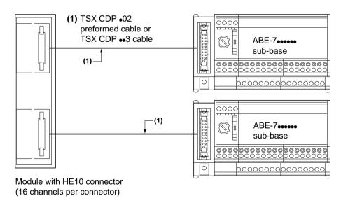
Connection of 16 channels (2 x 8) using an ABE-7ACC02 adaptor sub-base. Example 1 : Connection of 16 channels (2 x 8)
