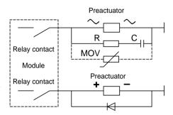
Note: A relay output, used on an AC load, must not then be used on a DC load and vice versa.
