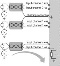
For safety reasons, the modules are fitted with an RC network (>30 M $\Omega$ , 4.7 nF), which grounds the reference voltage of the channels.
