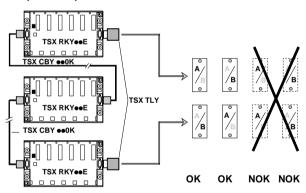
On a PLC station with a single TSX RKY••E extendable rack Note:
