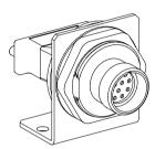
Mounting into an enclosure wall
