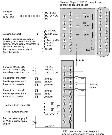
inputs (preset, enable, etc) and reflex outputs.
