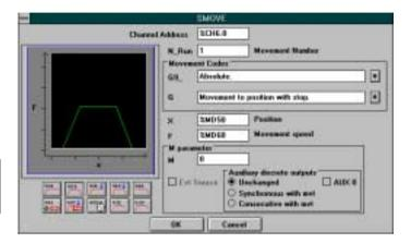
Screens for adjusting the axis parameters and setting up movements can also be accessed via PL7 Junior.
