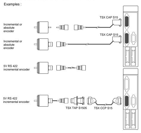
These accessories provide good signal and shielding continuity in adverse conditions. The encoder connection cables are generally offered by the encoder suppliers.
