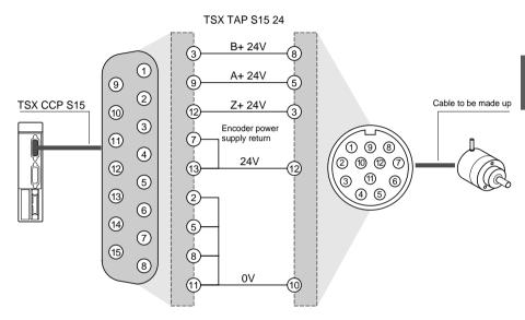
This type of connection is compatible with encoders with a 24V supply:
