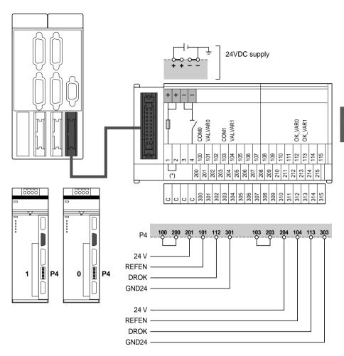
For direct connection use a TSX CDP 301 or 501 cable. See section 3.6-3.
