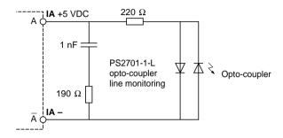
Inputs IA, IB and IZ used in RSS 422 are totally compatible with incremental encoder line drivers with RS 422 outputs and also with encoders with pushpull complementary outputs with a 5 V power supply. Line monitoring is performed on each output.
