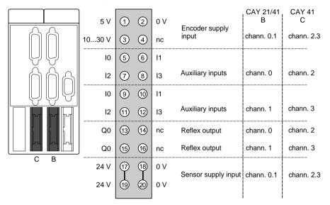
Channels 2 and 3 are assigned to the TSX CAY 41 module The auxiliary I/Os are assigned to the following functions:
