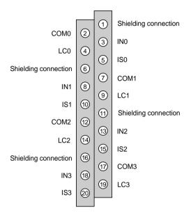
INx : +ve input channel x COMx : -ve input channel x ISx : +ve probe supply LCx : Line compensation
