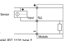
2-wire sensors and positive logic inputs (sink) IEC 1131 type 2.
