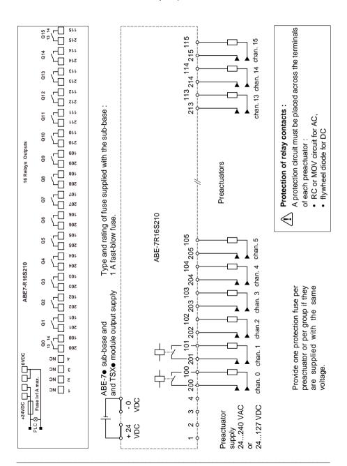
ABE-7R16S212 sub-base: 16 relay outputs, 1 "N/O", with distribution of 2 poles per group of 8 channels
