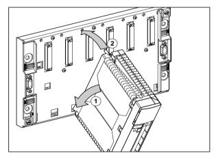
3 Fit the module firmly onto the rack by tightening the screw at the top of the module (3).
