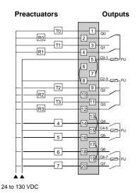
= strap 24 V must be connected when using 24 V AC or DC.
