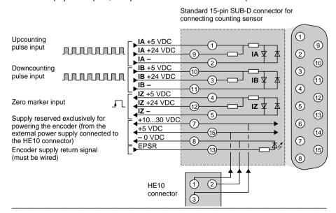
Use of two physical inputs with signals phase shifted by  $\pi/2$  (incremental encoder signals) with the possibility of multiplication by 1 or 4:
