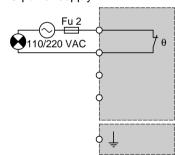
Note: when using several fan modules, the probe contacts will be placed in series.
