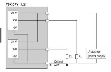
If there is a break in the supply cable segment between A and B, there is a risk of the RL actuators remaining energized. If possible, double the 0V supply connections for the module(s).
