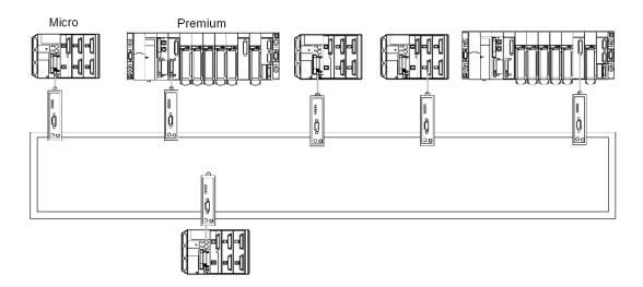
A large number of Schneider products which operate on the Fipway network can be connected to the OZD FIP G3 transceiver:
