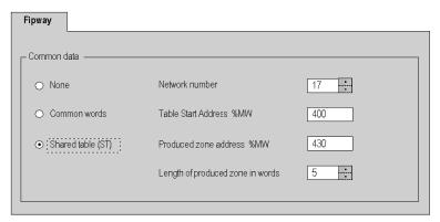
The area produced by the station begins with the address %MW430.
