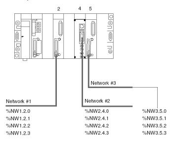
In a multi-network *(see EcoStruxure™ Control Expert, Operating Modes)* architecture, common words can be accessed through the network address of each module.
