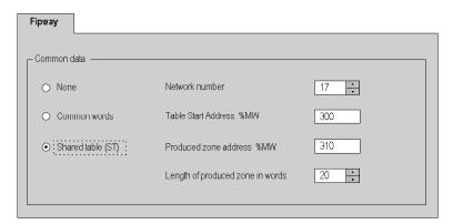
The area produced by the station begins with the address %MW310.
