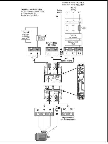
\* When using a 200V drive on a single phase supply, the live and neutral conductors can be connected to any of the AC connections on the drive.
