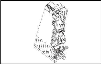
**NOTE** The size of the connecting cable between the encoder ground tab and the EMC bracket should be equal to the input cable.
