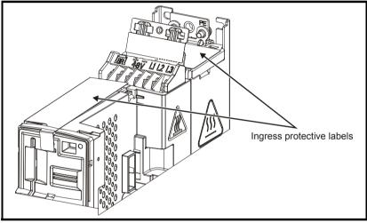
**NOTE** The ingress protective labels (shown in Figure 3-3 above) should remain in place while the drive is mounted, and until all the electrical wires have been connected. The labels should be removed before first power up.
