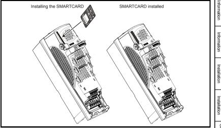
The SMARTCARD is located at the top of the module under the drive display (if installed) on the left-hand side.
