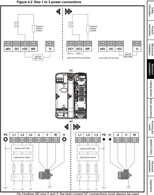
On Unidrive SP size 2 and 3, the high current DC connections must always be used when using a braking resistor, supplying the drive from DC (low voltage DC or high voltage DC) or using the drive in a parallel DC bus system. The low current DC connection is used to connect low voltage DC to the drive internal power supply and to connect the internal EMC filter.
