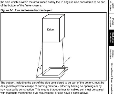
The bottom, including the part of the side considered to be part of the bottom, must be designed to prevent escape of burning material - either by having no openings or by having a baffle construction. This means that openings for cables etc. must be sealed with materials meeting the 5VB requirement, or else have a baffle above.
