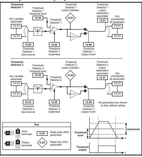
Figure 9-16 Menu 12 logic diagram
