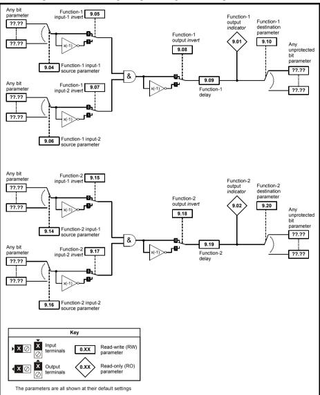
Figure 9-14 Menu 9 logic diagram: Programmable logic
