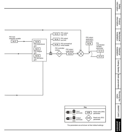
\*The PID controller is only controlled if Pr **14.16** is set to a non Pr **xx.00** and unprotected destination parameter.
