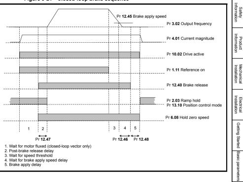
Figure 9-21 Closed-loop brake sequence
