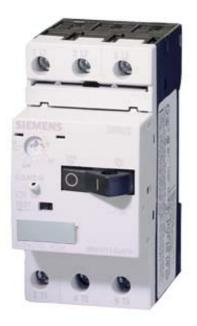
CIRCUIT-BREAKER SIZE S00, FOR MOTOR PROTECTION, CLASS 10, A-REL.1.8...2.5A, N-REL. 33A, SCREW TERMINAL, STANDARD SWITCHING CAPACITY
