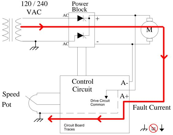
these terminals will effectively short out the power line through the circuit board traces. The Focus 3 Regenerative drives (**F3R**2C / **F3R**2E / **F3R**5C / **F3R**5E) are isolated from the power line and therefore, connections on TB2 can be tied to earth ground.
