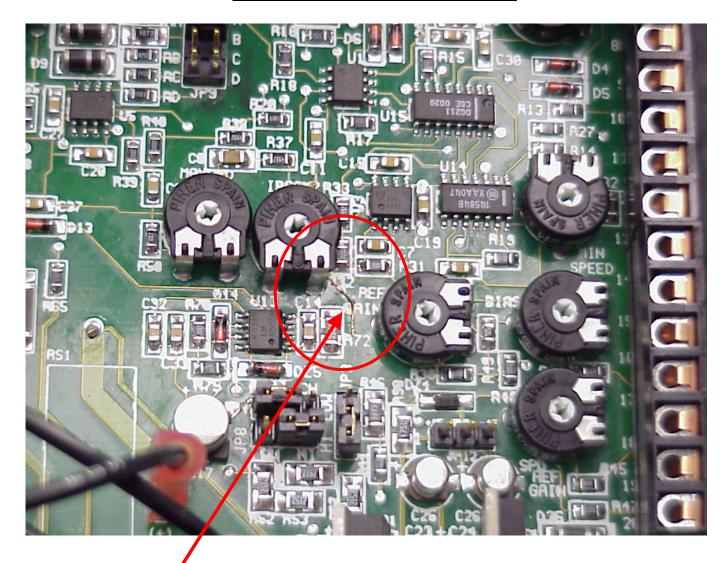
Typical Damaged circuit trace due To earth ground connection on Control terminal strip
