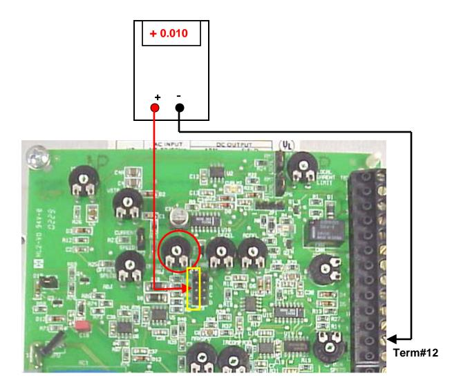
With power applied to the drive but NOT in run. Measure the dc voltage at JP9 (any of the free pins on the left side) with respect to signal common (terminal #12).
