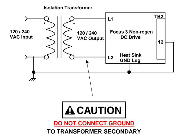
Transformer KVA = 1.5 x Rated Armature Current x 120 Vac (or 240)
