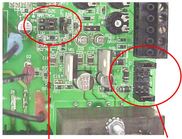
Photo shown jumpered for 120Vac input
