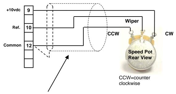
Cable should be 3 conductor with overall shield w/pot end tied off and dressed. Cable and pots are available from:
