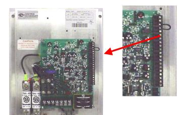
The Chassis Model has no operator devices connected to the drive control terminal strip. The only connections made are connections from terminal #3 to #4 which is required for three wire Start/Stop controls.
