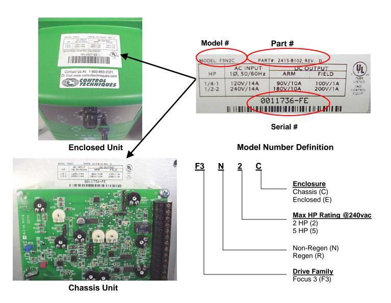
Always record the drive *Model Number*, *Part Number* and *Serial Number* for future warranty situations and spare parts. A good location to record these is on the **Start-up Guide Worksheet** on page #49.
