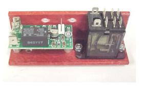
This Kit includes a magnetic contactor that can be mounted either in the Focus 3 enclosed unit or on the chassis mount unit. It provides a positive disconnect of the motor armature when the controller is stopped, preventing motor rotation in the event of SCR mis-fire due to line noise. This kit may also be required by local and/or National Electrical Codes. This kit also includes the DB (dynamic braking) poles, an auxiliary normally open contact and all connection wires.
