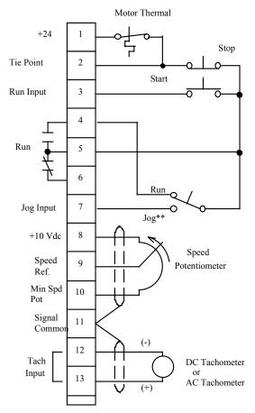
Note: Fwd / Rev switch connected to reversing board, not shown
