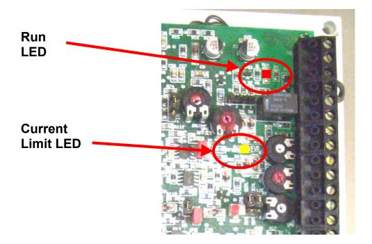
**Run LED** – This red led will illuminate any time the run relay is energised
