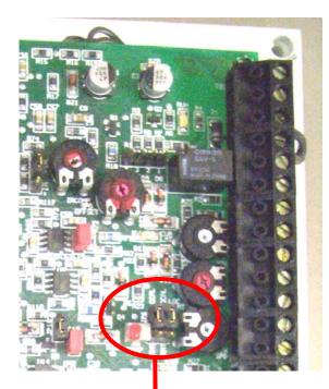
JP9 -- Max Output Current (100%) Removed - 2.7 A and less
