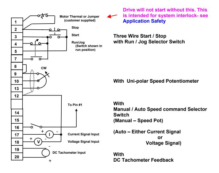
Shielded cable should be 3 conductor with overall shield w/pot end tied off and dressed. Cable and pots are available from Control Techniques Service Center @ 1-800-367-8067
