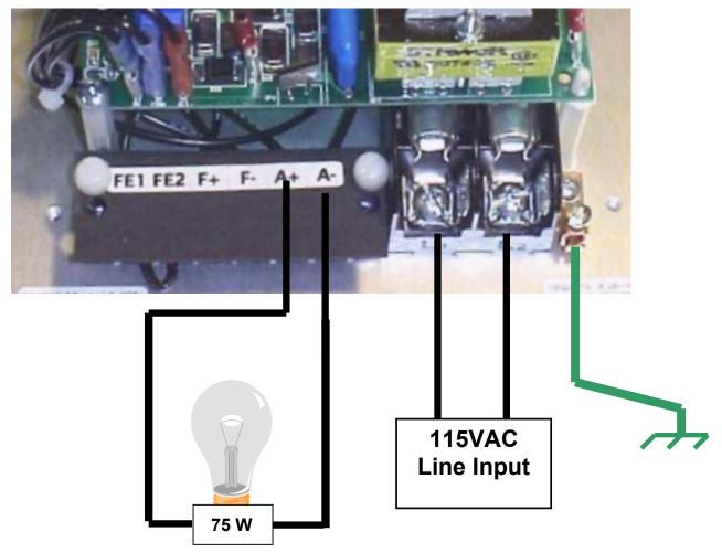
In order to test the Focus, one would need to setup the input for 115 Vac operation and for basic Armature Voltage feedback. The drive should also be set for the lowest current setting. Therefore before testing, one should record the settings before test so that they could be reset back after the test.
