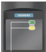
LEDs for indicating the drive state
