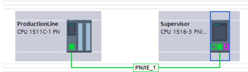
Figure 10-65 Example of assigning connection parameters in the network view
