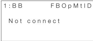
\*2. The following display will appear if a Feedback Option Module is connected but there is no Servomotor or encoder information in the Option Module
