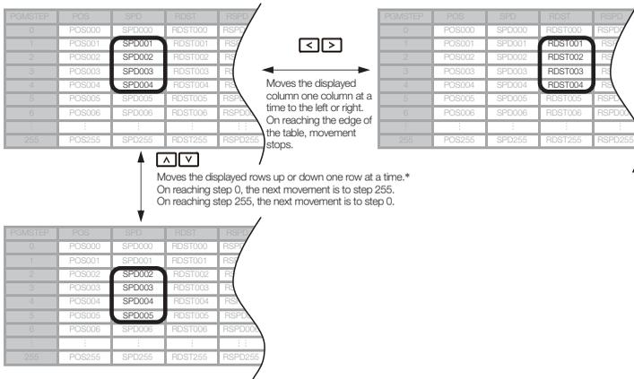
\* You can move 4 rows at a time by holding down the or key. By using the key at the same time as these keys, you can move 30 rows at a time.
