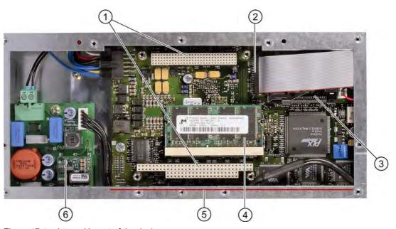
Figure 17-1 Internal layout of the device
