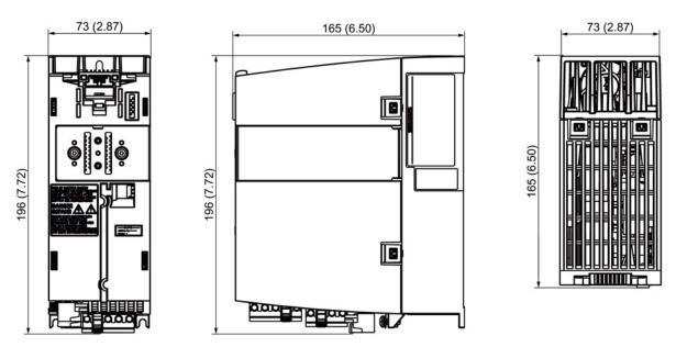
Figure 4-7 Dimension drawing of PM240-2 Power Modules, frame size FSA, all data in mm (inches)
