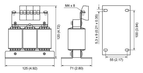
Figure 3-9 Dimensional drawing of line reactors, PM240-2 frame size FSA, 0.55 ... 1.1 kW, all dimensions in mm and (inch)
