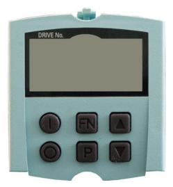
Figure 7-23 Basic Operator Panel BOP20
