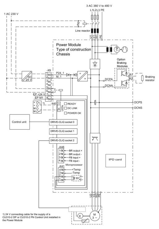
Figure 4-59 Connection example: Power Module chassis
