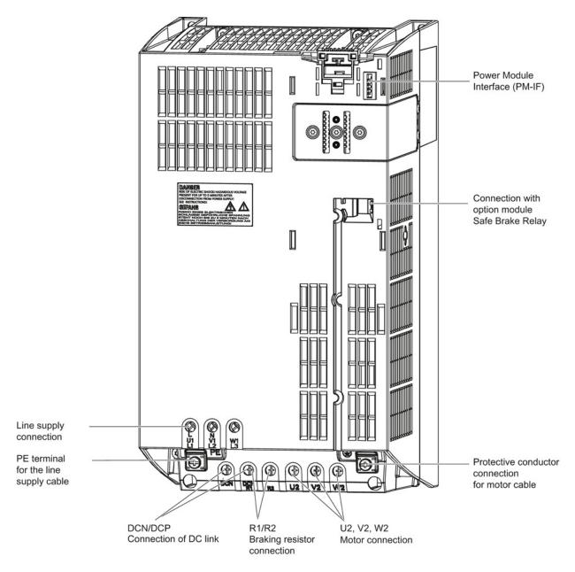
Figure 4-30 PM340, frame size FSC
