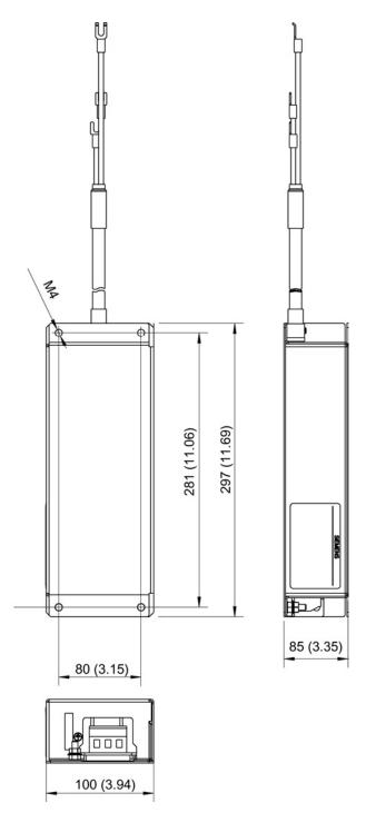
Figure 3-4 Dimension drawing of the line filter, Power Module PM240-2 frame size FSB, all data in mm (inches)
