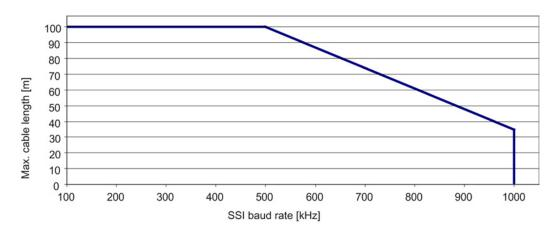
Figure 7-4 Maximum cable lengths depending on the SSI baud rate for SSI encoders
