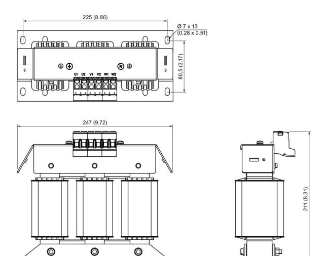
Figure 6-2 Dimension drawing of motor reactor, PM240-2 frame size FSB, all data in mm (inches)
