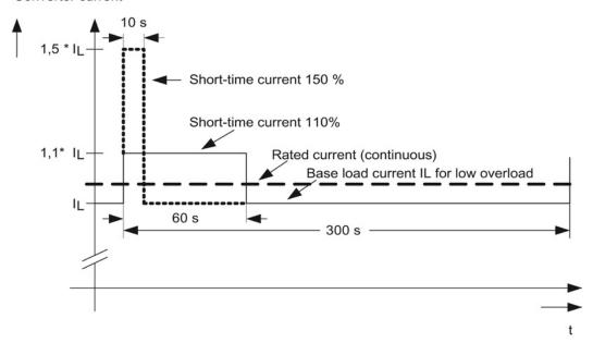
Figure 4-64 Characteristic: Low overload
