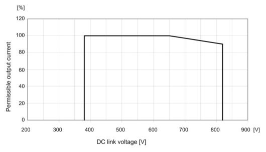
Figure 4-27 Current derating as a function of the DC-link voltage
