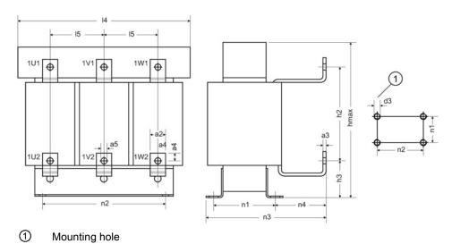
Figure 3-16 Dimension drawing, line reactors
