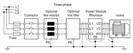
Figure 3-1 Example of a Blocksize line connection
