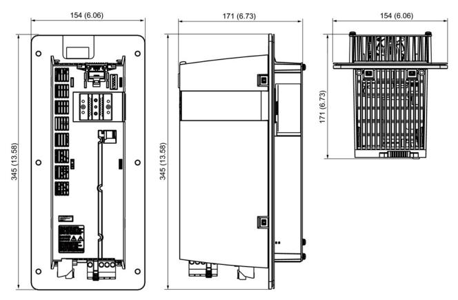
Figure 4-11 Dimension drawing of PM240-2 Push Through Power Modules, frame size FSB, all data in mm (inches)
