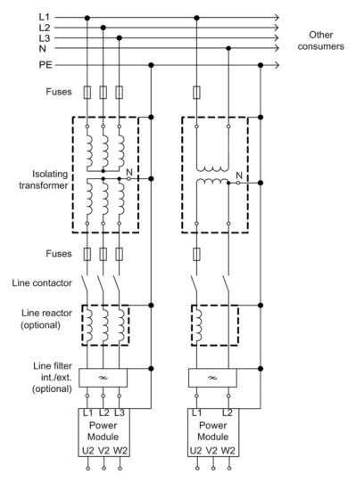
Figure 3-33 Isolating transformer
