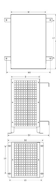
Figure 5-7 Dimension drawing of braking resistor for PM340, frame sizes FSC / FSD / FSE / FSF
