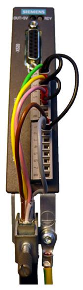
Figure 8-12 Photo of connection example 2: SMC30, 30 mm wide
