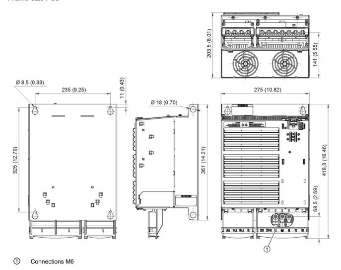
Figure 4-38 Dimension drawing, PM340 Power Module, frame size FSD (without integrated line filter); all dimensions in mm and (inches)
