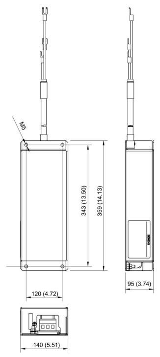
Figure 3-5 Dimension drawing of the line filter, Power Module PM240-2 frame size FSC, all data in mm (inches)
