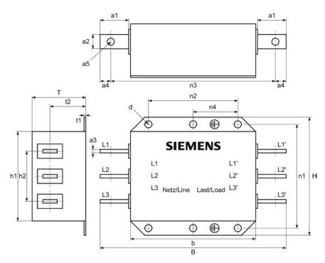
Figure 3-7 Dimension drawing, line filter
