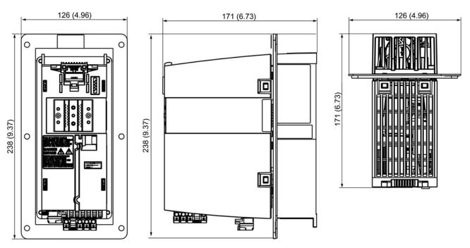
Figure 4-10 Dimension drawing of PM240-2 Push Through Power Modules, frame size FSA, all data in mm (inches)
