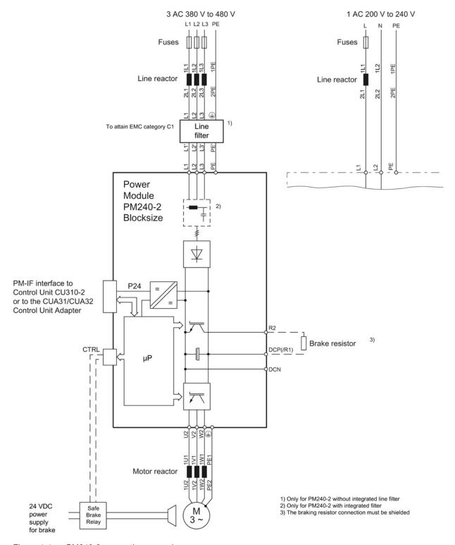
Figure 4-4 PM240-2 connection example
