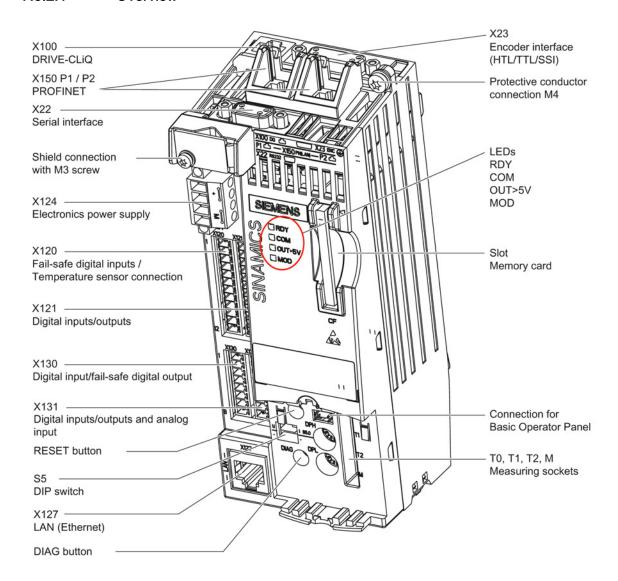
Figure 7-2 CU310-2 PN overview of interfaces
