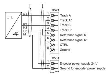
Figure 8-11 Connection example 2: HTL encoder, unipolar, with reference signal<sup>1)</sup>
