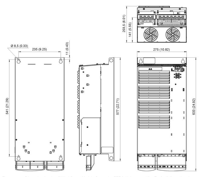
Figure 4-41 Dimension drawing, PM340 Power Module, frame size FSE (with integrated line filter); all dimensions in mm and (inches)
