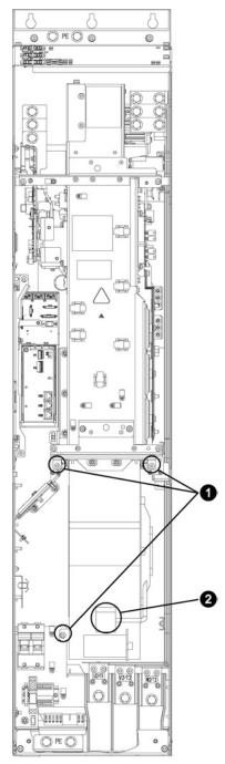
Figure 11-12 Replacing the fan, Power Module, frame size GX
