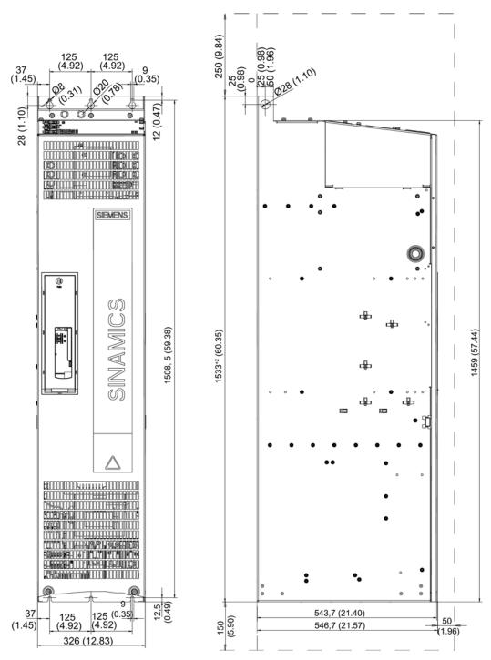
Figure 4-61 Dimension drawing Power Module, frame size GX
