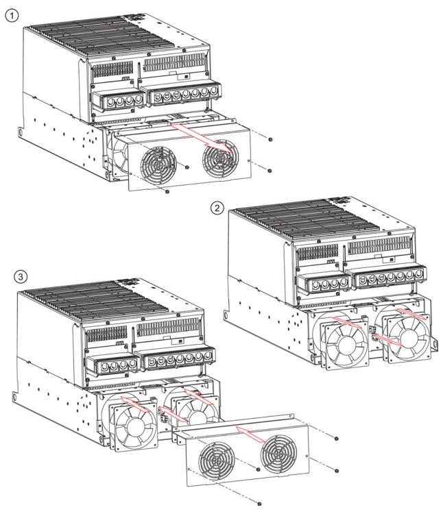
Figure 11-5 PM340 fan replacement, frame size FSF
