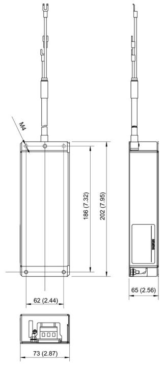
Figure 3-3 Dimension drawing of the line filter, Power Module PM240-2 frame size FSA, all data in mm (inches)
