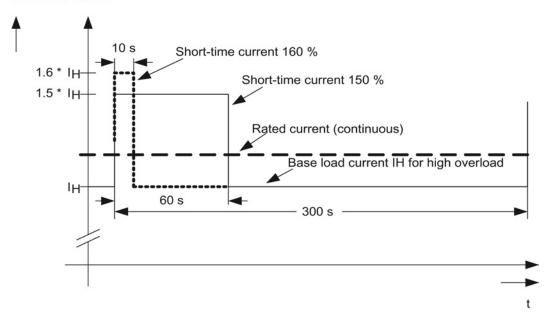
Figure 4-65 Characteristic: High overload
