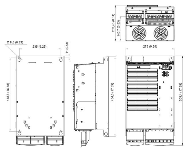
Figure 4-39 Dimension drawing, PM340 Power Module, frame size FSD (with integrated line filter); all dimensions in mm and (inches)
