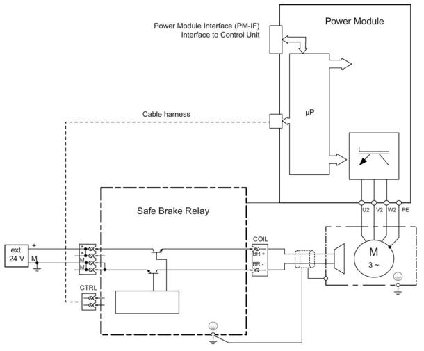
Figure 8-21 Safe Brake Relay connection example
