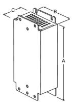
Figure 6-4 Dimension drawing motor reactor, PM340 frame size FSA
