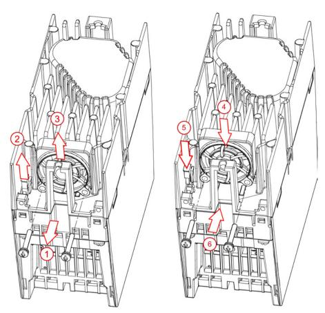
Figure 11-2 PM340 fan replacement, frame size FSA
