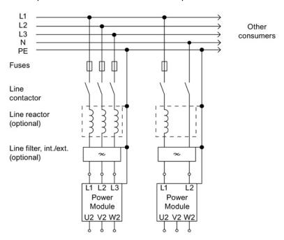
Figure 3-30 Direct operation on the line supply
