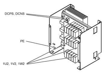
Figure 6-16 Interface overview, Voltage Peak Limiter, type 1
