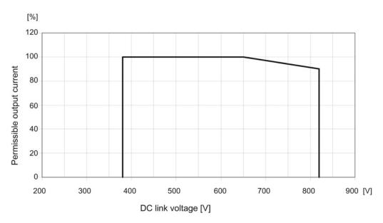
Figure 4-56 Current derating as a function of the DC-link voltage
