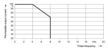
Figure 4-52 Frame size FSF: Output current as a function of the pulse frequency
