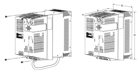
Figure 6-12 Mounting Power Modules and motor reactors, frame sizes FSB / FSC
