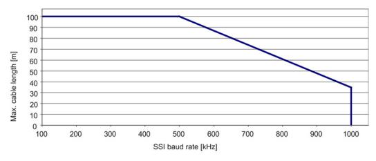
Figure 8-8 Maximum cable lengths depending on the SSI baud rate for SSI encoders
