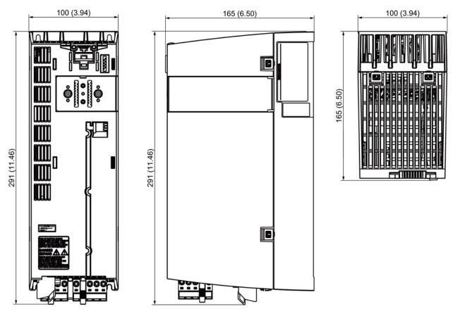
Figure 4-8 Dimension drawing of PM240-2 Power Modules, frame size FSB, all data in mm (inches)
