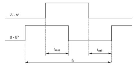
Figure 8-18 Signal characteristic of track A and track B between two edges: Time between two edges with pulse encoders
