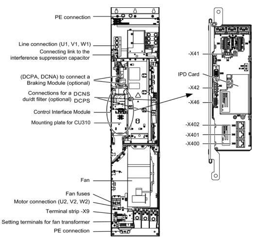
Figure 4-58 Power Module, frame size GX
