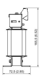
Figure 6-1 Dimension drawing of motor reactor, PM240-2 frame size FSA, all data in mm (inches)
