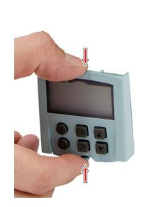
2. Press the latching cams on the BOP20 together simultaneously and push the BOP20 straight into the housing of the CU310-2 until you hear it latch into position.
