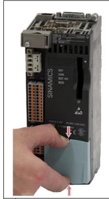
To remove the blanking cover, press the latching cams of the cover together simultaneously and pull the cover straight out.
