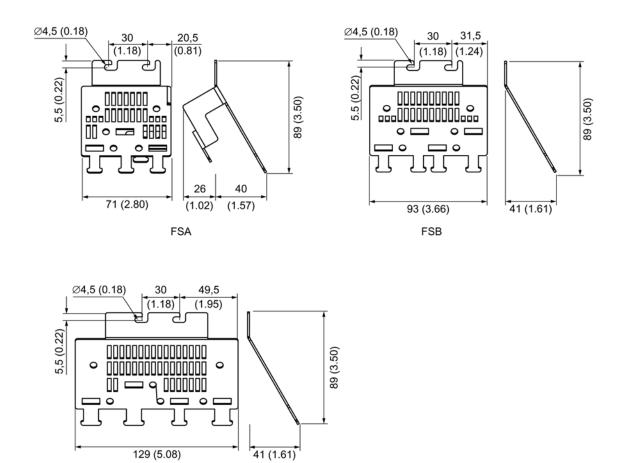
Figure 4-13 Dimension drawing of shield connection plates for PM240-2 Power Modules, frame size FSA to FSC, all data in mm (inches)
