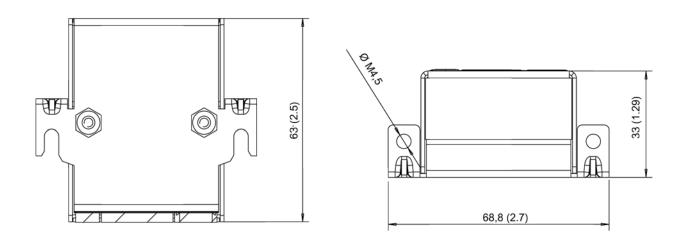
Figure 8-22 Dimension drawing of Safe Brake Relay, all data in mm and (inches)
