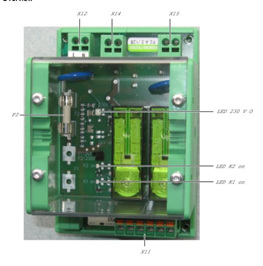
Figure 8-25 Interface overview, Safe Brake Adapter 230 VAC
