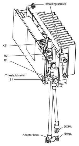
Figure 5-9 Braking Module for Power Module, frame size FX
