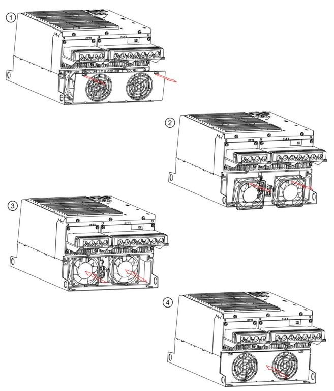
Figure 11-4 PM340 fan replacement, frame sizes FSD/FSE
