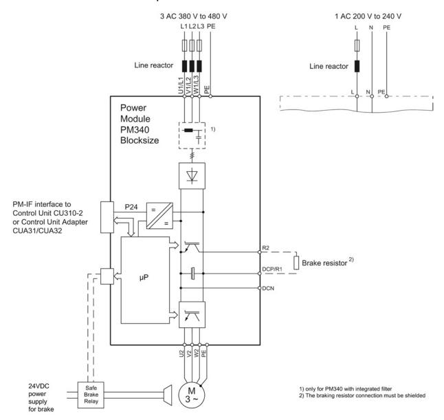
Figure 4-34 PM340 connection example
