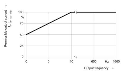
Figure 4-66 Output current as a function of the output frequency
