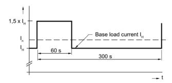
Figure 4-49 Duty cycle with 60 s overload with a duty cycle duration of 300 s
