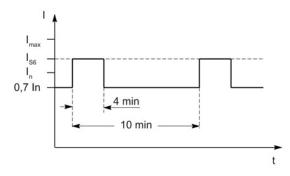
Figure 4-47 S6 duty cycle with initial load (for servo drives)
