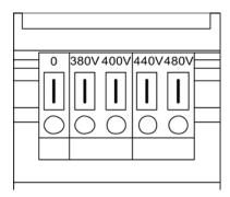
Figure 4-62 Setting terminals for the fan transformers
