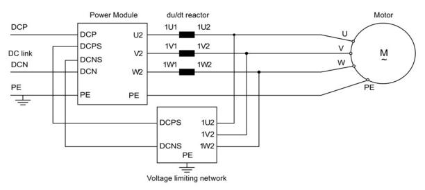
Figure 6-18 Connecting the dV/dt filter plus Voltage Peak Limiter
