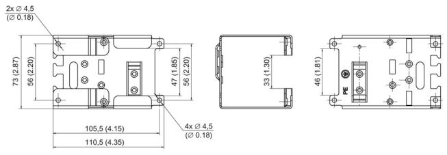
Figure 9-16 Dimension drawing of the shield connection kit for PM340 Power Modules, frame size FSA, all data in mm (inches)
