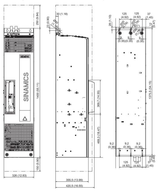
Figure 4-60 Dimension drawing Power Module, frame size FX
