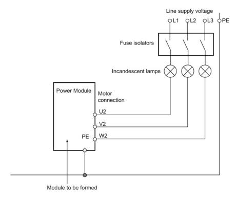
Figure 11-13 Forming circuit for 3-ph AC Power Modules with incandescent lamps
