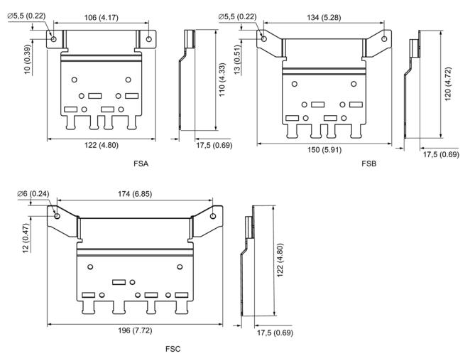
Figure 4-14 Dimension drawing of shield connection plates for PM240-2 Push Through Power Modules, frame size FSA to FSC, all data in mm (inches)
