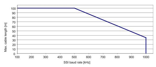
Figure 8-16 Maximum cable lengths depending on the SSI baud rate for SSI encoders
