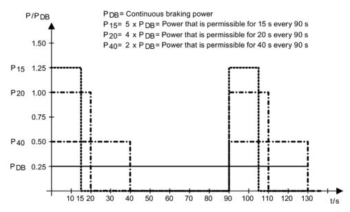
Figure 5-14 Duty cycle for braking resistors
