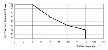
Figure 4-51 Frame sizes FSA to FSE: Output current as a function of the pulse frequency
