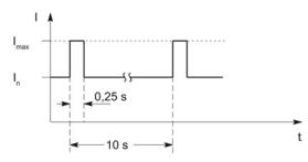
Figure 4-17 Duty cycle with initial load (for servo drives)
