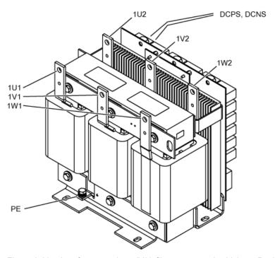
Figure 6-23 Interface overview, dV/dt filter compact plus Voltage Peak Limiter, type 2
