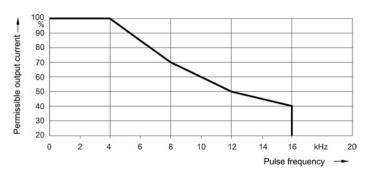
Figure 4-23 Output current as a function of the pulse frequency
