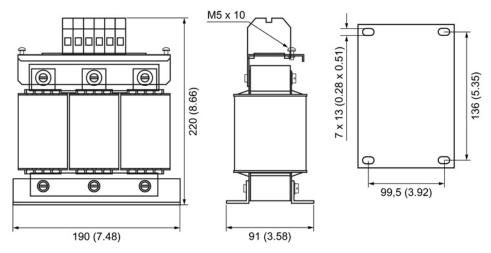
Figure 3-12 Dimensional drawing of line reactors, PM240-2, frame size FSC, 11 ... 15 kW, all dimensions in mm and (inch)
