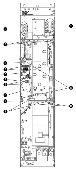
Figure 11-8 Replacing the Powerblock, Power Module, frame size GX
