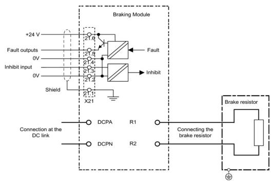
Figure 5-11 Example connection of Braking Module
