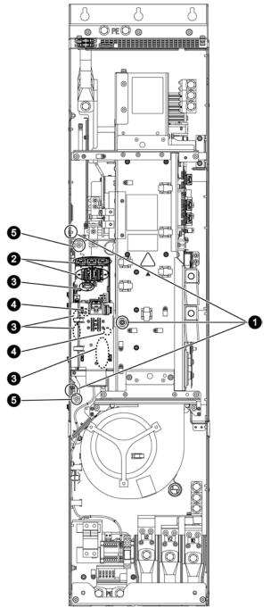
Figure 11-9 Replacing the Control Interface Module, Power Module, frame size FX
