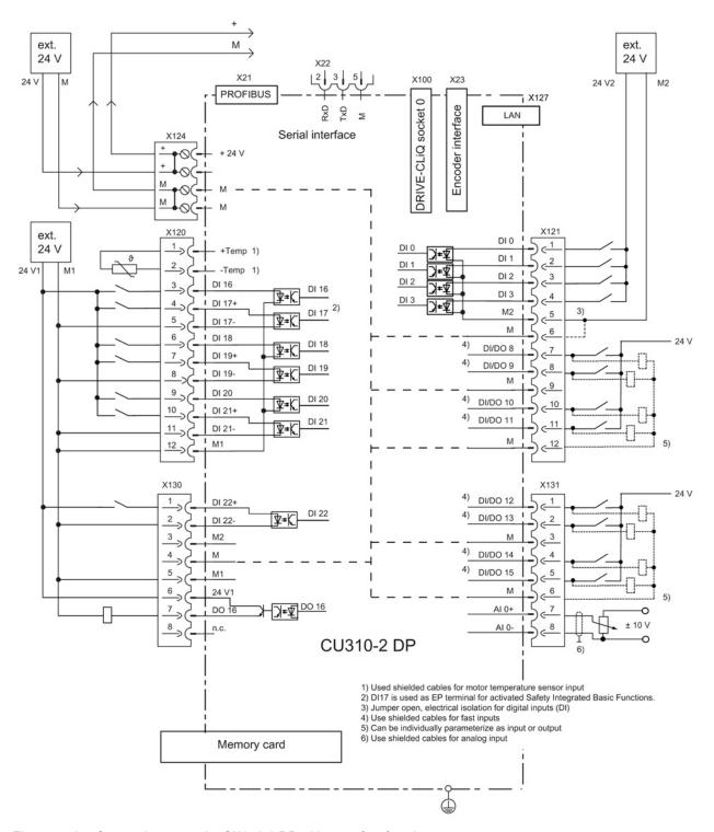
Figure 7-13 Connection example, CU310-2 DP without safety function
