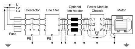
Figure 3-2 Example of a chassis line connection
