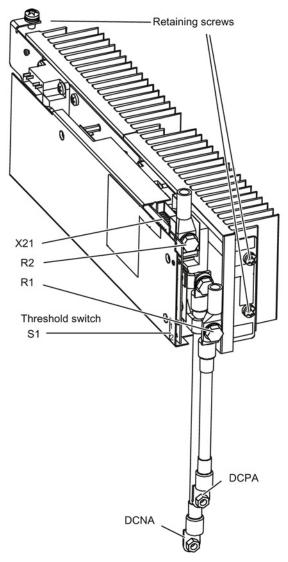
Figure 5-10 Braking Module for Power Module, frame size GX
