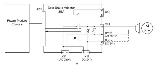
Figure 8-26 Connection example for a Safe Brake Adapter
