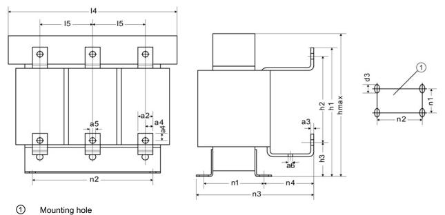
Figure 6-19 Dimension drawing, dV/dt reactor
