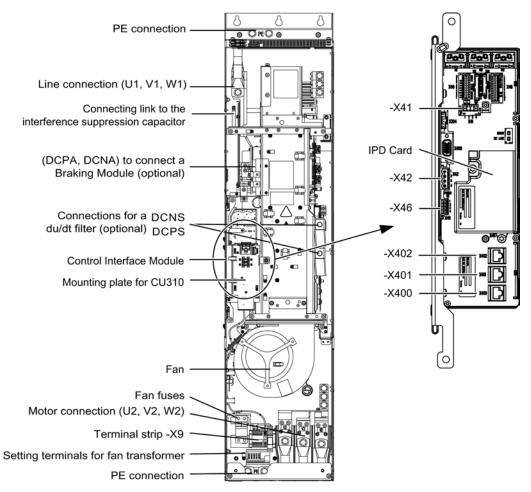
Figure 4-57 Power Module, frame size FX
