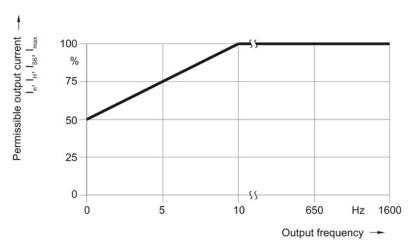
Figure 4-26 Output current as a function of the output frequency
