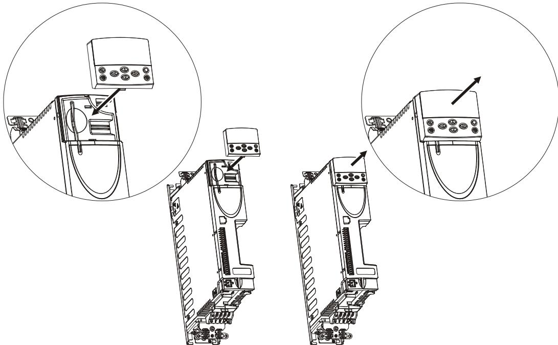
To fit, align the SP0 / SPz Keypad and press gently in the direction shown until it clicks into position.
