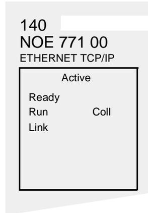
If the **Coll** LED is flashing, the module is reporting collisions on the Ethernet network. While such collisions are normal, the frequency of the flashes is an indication of the volume of traffic on the network. The flashes may be so frequent that the LED appears to be shining steadily. Heavy traffic will slow communications. If response time is important to your application, you should consider segmenting your network to reduce the frequency of collisions.
