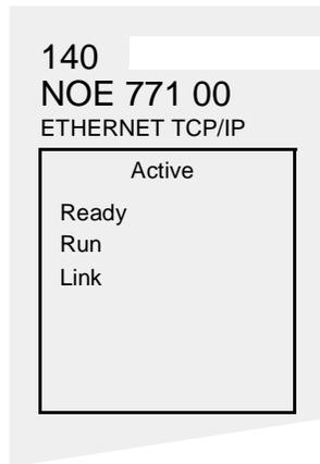
The **Run** indicator will be solid. The **Coll** LED may flash, indicating that collisions are occurring on the Ethernet network. Such collisions are normal.
