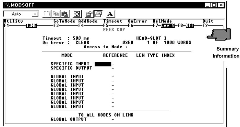
The cursor is initially in the Head Slot field. If you are not editing an initial template you may press the Esc key which re-positions the cursor to the SPECIFIC INPUT field. To traverse the Heads and Nodes you can re-display the Add Node select box from the main Menu line.
