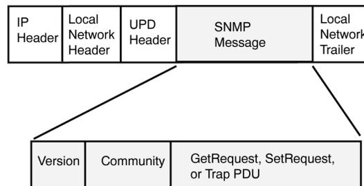
The PDUs within the SNMP initiate the communication between the manager and the agents. The SNMP installed on your NOE 771 00 module uses three PDUs:
