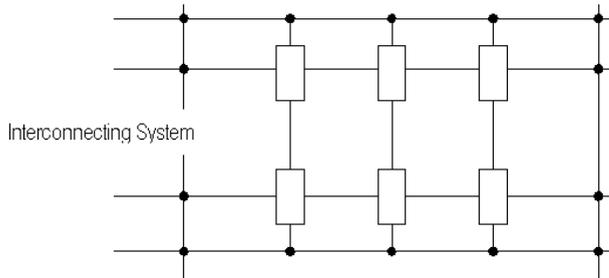
This creates a perfectly meshed system. The connections are arranged between the devices ground, cable runs, existing or under construction metal structures etc. Shielding, filtering devices, return conductors, etc. are directly connected to the ground cable.
