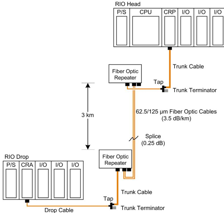
The specified power loss budget for a link using this optical cable is 11 dB. We know that the cable's attenuation over 3 km is  $3.5 \text{ dB/km} \times 3 = 10.5 \text{ dB}$ , and we are given an attenuation of 0.25 dB for the cable splice. Thus, we have a total optical power loss of 10.75 dB on the fiber optic link, which is under power loss budget and therefore conform to the expectations.
