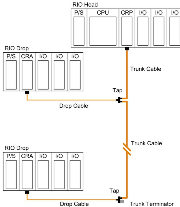
To avoid attenuation, noise and/or distant ground in case of a long trunk cable, it can be useful to install fiber optic repeaters.
