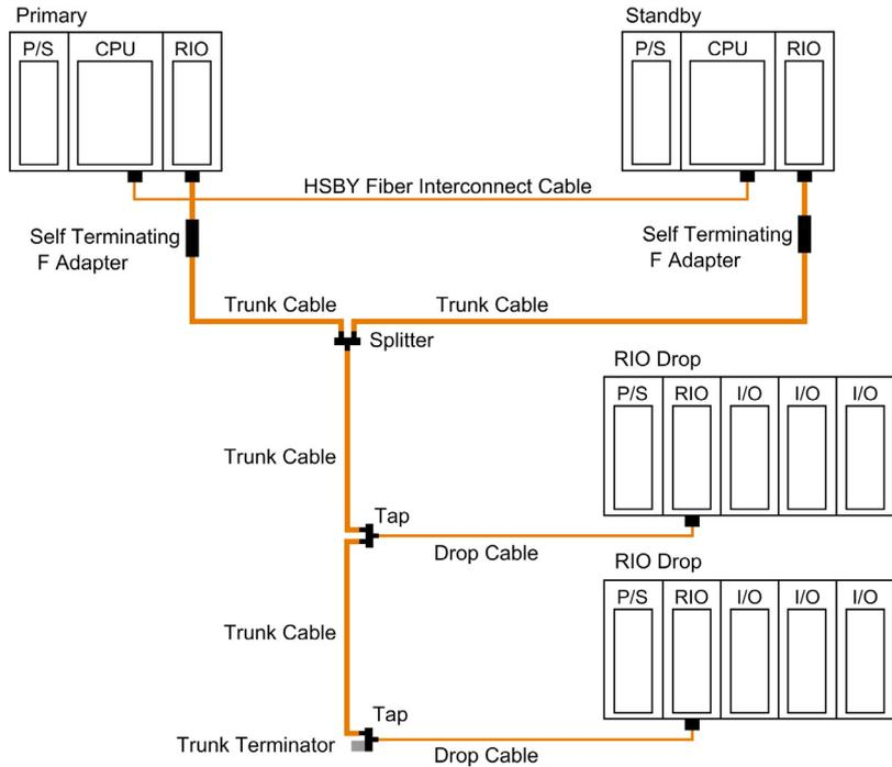
To avoid noise, attenuation and/or distant ground in case of long distances between both RIO heads of the HSBY system, it can be useful to install fiber optic repeaters.
