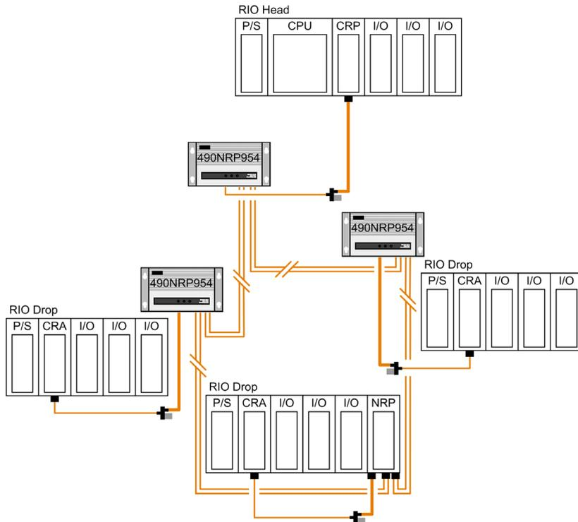
**NOTE:** Depending on the architecture topology, some restrictions may appear on the diagnostic relay features (*see page 26*) when 140 NRP 954 00 and 490NRP954 fiber optic repeaters are connected together.
