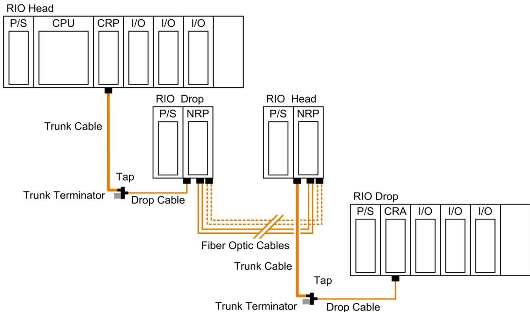
Each 140 NRP 954 0• can be placed on the racks where the RIO head and RIO drop modules are located.
