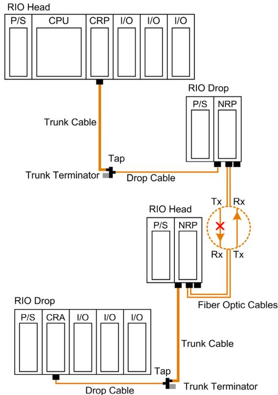
A break in the receive line as shown above will deprive the PLC of input data. Under ordinary circumstances, the PLC will continue to drive outputs via the intact transmit line. This could lead to outputs turning ON or OFF due to invalid (INPUT STATE: 0) input data.
