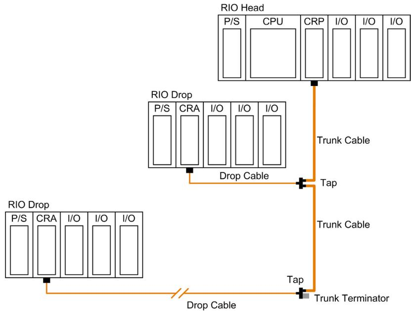
To avoid attenuation, noise and/or distant ground in case of a long drop cable, it can be useful to install fiber optic repeaters.
