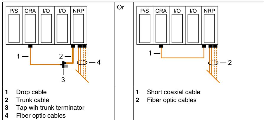
The short coaxial cable is a RG-6 cable fitted with type F female connectors. The maximum length of this cable is 30 cm (11.8 in.).
