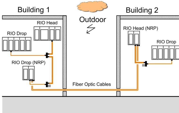
If this is not possible because of the system or construction specific reasons the best way to ensure that everything works properly is to maintain good equipotentiality between equipments using equipotential conductor.
