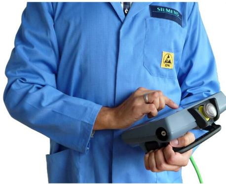
When holding the Mobile Panel as shown, you can, for example, perform movements in the fail-safe automation system during setup mode.
