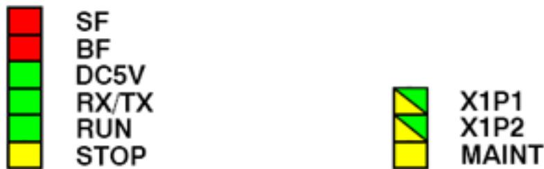
Figure 4-1 LEDs of the CP 343-1 Lean CX10
