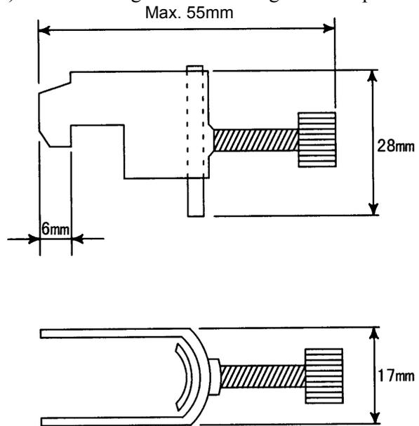
Fig.7.3.4(e) Outer drawings of metal fittings for clamp
