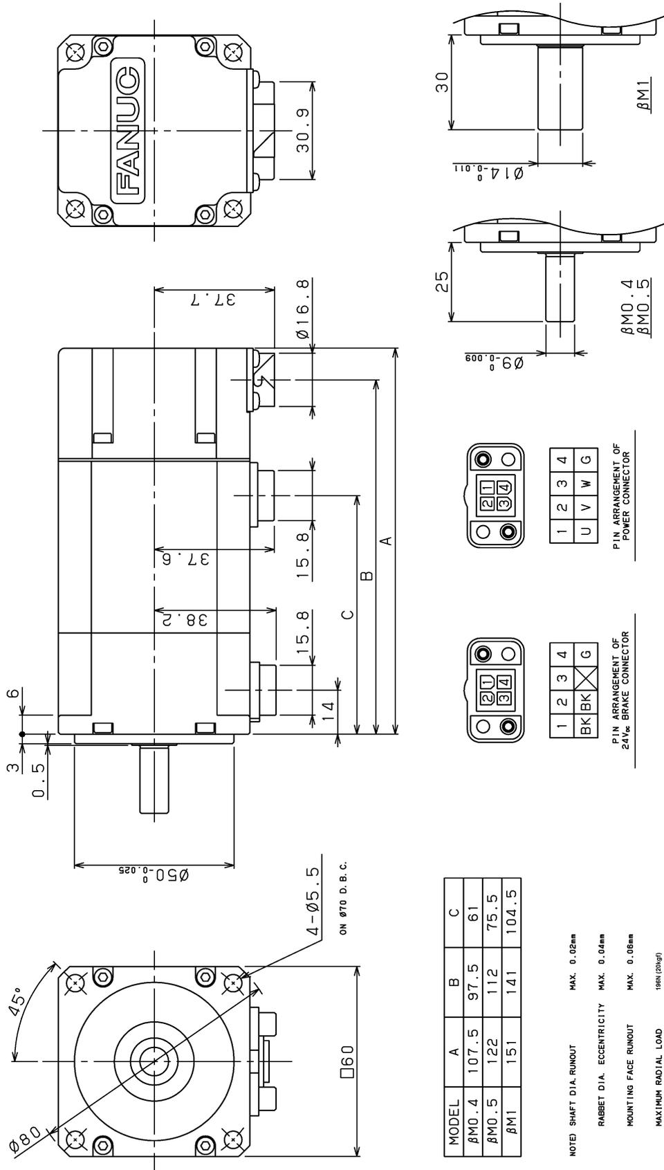
**Fig.2.4(f) Models  $\beta$ M0.4 and  $\beta$ M0.5: Shaft option**
