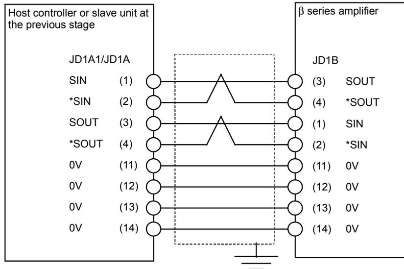
Details of connection of cable K20 (when a connection is made with the slave unit at the next stage)
