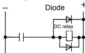
Use a diode which can withstand a voltage up to two times the applied voltage and a current up to two times the applied current.
