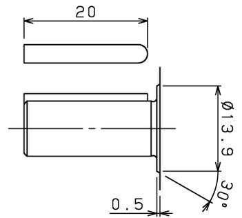
**Fig.2.4(g) Model  $\beta$ M1: Shaft option**
