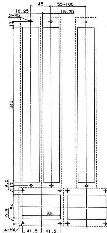
When three units of forced air cooling type are installed in parallel (The fan adapter (A06B-6078-K002) is used.)
