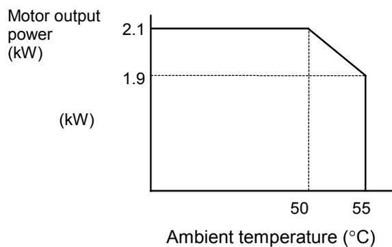
Derating curve of motor output
