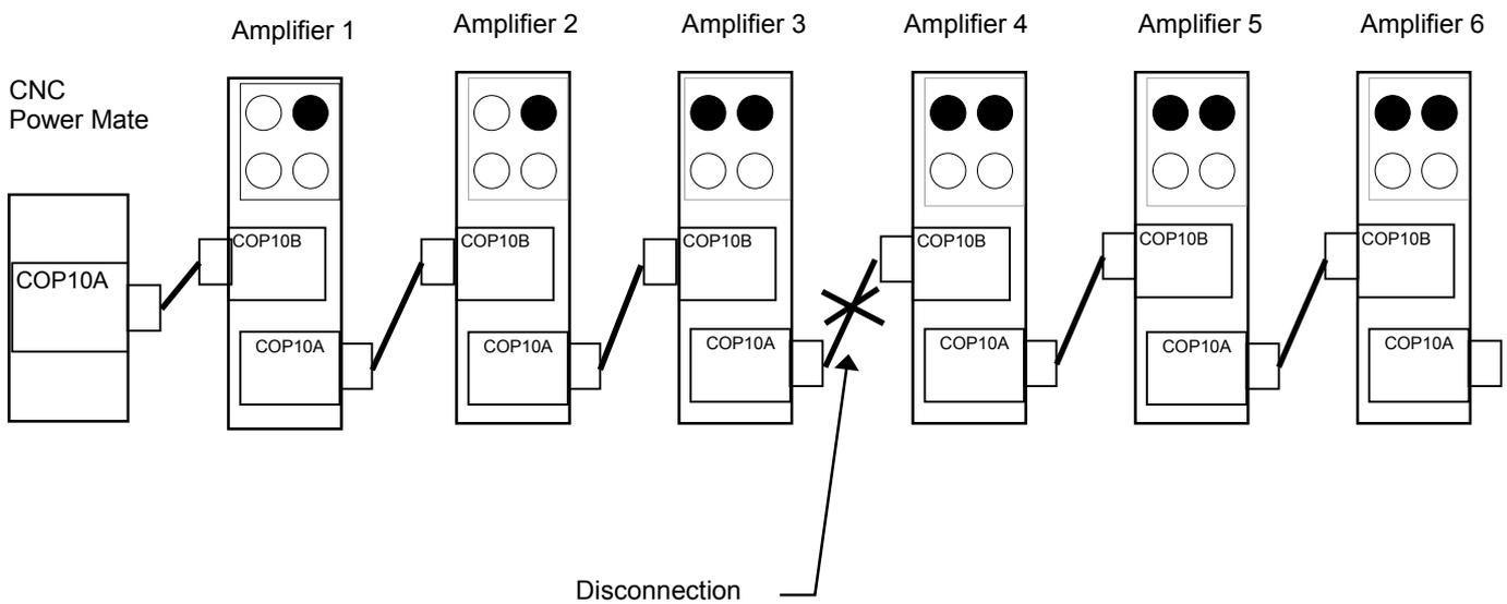
When the optical cable connecting the third  $\beta$  amplifier with the fourth  $\beta$  amplifier, the "ALM" LEDs on the third and subsequent amplifiers are turned on, and the "LINK" LEDs and the "READY" LEDs are turned off.
