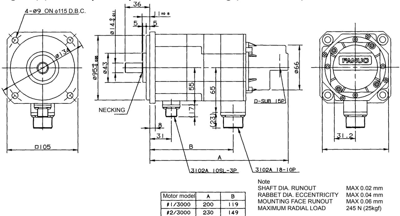
**Fig.2.4(c) Models  $\beta 1$  and  $\beta 2$  : Shaft option**
