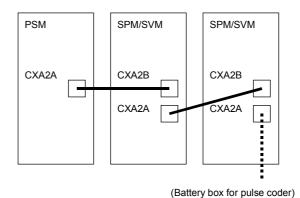
(b) The interface cable between CXA2B of the power supply module and CXA2A of the SVM or SPM is defective.
