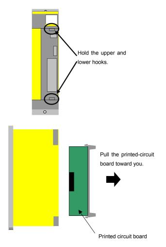
To insert the printed-circuit board, reverse the above procedure. Ensure that the upper and lower hooks snap into the housing. If the printed-circuit board is not inserted completely, the housing remains lifted. Pull out the printed-circuit board and insert it again. B-65285EN/03 TROUBLESHOOTING 4.HOW TO REPLACE THE FUSES AND PRINTED CIRCUIT BOARDS
