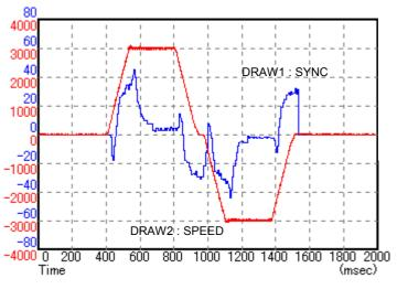
DRAW1 : SYNC (synchronization error) \*1 DRAW2 : SPEED (motor speed)
