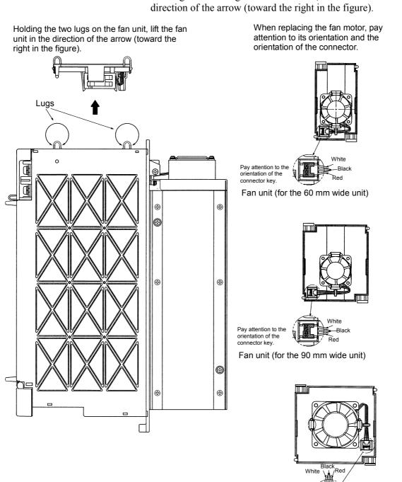
1 Holding the two lugs on the fan unit, lift the fan unit in the direction of the arrow (toward the right in the figure).
