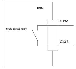
(5) The PSM, SVM, or SPM is defective.  $\rightarrow$  Replace the defective module.
