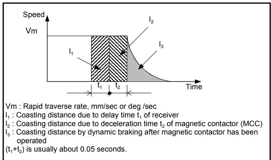
$$\text{Coasting distance due} = V_m \times (t_2 + t_2) + (J_m + J_L) \times (A \times N_o + B \times N_o^3) \times L$$
