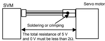
[Case 2] Sheath diameter of exceeds  $\phi 8$ .
