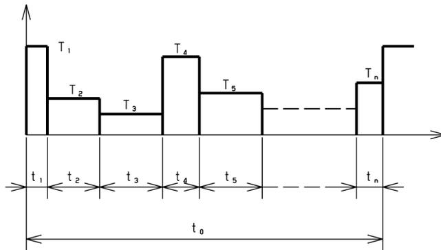
$$T_{rms} = \sqrt{\frac{T_1^2 t_1 + T_2^2 t_2 + T_3^2 t_3 + \dots + T_n^2 t_n}{t_0}}$$
