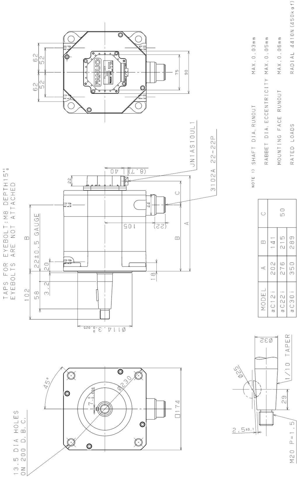
Fig.2.3(e) Models  $\alpha$ C12i,  $\alpha$ C22i, and  $\alpha$ C30i (with brake)
