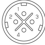
Connections: 1=BK, 2=BK, 3=NC(Not Connected), 4=GND<sup>(Note)</sup>
