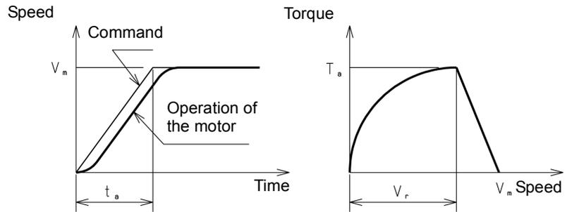
$$T_a = V_m \times 2\pi \times \frac{1}{t_a} \times J_M \times (1 - e^{-k_s \cdot t_a})$$
