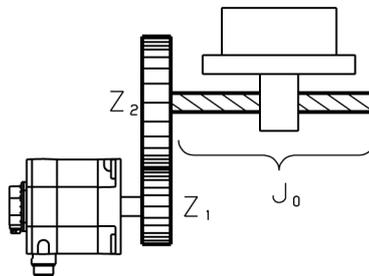
The inertia applied to the motor shaft by inertia  $J_0$  is calculated as follows:
