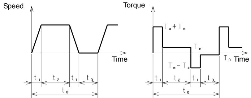
From the time-torque graph, obtain the root-mean-square value of torques applied to the motor during the single operation cycle. Check whether the value is smaller than or equal to the torque at stall (condition 3).
