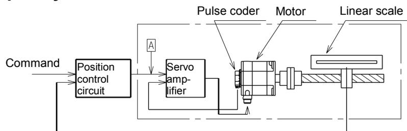
This method is shown in the figure above by block diagram. The response of this control system is determined by the adjustment value (position loop gain) of the position control circuit. In other words, the position loop gain is determined by the specified response time of the control system. In the diagram above, the section enclosed by the broken line is called the velocity loop.
