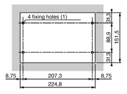
(1) The diameter of the fixing holes must be sufficient to take M6 screws.
