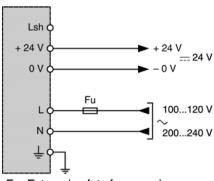
Fu=External safety fuse on phase (Fu): 250V 4A time delay
