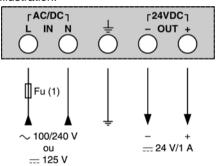
(1) External protection fuse on phase: 1A time delay 250V if single supply block.
