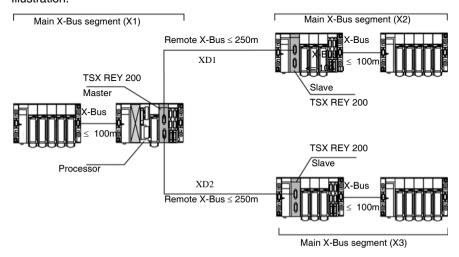
Taking this into account, the maximum distance possible between the processor and the remote modules is 350 meters.
