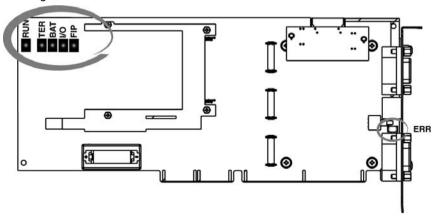
Due to the small amount of space available on the shield, only the ERR LED is visible when the PC housing the processor is closed.
