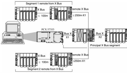
Station with extendable racks: 8 racks 12 positions or, 16 racks 4, 6 or 8 positions, two possible remotes,
