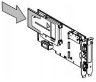
**Note:** if the program in the PCMCIA memory cartridge contains the **RUN AUTO** option, the processor will automatically restart in RUN mode after the cartridge is inserted and the PC is turned on.
