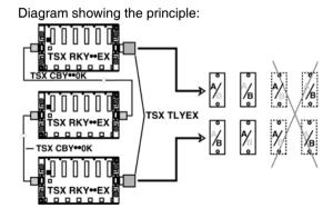
Positioning on a PLC station containing a single TSX RKY..EX extendable rack Diagram showing the principle:
