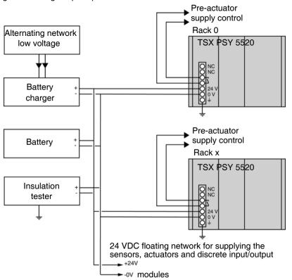
**Note:** a device can continually measure the level of insulation of the 24 VDC (or 48 VDC) in relation to the ground, and can give an alert when the level of insulation is abnormally low.
