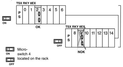
**Note:** If two racks are declared at address 0, the rack supporting the "high" address modules cannot receive a slave extension module.
