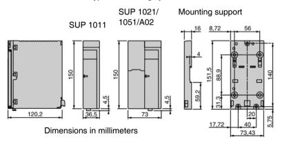
TSX SUP 1011/1021/1051/A02 power supply modules can be mounted in different ways:
