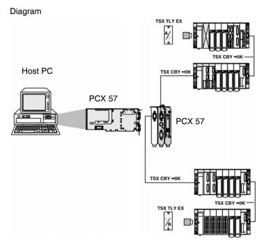
**Note:** in this example, as the PCX 57 processor is no longer integrated at the start of the line, the **TSX TLY EX A/** and **/B** line terminators must be installed on each of the racks situated at the end of the lines.
