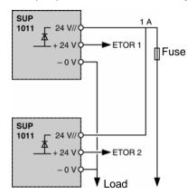
Discrete inputs 1 and 2 on the PLC indicate the failure of one or other of the power supplies.
