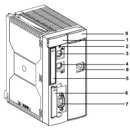
Double format processor with on-board Ethernet: TSX P57 2623/2823/3623/3623A/4823/4823A
