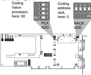
Position of the RACK ADD micro-switches in relation to the rack address:
