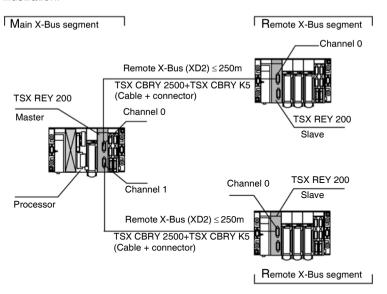
**Note:** Each X-Bus segment must have a A/ and B/ line terminator (See *Line terminator TSX TLYEX, p. 105*)at each end.
