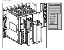
If there is a power outage while the battery is being changed, the processor ensures the RAM memory is saved, as it has its own offline independent save function.
