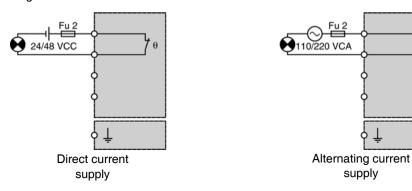
**Note:** If several ventilation modules are used, the probe contacts are set up in series.
