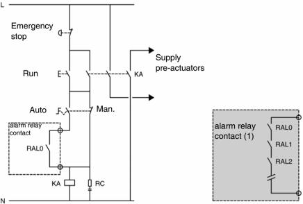
KA: contact controlled by alarm relay from supply module in AUTO run mode.
