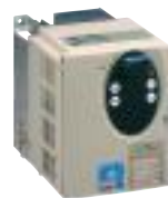
Lexium 05 drives from 4 A to 25 A ■ Lexium 05 operates in either torque or speed control mode by means of its \pm 10 V analog interface. Its encoder interface also performs the function of an electronic gearbox.
