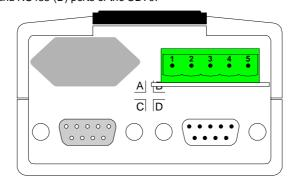
The pin connections for the DeviceNet connector are given in the table below. (Pins are numbered 1 to 5 from left to right on the above diagrams.)
