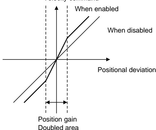
Fig. 4.8.1 (a) Position gain switching
