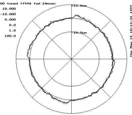
**Fig. 3.4.3 (d) Effect of velocity loop gain****Velocity loop gain: 300%****Advanced preview feed-forward coefficient: 99%****FAD time constant: 24 ms (linear type)**
