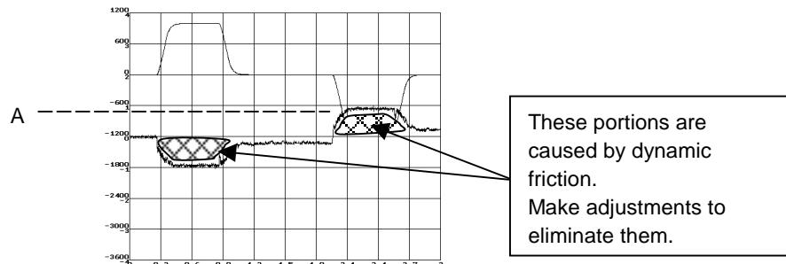
First, read the estimated disturbance value at a constant rotation speed of 1000 rpm. Set the dynamic friction compensation value parameter according to the read value.
