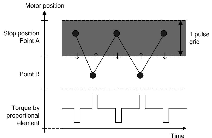
**Fig. 4.4.4 (a) N pulse suppression function disabled (Torque due to the proportional term keeps up, leading to vibration.)**
