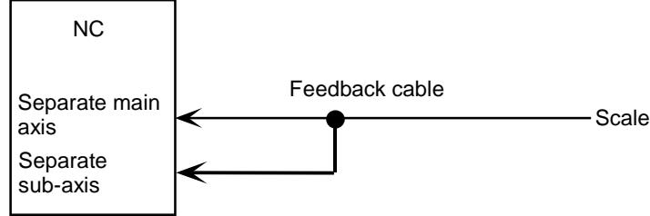
**Fig. 4.17.8 (b) Cable on the scale side when the position feedback switching function is used (full-closed loop)**
