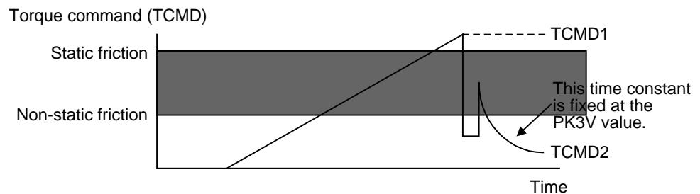
**Fig. 4.7 (f) Torque command (when overshoot is used)**
