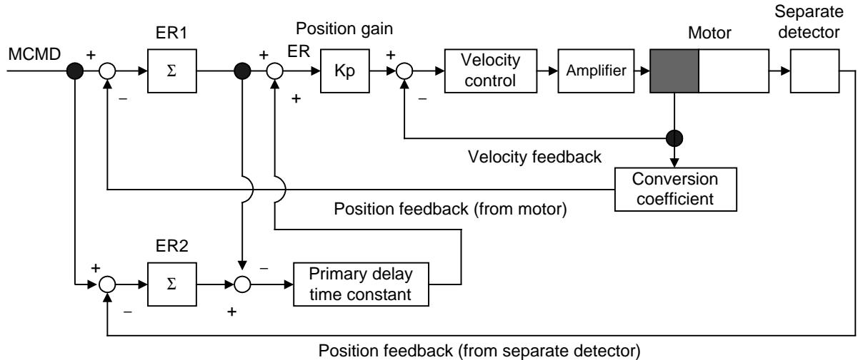
**Fig. 4.5.4 Block diagram of dual position feedback control**
