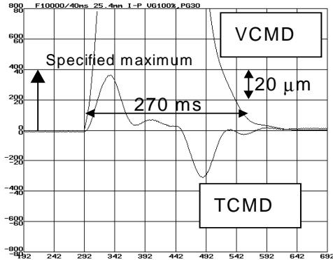
Fig. 3.4.4 (b) When I-P control is used
