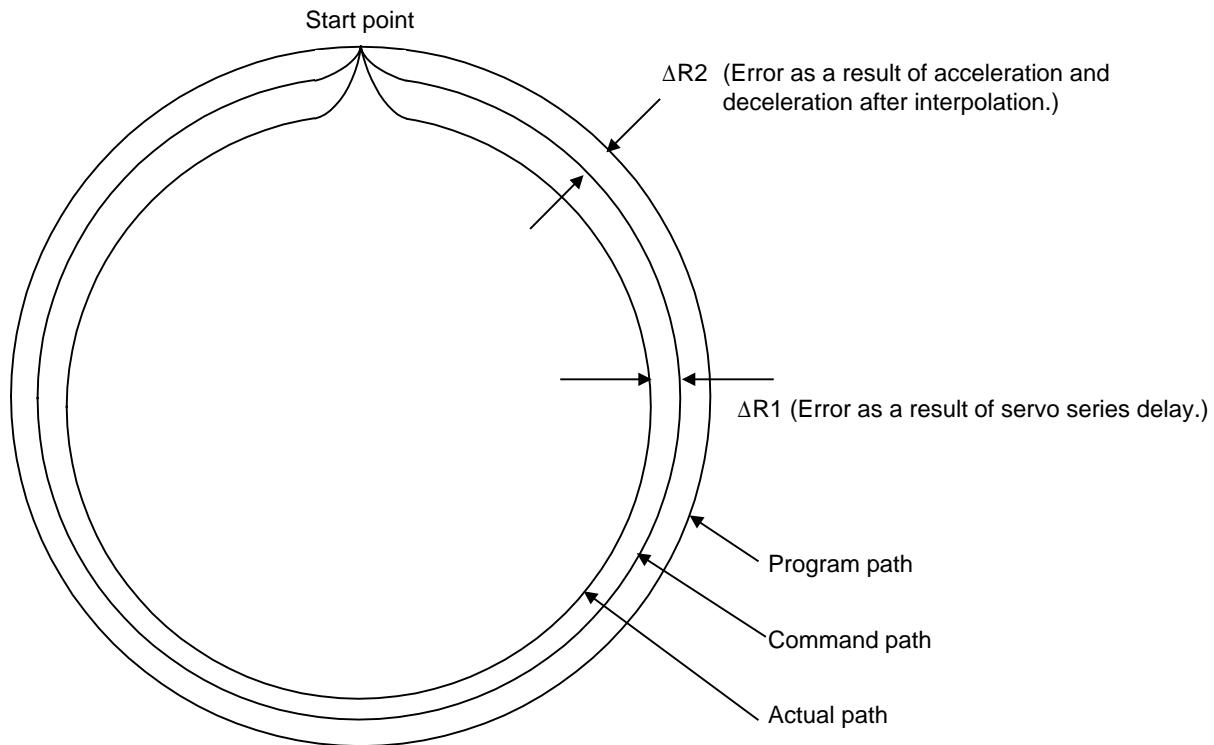
**Fig. 4.6.1 (b) Path error during circular cutting**
