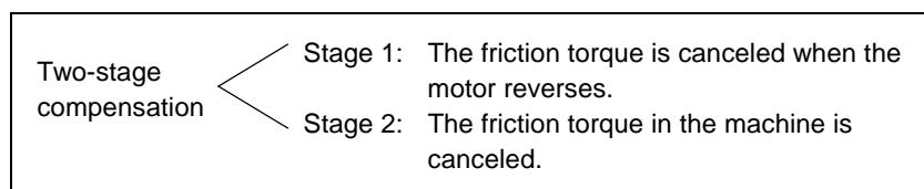
Furthermore, optimum compensation can be performed at all times for stage 1 against changing speed and load.
