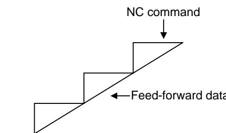
Fig. 4.6.2 (a) Conventional feed-forward control
