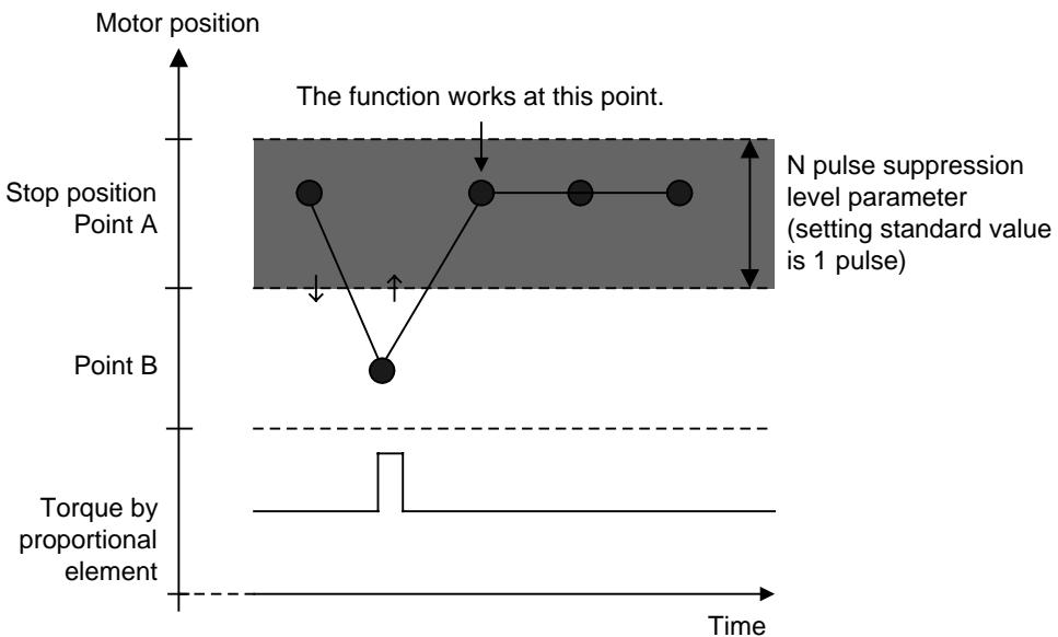
**Fig. 4.4.4 (b) N pulse suppression function disabled**
