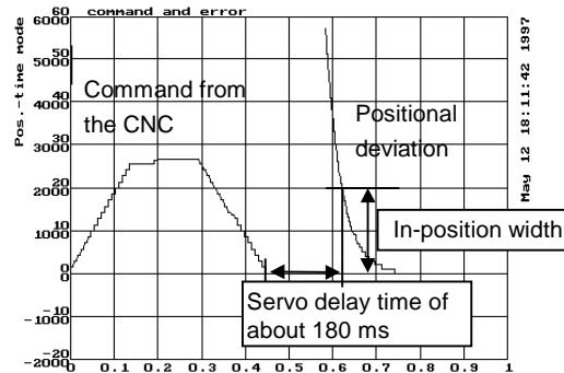
**Fig. 3.4.5 (e) Measurement of time before adjustment**
