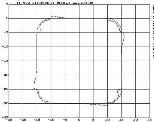
**Fig. 3.4.3 (i) Velocity feed-forward adjustment**
