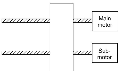
Fig. 4.17.10 (b) Example of synchronous control
