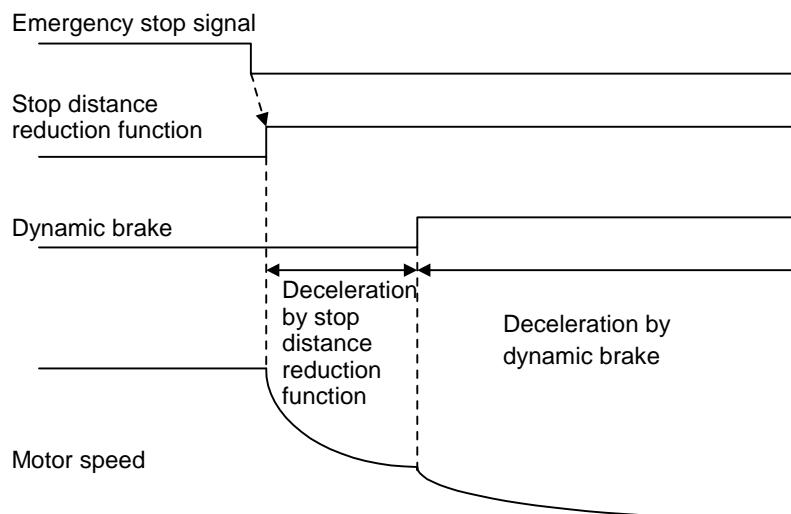
Fig. 4.11.1 (a) Timing diagram of stop distance reduction function
