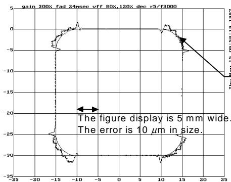
Fig. 3.4.3 (o) Arc radius based feedrate clamping
