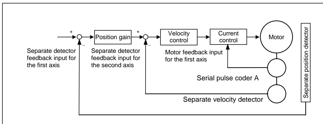
Fig. 4.16 Special system for super-precision machining
