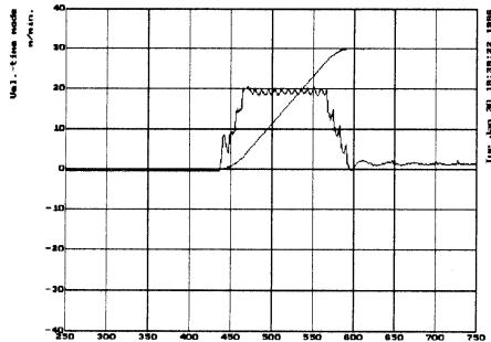
**When the feed-forward and rapid traverse bell-shaped acceleration/deceleration (acceleration/deceleration by the CNC) functions are used**
