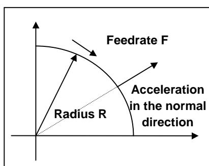
In the figure at left, let  $R$  be the radius of the arc, and  $F$  be the feedrate. Then, the acceleration in the normal direction is  $F^2/R$ . The arc radius based feedrate clamp function specifies  $R$  and  $F$  as its parameters to ensure that the acceleration in the normal direction at a specified arc does not exceed the specified value.
