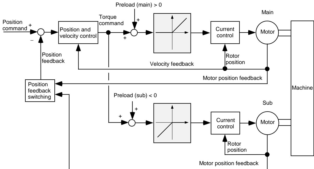
Fig. 4.17.7 (c) Servo block diagram (full preload function)
