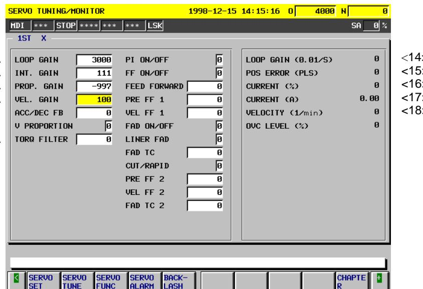
Fig. 3.1 (c) Series 15i servo adjustment screen
