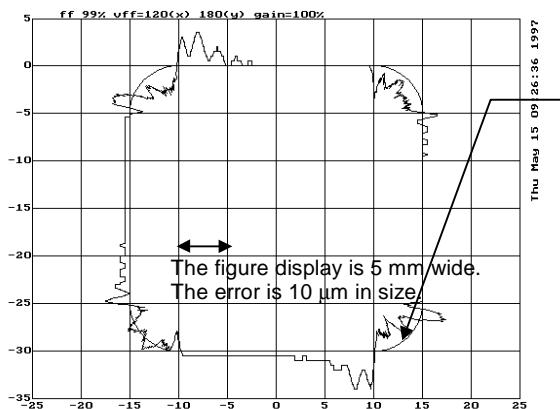
Machine vibration caused by insufficient velocity control response is observed.
