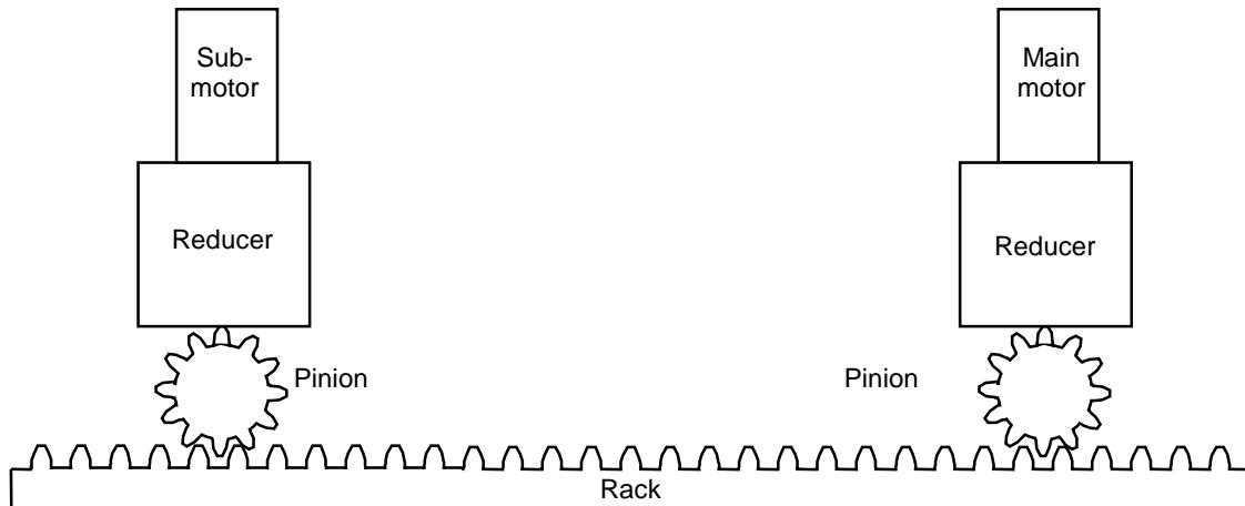
Fig. 4.17 (a) Example of tandem control application (1)
