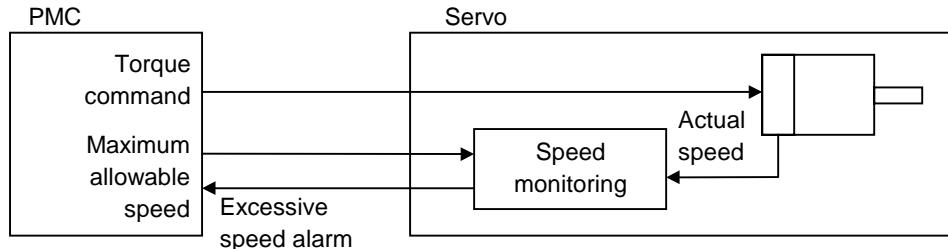
**Fig. 4.15 (a) Torque control type 1**
