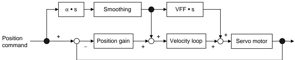
Fig. 4.6.1 (a) Feed-forward control block diagram
