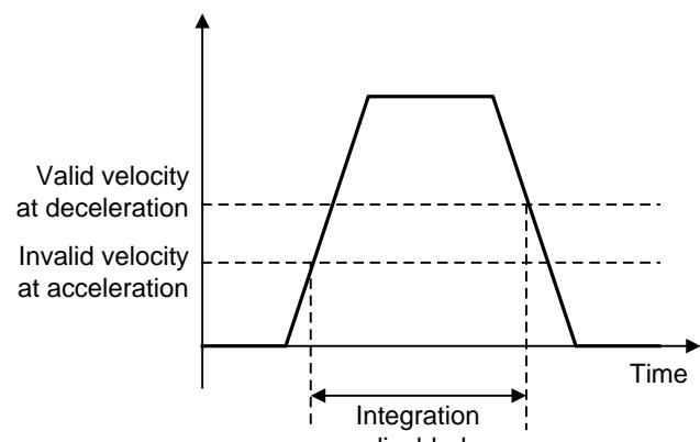
Fig. 4.8.1 (b) Integration invalid range at low-speed integration
