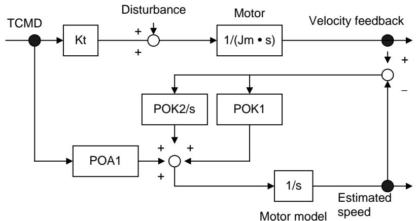
Fig. 4.5.2 (b) Block diagram of the observer
