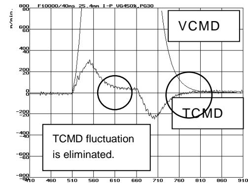
Fig. 3.4.4 (c) After velocity loop gain adjustment
