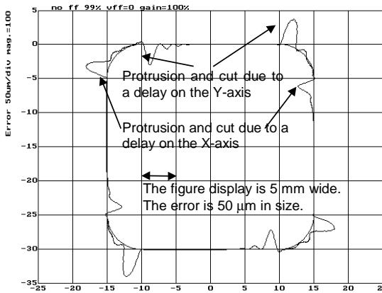
**Fig. 3.4.3 (g) Velocity feed-forward adjustment**
