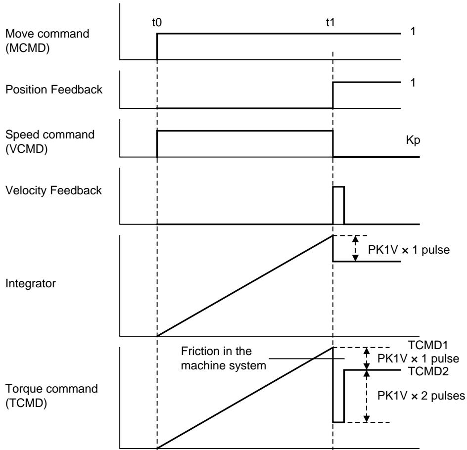
Fig. 4.7 (c) Response to 1 pulse movement commands
