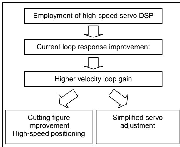
With higher velocity loop and position loop gains, the response and rigidity of a servo system can be improved. This capability enables cutting figure error reduction and higher-speed positioning with machine tools. Moreover, this capability simplifies servo adjustment. Thus, level-up HRV control can improve overall servo performance.
