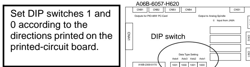
Example of setting with the DIP switches on your side as shown at the right.
