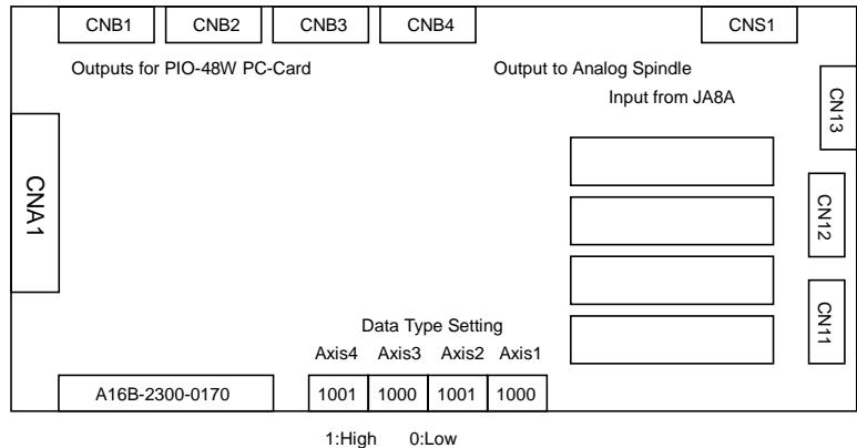
**Fig. 4.19 (b) Connector layout on servo check board B
