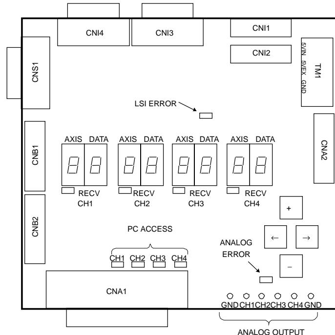
**Fig. 4.19 (a) Connector layout on servo check board A
