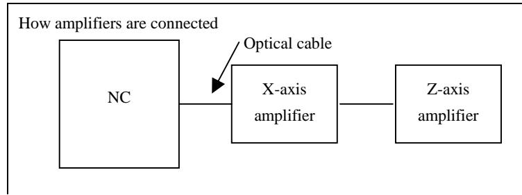
Let us consider how to make the Y-axis (second axis) a dummy axis in the above configuration.
