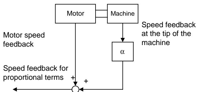
The current machine speed feedback configuration is as shown left figure. Assuming that the motor speed feedback is much the same as the speed feedback at the tip of the machine, the speed feedback for the proportional term is  $(1 + \alpha)$  times the motor speed feedback. This causes a conflict to the weight of the VCMD.
