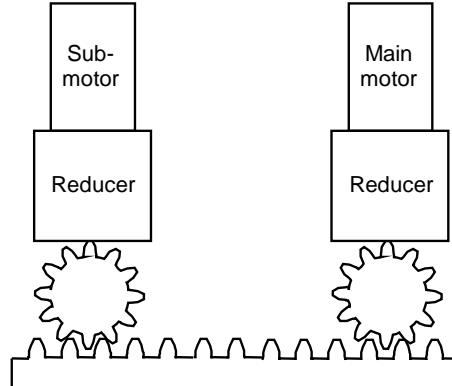
Fig. 4.17.10 (c) Example of tandem control
