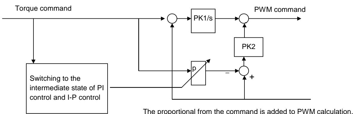
Fig. 4.5.7 Block diagram of current loop 1/2PI control
