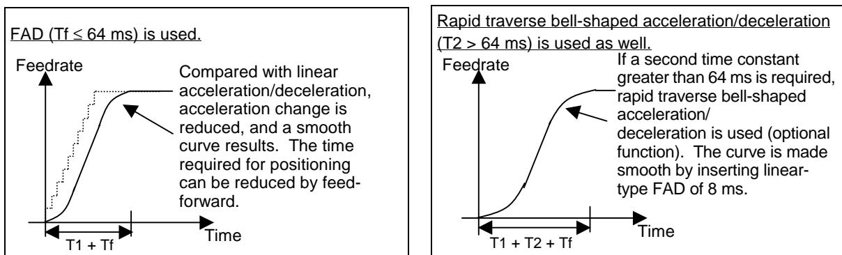
Fine acceleration/deceleration increases the time required for command distribution by a time constant. However, a time reduction in positioning achieved by feed-forward is greater than this increase, so the time required for positioning can be reduced in total. Thus, positioning can be speeded up using fine acceleration/deceleration. The adjustment procedure is described in (3) below.
