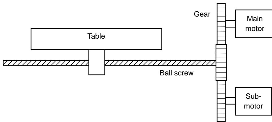
**Fig. 4.17 (b) Example of tandem control application (2)**
