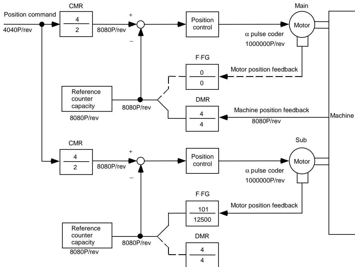
Fig. 4.17.9 (a) Example of position feedback setting
