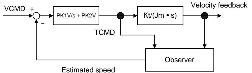
Fig. 4.5.2 (a) Configuration of velocity loop including observer
