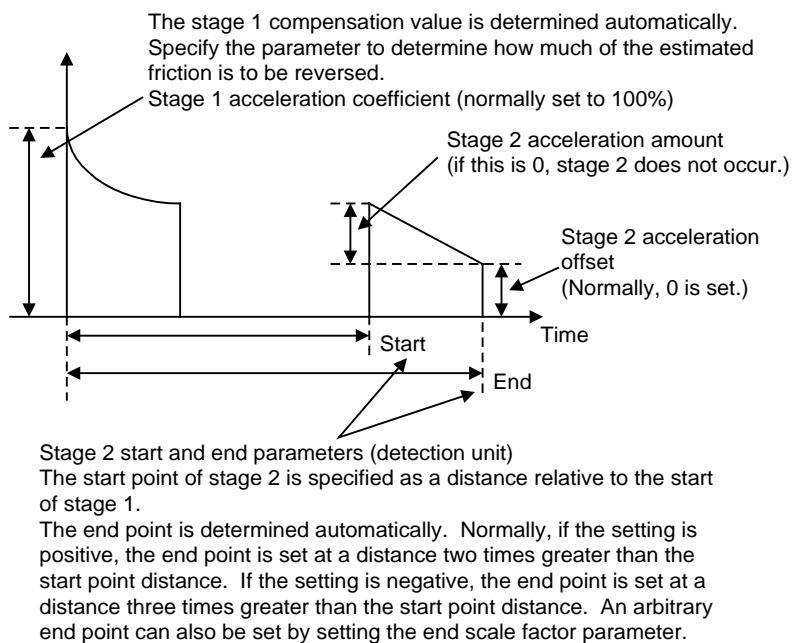
**Fig. 4.6.5 (a) Backlash acceleration under control of the two-stage backlash acceleration function**
