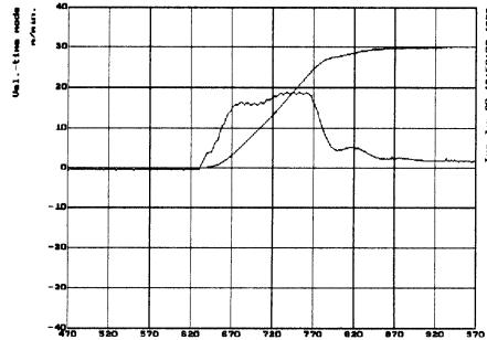
**Conventional control in which the feed-forward function is not used**
