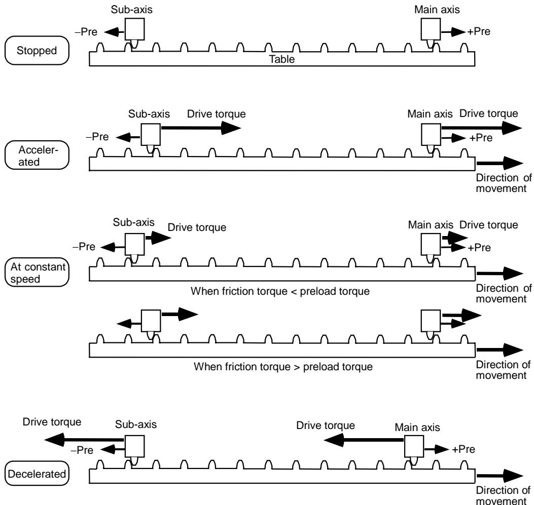
Fig. 4.17.1 (a) Changes of torque during movement
