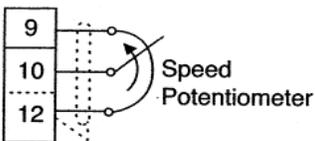
**With Uni-polar Speed Potentiometer ( DO NOT Connect Shield to Earth Ground ! )**
