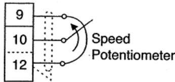
The Start/Stop Switch And the Speed Potentiometer are supplied as shown on the drive cover
