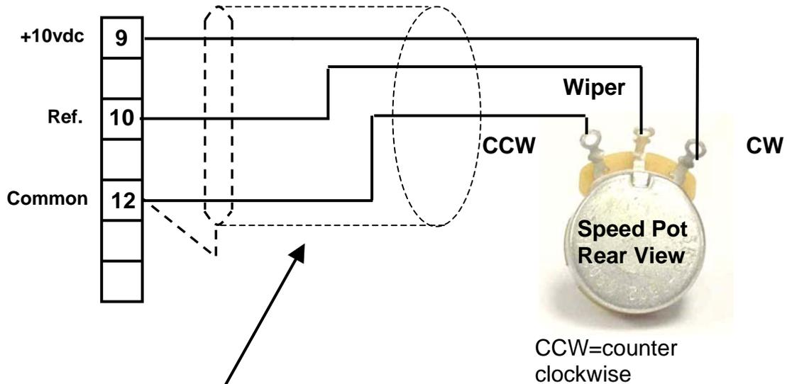
Cable should be 3 conductor with overall shield w/pot end tied off and dressed. Cable and pots are available from:
