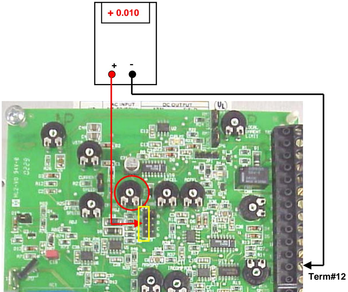
With power applied to the drive but NOT in run. Measure the dc voltage at JP9 (any of the free pins on the left side) with respect to signal common (terminal #12).
