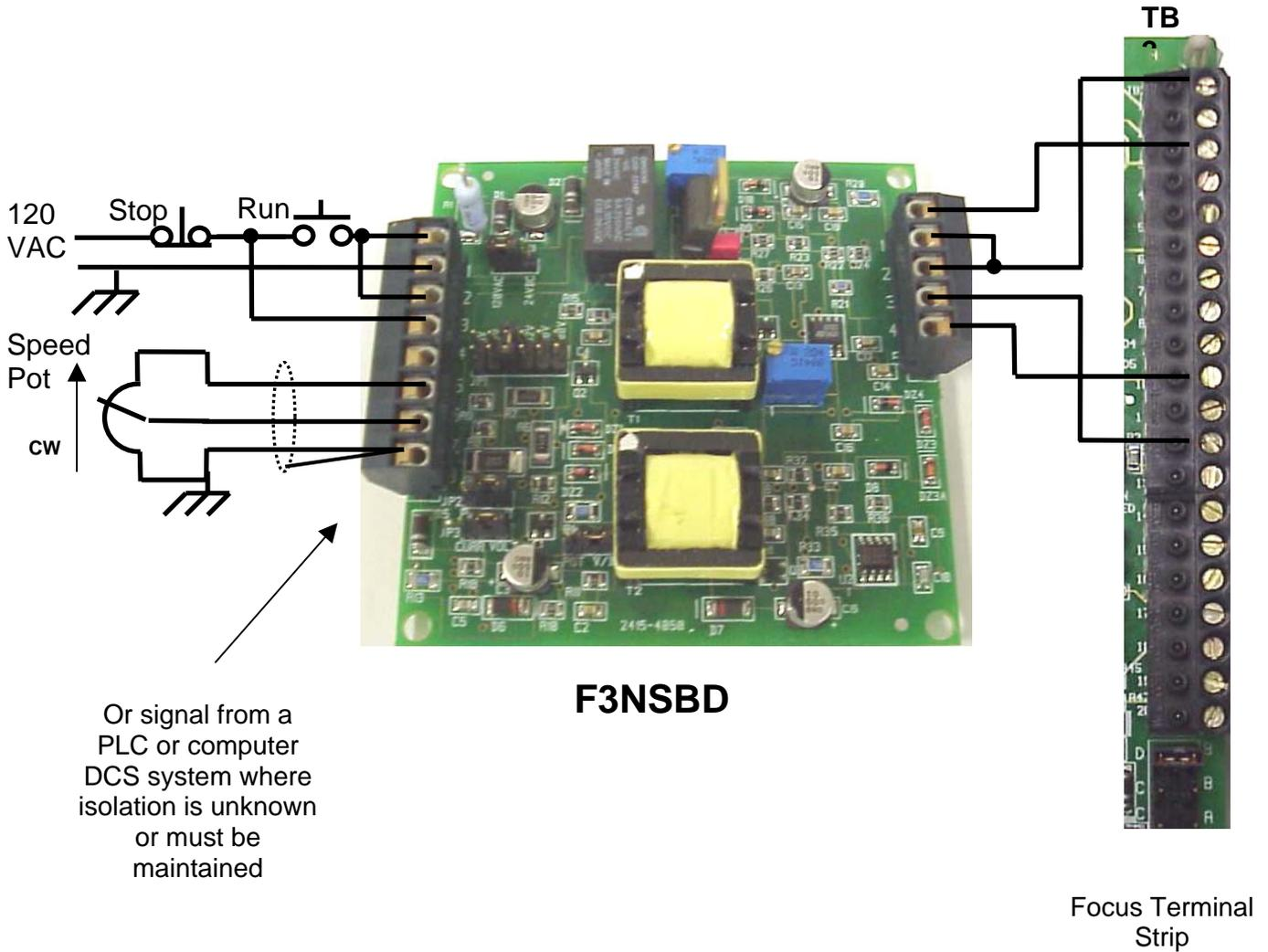
Or signal from a PLC or computer DCS system where isolation is unknown or must be maintained
