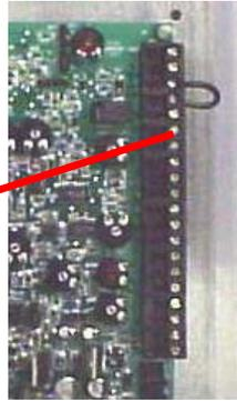
The Chassis Model has no operator devices connected to the drive control terminal strip. The only connections made are connections from terminal #3 to #4 which is required for three wire Start/Stop controls.
