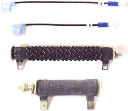
For use with Focus 3 Contactor Kits. Dynamic braking provides rapid motor stopping by quickly dissipating the stored energy in the rotating motor and load. These resistors have been sized in accordance with Nema specifications for dynamic braking.
