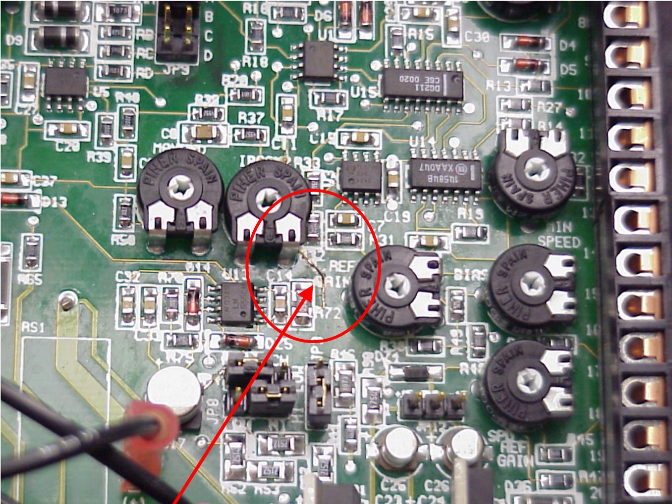
**Typical Damaged circuit trace due To earth ground connection on Control terminal strip**
