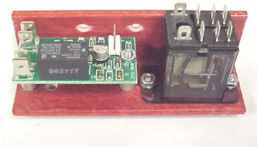
This Kit includes a magnetic contactor that can be mounted either in the Focus 3 enclosed unit or on the chassis mount unit. It provides a positive disconnect of the motor armature when the controller is stopped, preventing motor rotation in the event of SCR mis-fire due to line noise. This kit may also be required by local and/or National Electrical Codes. This kit also includes the DB (dynamic braking) poles, an auxiliary normally open contact and all connection wires.
