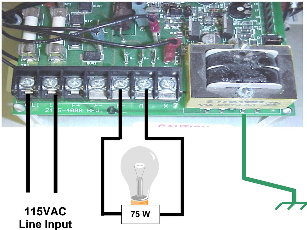
In order to test the Focus, one would need to setup the input for 115 Vac operation and for basic Armature Voltage feedback. The drive should also be set for the lowest current setting. Therefore before testing, one should record the settings before test so that they could be reset back after the test.
