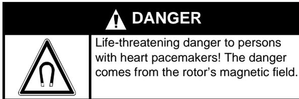
Mark the storage location clearly with warning notices as per the packaging of the built-in motors.
