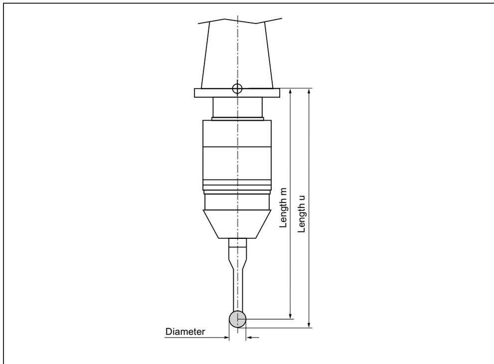
Figure 8-17 Electronic workpiece probe
