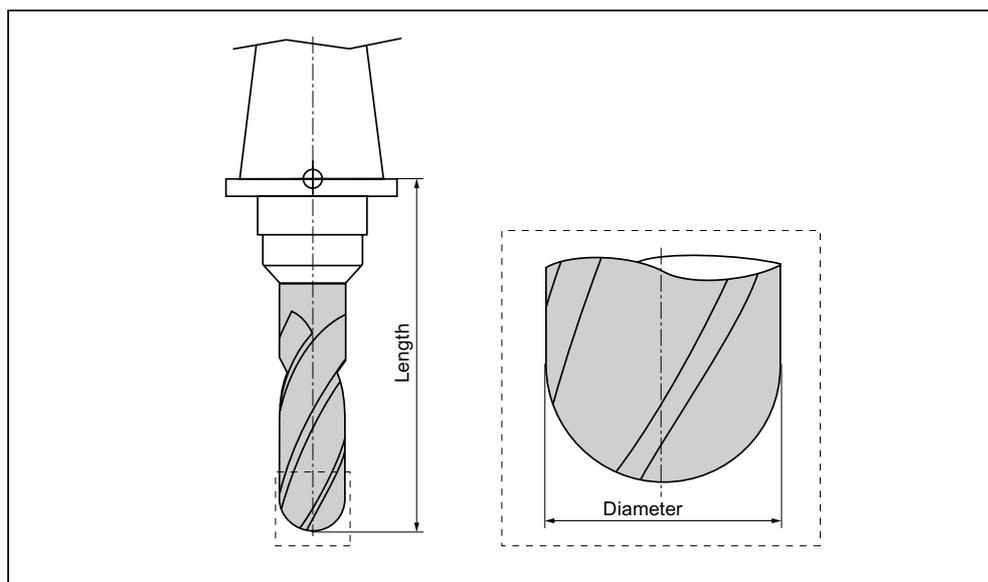
Figure 8-11 3D tool with an example of a cylindrical die-sinking cutter (Type 110)
