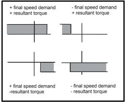
Depending on the sign of the final speed demand and the resultant torque the four areas of operation shown here are possible.
