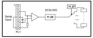
Once data has been received in this mode, a comms loss trip will occur if the comms link is lost and the last data received is non zero.
