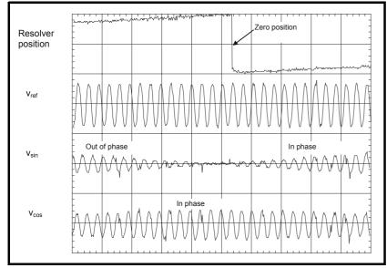
If the resolver output phase relationship is not correct an ENC.PH7 trip will occur during the resolver test for a servo machine, or during the magnetising current test for an induction machine operated in closed loop vector mode.
