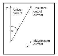
The magnitude given in Pr 4.01 is proportional to the length of the resultant output current vector.
