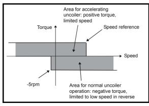
In this mode ramps are not active whilst the drive is in the run state. When the drive is taken out of the run state, but not disabled, the appropriate stopping mode is used. It is recommended that only coast or stopping without ramps is used. If ramp stop mode is used the drive changes to speed control mode to ramp to stop with a reference defined by the user speed demand. This causes the speed to increase towards the reference and then ramp to stop.
