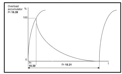
Pr **10.31** defines the time for the resistor to fall to ambient temperature but this does not mean that this amount of time is required between braking. The actual period between braking will depend on the amount of energy put into the resistor during a braking period, since the braking resistor accumulator must remain below 100% to prevent a trip (dotted line).
