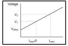
The gradient of the line gives the stator resistance, cabling resistance and resistance effects within the drive. The units are converted to ohms before being stored in Pr **5.17**.
