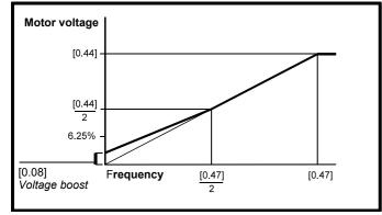
Vector control causes the voltage boost to be automatically regulated according to the load on the motor.
