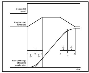
Since the ramp rate is defined in s/100Hz or s/1000rpm and the S ramp parameter is defined in s2 /100Hz or s2 /1,000rpm, the time T for the 'curved' part of the S can be determined from:
