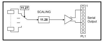
In the event of the drive tripping a value of zero is transmitted. Mode 3 input variable from another drive.
