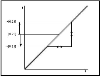
When the frequency/speed (input) reference ascends into a skip band, the resulting (output) reference remains at the lower edge of the band until the input reference has reached the upper edge of the band. The output reference then jumps to the value of the input reference.
