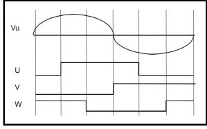
A static test can also be done to check the alignment by passing a DC current through the machine as shown below. The U commutation signal should be toggling from high to low, the V signal should be low and the W signal should be high.
