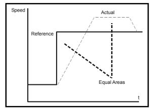
In non rigid lock mode the position loop is only closed when the 'At Speed' condition is met. This allows slippage to occur while the speed loop is not satisfied.
